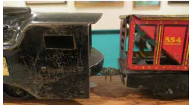
Tab and Slot coupler that the Marx train used.
