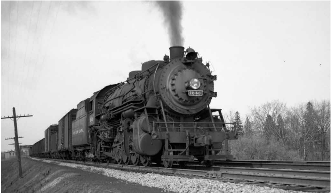
The NYC local freight above makes a round-trip daily between Corning and Dresden, N.Y., and is shown chuffing slowly uphill on its southward lap at Himrod Junction. Its power is a trim light USRA Mikado, no.1848, which is one of almost 150 such machines on the Central, with the H-6a classification. (Jeremy Taylor photo.)
