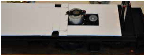
You can see the floor that will go inside the unit to support the prime mover and the added section to be installed in the front section of the loco.
