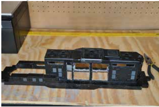
You can see that all of the panels have been removed and the door edges are smooth.
