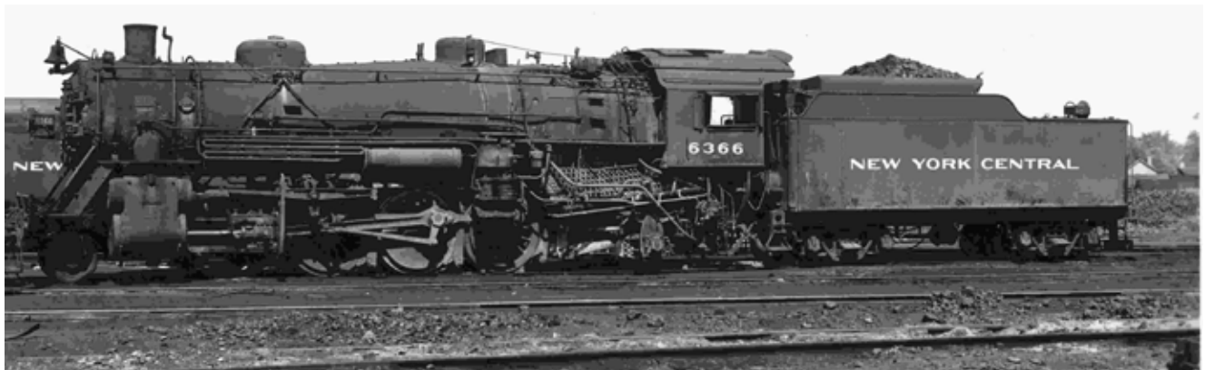
Renumbered 1951, USRA design, extended tender coal boards, Built. 1918 (Lentz Bros. Studio, NYCSHS Collection.)
