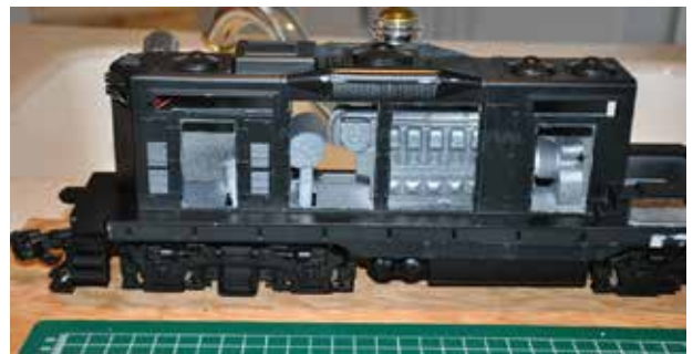
The shell is in place and the prime mover is visible through the open access panels.
