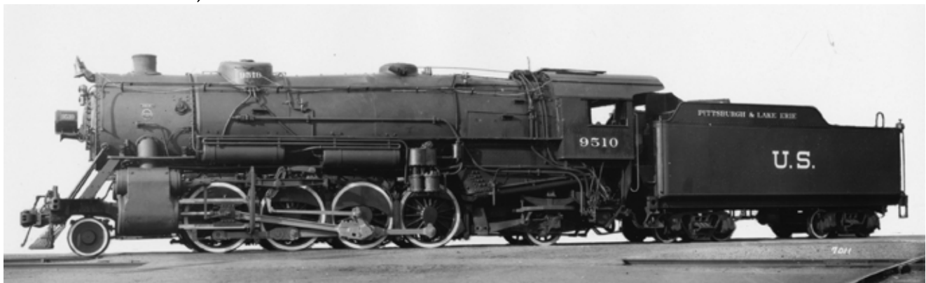
Builder photo, USRA Mikado B side. P&LE # 7011.(Contributed by Jeffrey Moreau., NYCSHS Collection)
