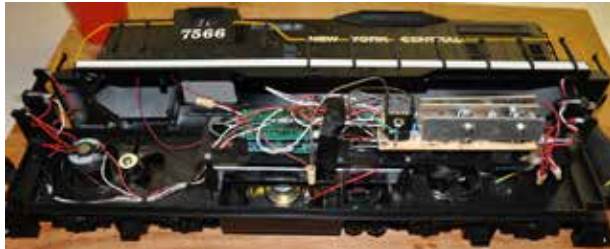
The GP-9 with the "guts" being removed.
