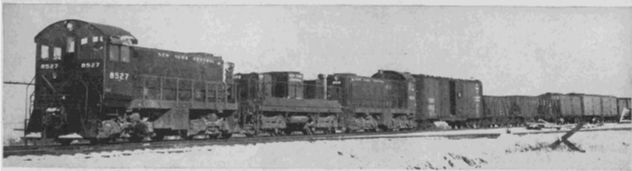
At two miles per hour, a new diesel-electric hump locomotive pushes a train of loaded freight cars over the hump of the eastbound Classification Yard at DeWitt, N.Y. Two switchers, separated by a trailer, are operated as a single unit by means of pneumatically connected controls. This
