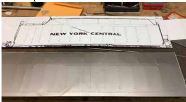
The drawing used for the decals Steve applied to the metal tender sides he had fabricated and then drilled and tapped the rivets in place.
