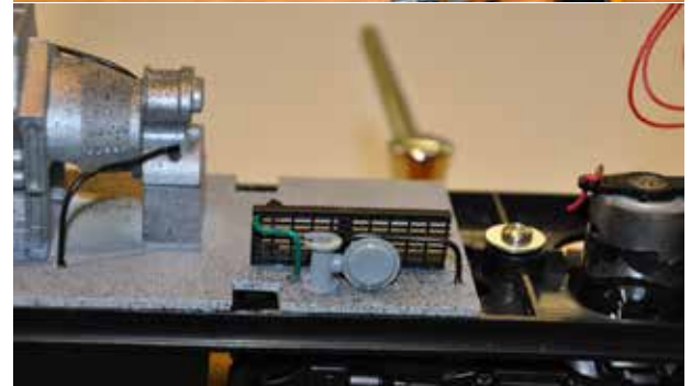
The prime mover and all of the auxiliary equipment are installed on the floor of the frame.
