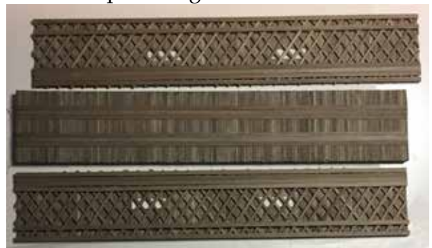
Both side walls and floor assemblies are completed and stained and ready for final assembly as the bridge.
