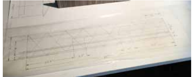
Simple drawing used to create model, only one side elevation and one end elevation.
