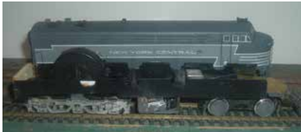
The motor and running gear on the track in front of the modified shell.
