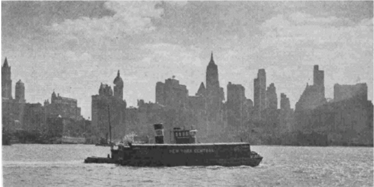
Eighty thousand freight cars are handled in six months by the NYC's Marine Department. NYC's diesel Tug 33 rounding lower Manhattan from the Hudson River into the East river with a covered barge
