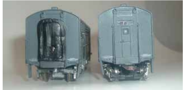
You can see the finished product after Robert installed the rubber diaphragm on the rear door of the second A-unit.
