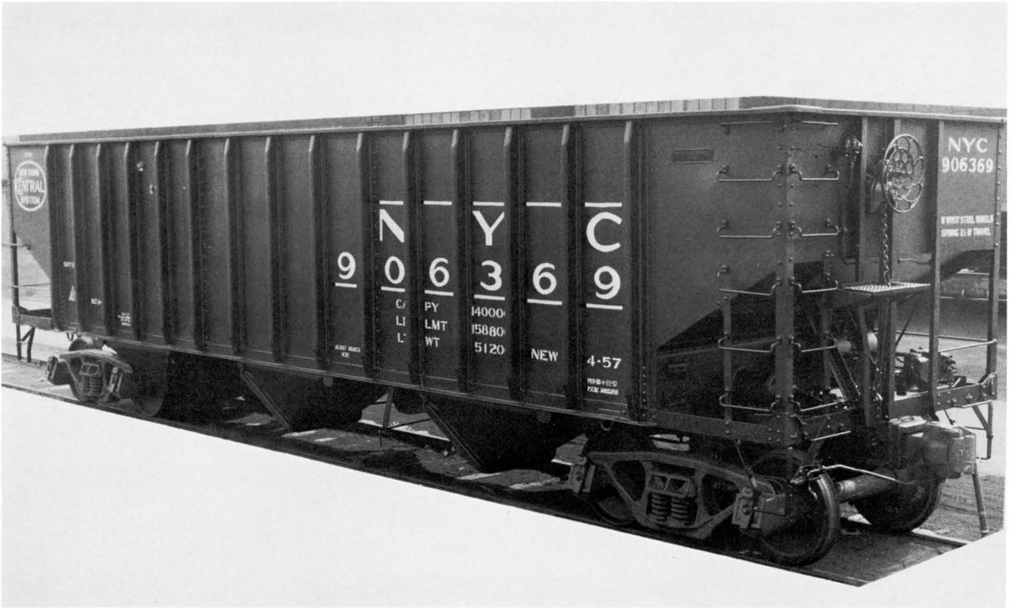
Car 906369, Lot 869-H, was built by Pullman-Standard at Butler, Pa. in April 1957 to Specification 959-B. This car is equipped with Barber trucks.
