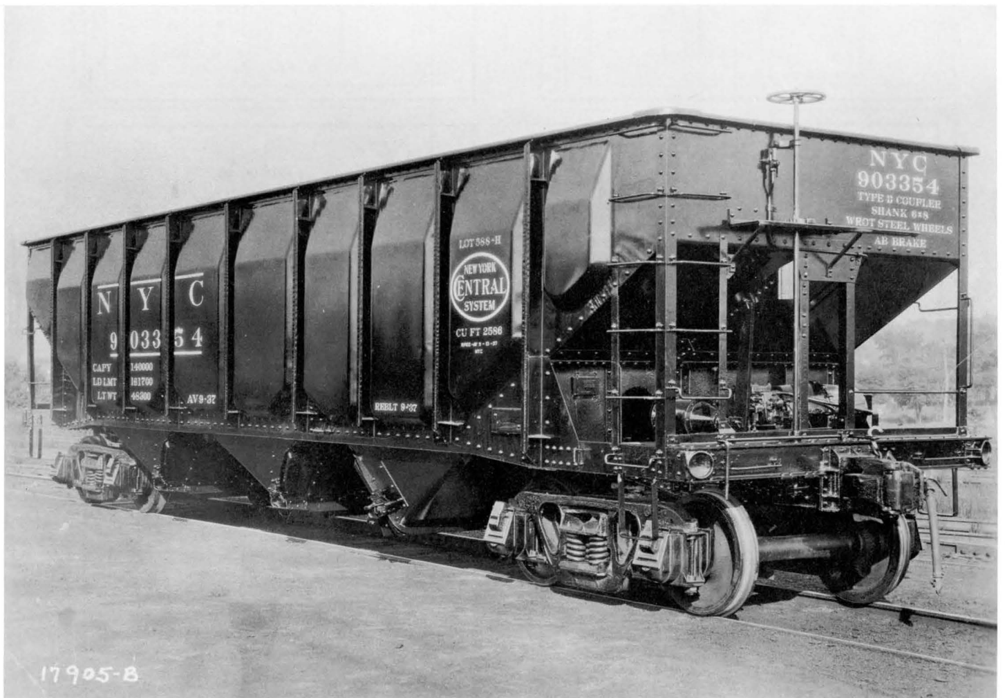
Car 903354, Lot 588-H, exemplifies this lot as rebuilt with panel sides at Avis, Pa. in 1937. All cars except 903171 (ex-435171) received this treatment. Note also that AB brake equipment was applied. Trucks are still the Andrews type.
