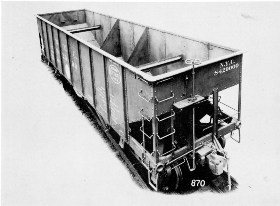
The 13,800 cars built to Specification 480 were exemplified by these photographs of NYC S-429000, built by the Standard Steel Car Co. in 1924. This car was one of 1,600 to this specification built with truck design to NYC drawing N-38314, which was sprung at the journal box and was furnished by the car builder. These trucks were phased out after 1938.
