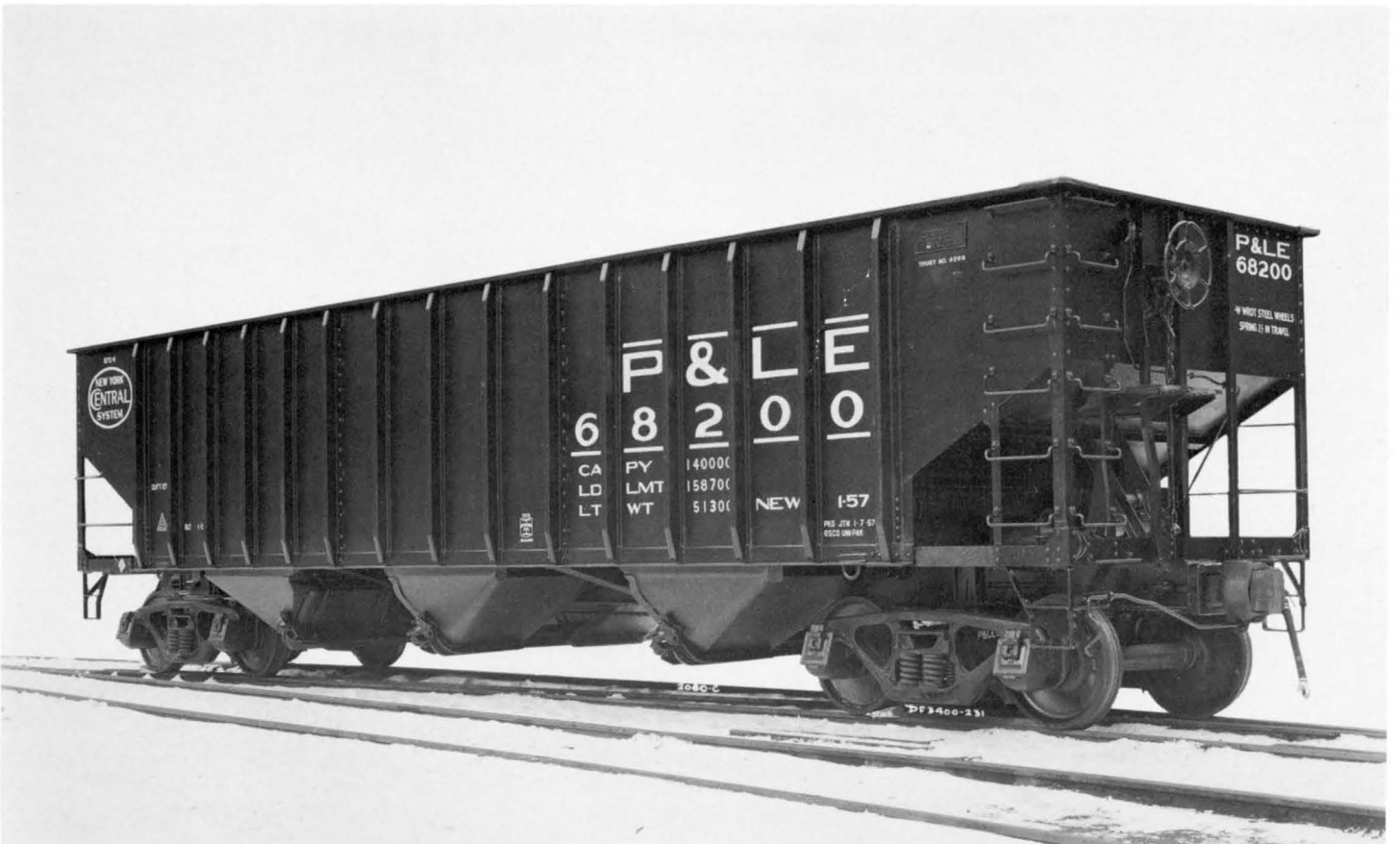
Car PLE 68200, Lot 870-H, was to Specification 959-B and was built by Bethlehem Steel Corp. at Johnstown, Pa. in 1957. Trucks are Barber type, and hopper doors have Wine latches. Hand brake is by Miner.
