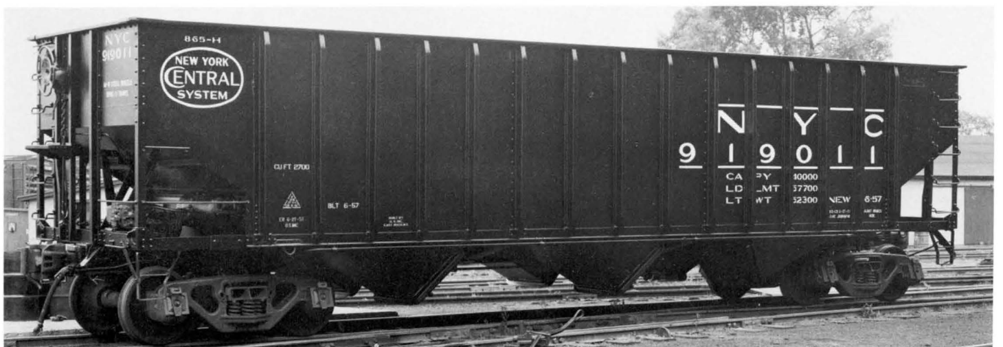
Car 919011, Lot 865-H, was the twelfth 70-ton hopper car to Specification 959-B completed at East Rochester in 1957. This car has National C-1 trucks, Enterprise door hardware and Miner hand brake.
