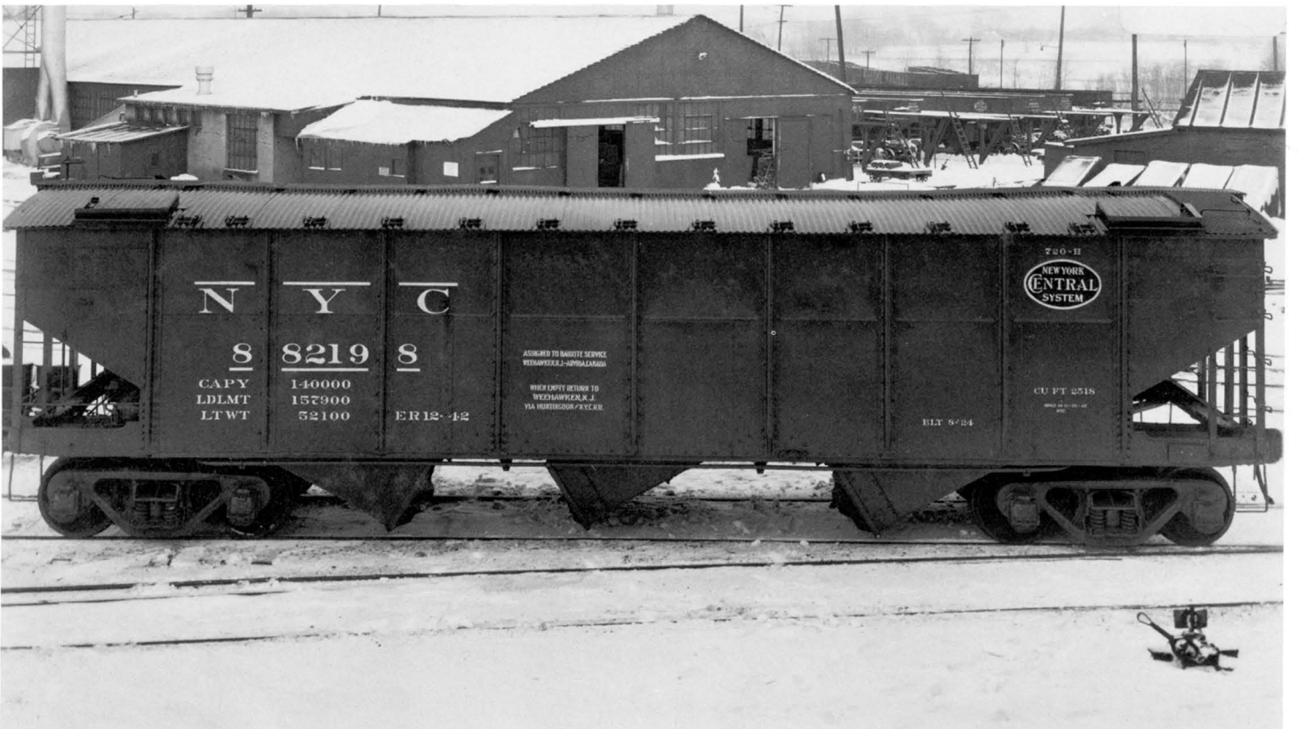
In 1942 240 cars from Lots 466-H, 467-H, 488-H, 496-H and 499-H (Specification 480) had removable sectional roofs applied and were assigned to bauxite service as Lot 720-H, cars 882000-882239. Car 882198 is shown as outshopped at East Rochester.
