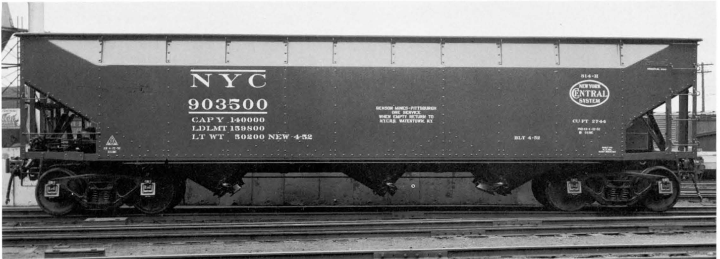
Car 903500, Lot 814-H, exemplifies the inside-stake hopper cars of the AAR 70-ton design, NYC Specification 954-B, as built at East Rochester in 1952. Note that the car is stencilled for Benson Mines-Pittsburgh ore service. Sintered ore was loaded hot, hence in-service cars were rarely seen with paint intact. This car has Barber stabilized trucks.
