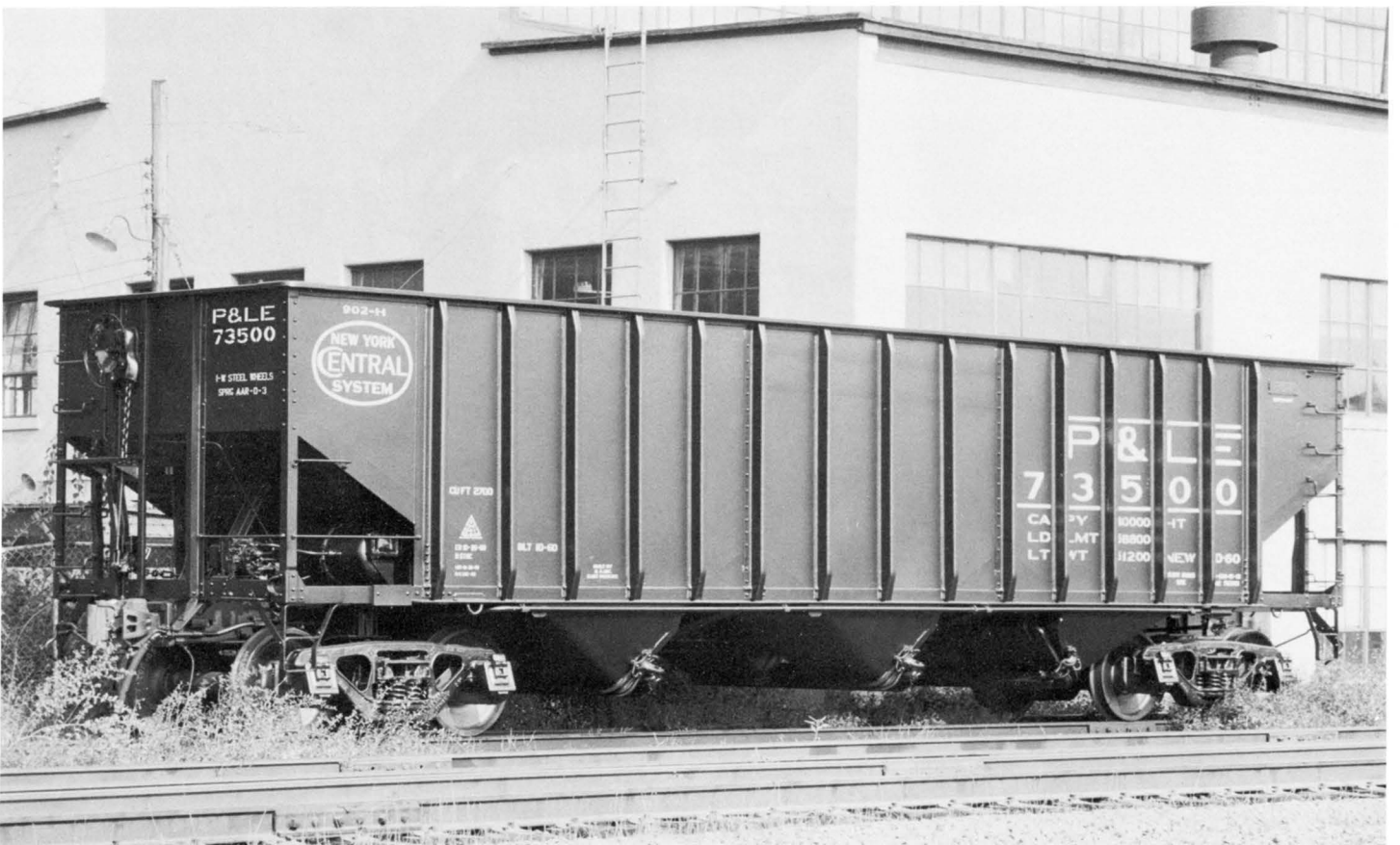
Car NYC 950000, Lot 904-H, was to Specification 959-E, and represents the last 350 70-ton hopper cars built for the NYC. This car has Enterprise longitudinal hopper doors for ballast service. Trucks are of the Barber design.
