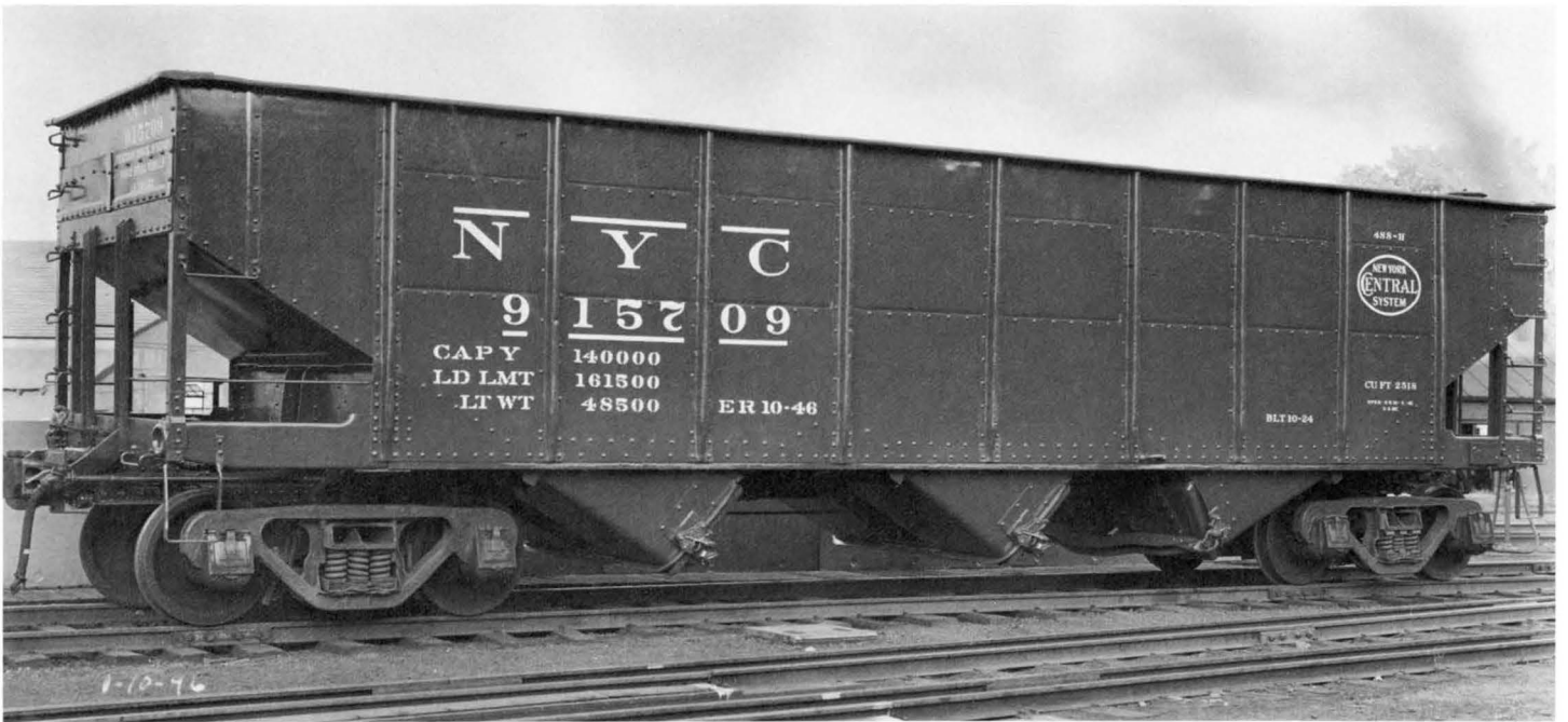
Car 915709, ex 431709, was from Lot 488-H and is shown as repaired at East Rochester in 1946. This car has USRA 70-ton trucks with Keystone separable journal box side frames.
