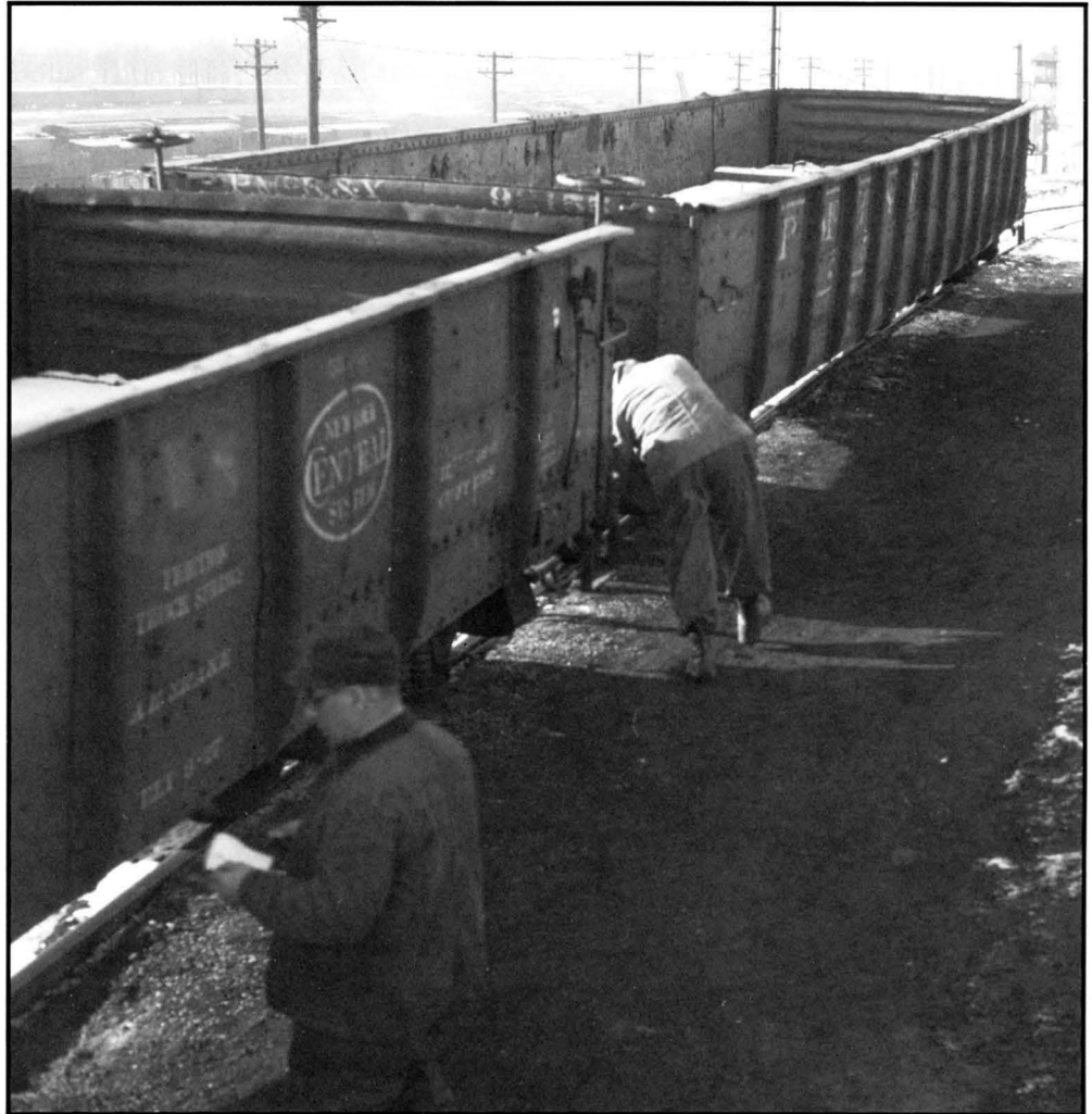
Hump conductor pulling the pin, Selkirk, N.Y. Photo by J. Taylor.
