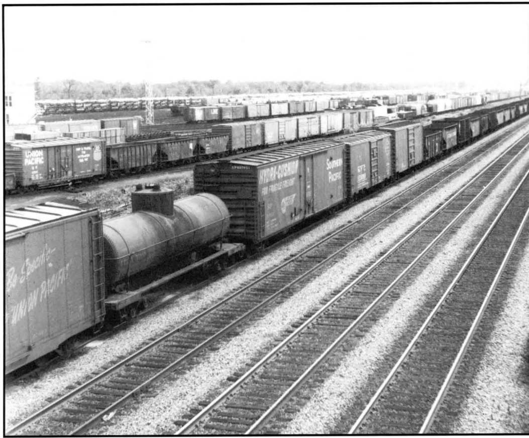
An about-face and slight shift to the south from the previous location provides this view of the main line extending east alongside the yard. Beyond the two mains are the controlled siding, "4 outside" (here occupied by a westbound relay train), the westbound receiving yard (the cut just above the car-tops of the relay train is advancing toward the westbound hump), and the Eastbound Class and North Yard portions of the eastbound classification complex. (The light tower stands between tracks 34 and 36 in the Eastbound Class; the multilevels are in the North Yard.) Controlled point SE, consisting of universal cross-overs between main tracks and between no. 1 main and the controlled siding, is in the right background beyond the signal bridge. Photo by J. Taylor.
