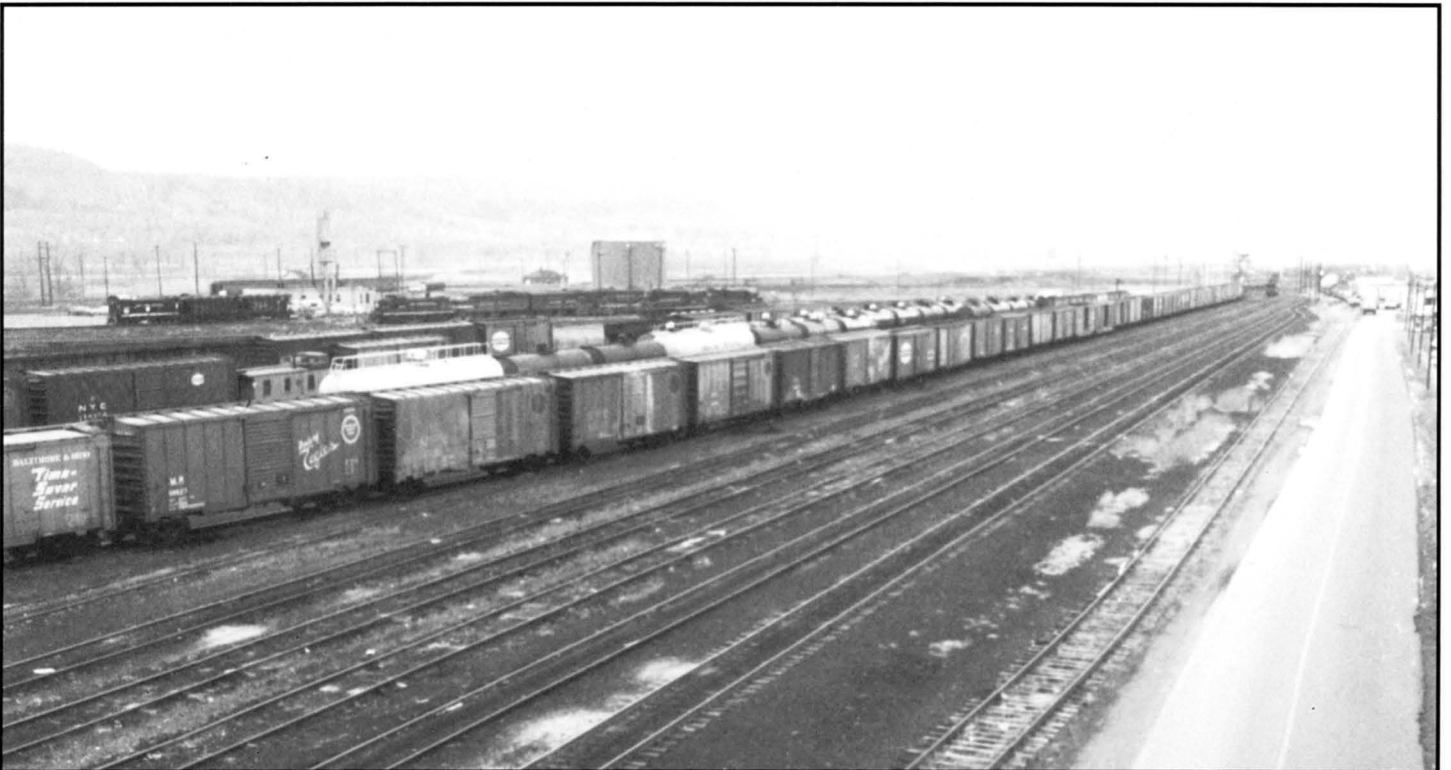
The boxcars were part of a cut being advanced from the class yard to the departure yard in this scene looking west from Jericho Road bridge. Approaching the camera, the long tracks in the class yard were numbered 24, 26, 28, 30, and 32. The track in the foreground stubbed just out of the picture, and ran down into the Flexivan pad in the right background. The multilevel unloading site was (and is) across the paved road, and the fueling station was in the left background. Photo by J. Taylor.
