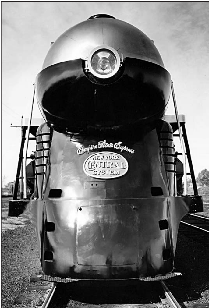
By October 10, 1941, when this photograph was taken at West Albany, the streamlining of the 5429 was complete, and the locomotive posed for a series of company photographs. This front-end view clearly shows the wider jacketing around the lower half of the smokebox. The distinctive NYC oval featured a red background; this was the first instance of a red oval being applied to the front of a New York Central locomotive, a feature that would become a tradition on New York Central diesels. NYC Negative 5978-2, NYCSHS Collection.
