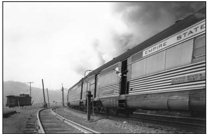
Gotcha! The mail hook on John A. Dix snags a mailbag at Hudson, New York as No. 51, the westbound Empire State Express , cants around a curve at Hudson, New York on April 30, 1946. Obviously, steam was immediately ahead. NYC Negative 7276, NYCSHS Collection.
