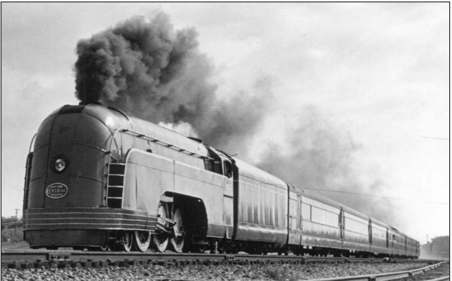
Headed by Dreyfuss-streamlined K-5b Pacific 4917, The Mercury was photographed in 1936 or 1937 near Cleveland by Melvin Stahley, a Cleveland policeman who enjoyed photography. Clearly he was good at what he enjoyed. It is unclear if the train is eastbound or westbound, perhaps one of our readers can enlighten us. Collection of Jim Semon.
