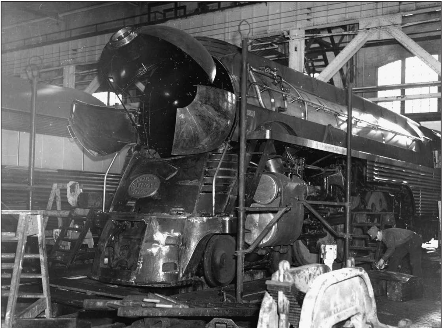
It's early in October of 1941, and J-3a Hudson 5429 is being prepared for Empire service in the company shops at West Albany, New York. The manner by which the locomotive's smokebox door could be accessed is evident. It appears that the engine's tender is on the adjacent track. NYC Negative 5978-17, NYCSHS Collection.
