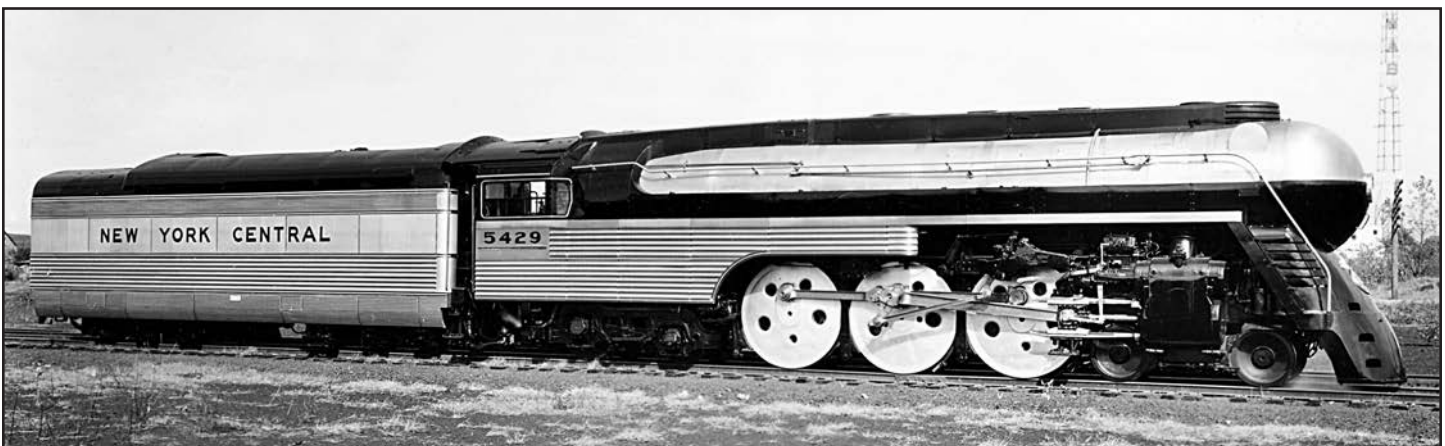
Disc drivers, covered boiler feed pipes and check valves, bullet nose, and straight-through horizontal sheathing rearward of the back drivers, gave the two Empire locomotives a distinctive appearance. The 5429 would travel west to haul the first eastward trip of the new streamlined train. NYC Negative 5978-3, NYCSHS Collection.
