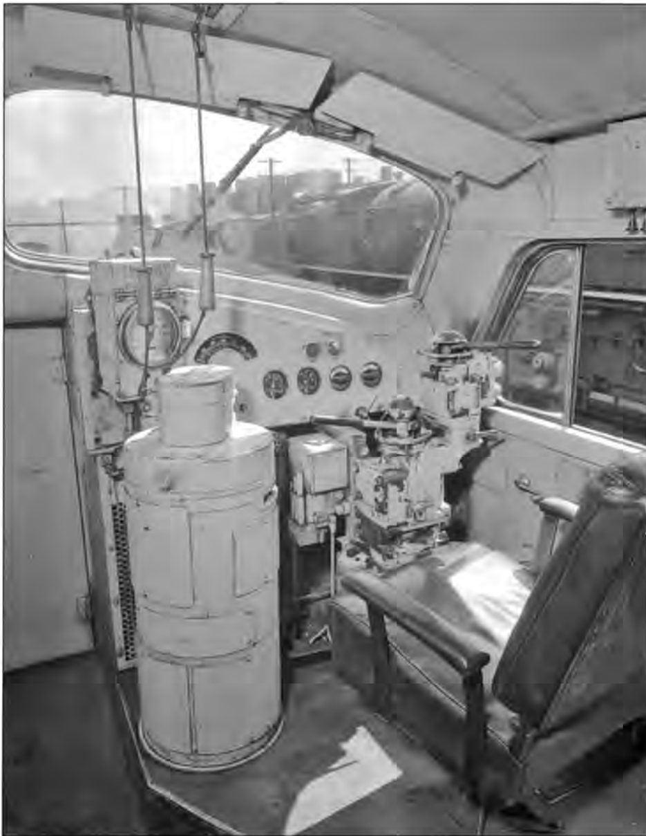
A view of the controls of E7 4002, including 8-ET brake equipment and 120 mph speedometer. Note the white running board stripe on the fireman's side of S-1b Niagara 6024, indicating that both sides of the Niagaras were striped at Alco. Niagara is almost new, delivered April 19, 1946. Negative 7433-2.
