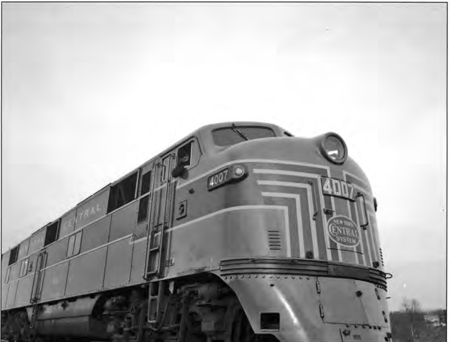
Light grey E7 4007 poses at Harmon on November 27, 1945. Nose detail includes painting, striping, and location and outline of the oval, the nose door details, as well as the front number plate composed of reflective buttons. Small number boards of the early E's were corrected with the E8 design, still several years away. Negative 7119.
