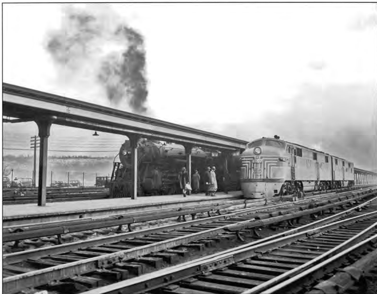
E7 4007 and a "B" unit sit at the station platform at Harmon on February 28, 1946. Elderly K-3Q Pacific 4673 is adjacent. Negative 7200.
