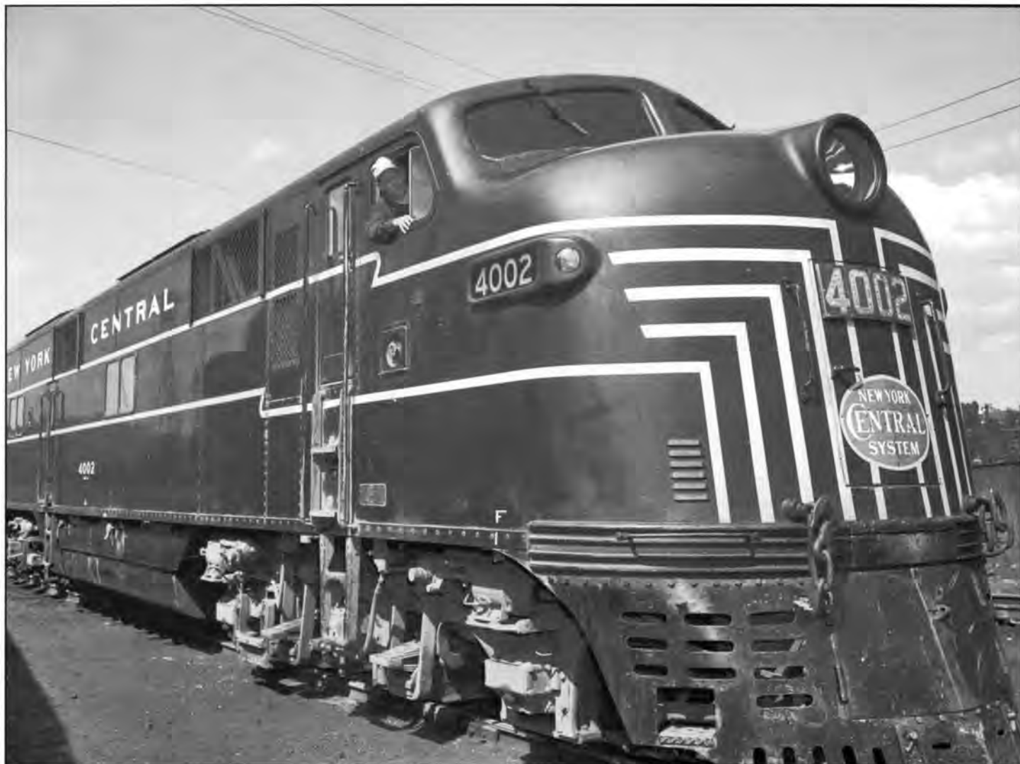
Black E7 4002 at Harmon on August 19, 1946. Notice soft corners on lightning stripe below engineer's window, a feature of this early paint scheme, and early style pilot. Holes in pilot were reportedly to provide additional air circulation to the traction motors. Negative 7476-1.
