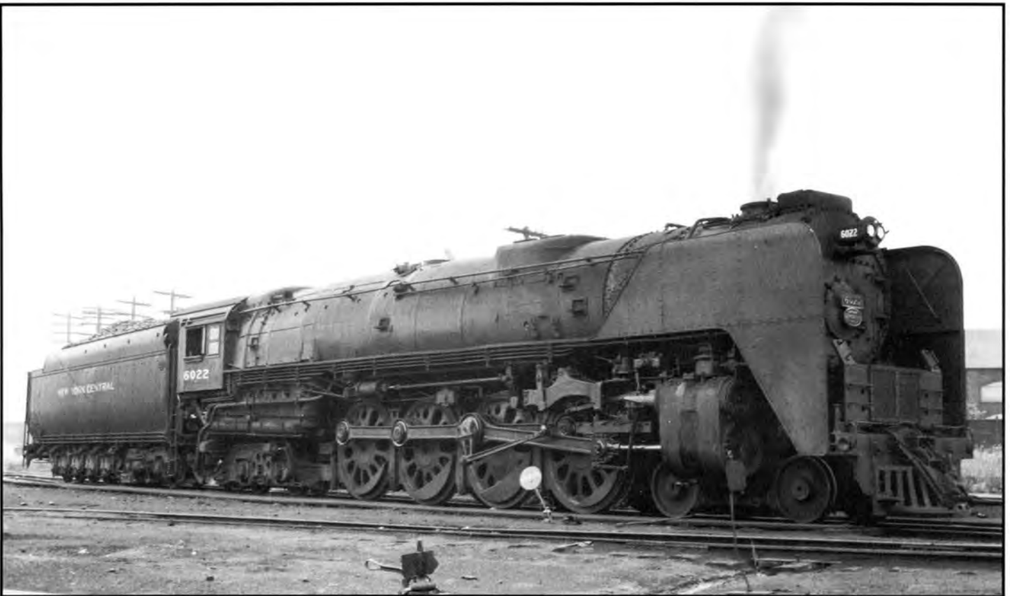
Class S1b No. 6022 at Buffalo, New York, August 9, 1953. Note bell relocated at valve gear. Photo by Joseph Brauner.
