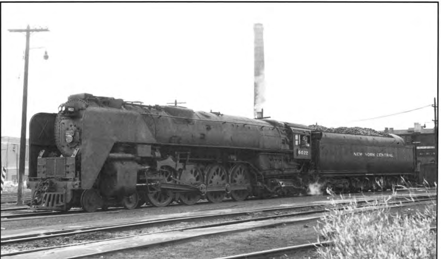
Class S1b No. 6022 at Buffalo, New York, August 9, 1953. Note headlight generator relocated between third and fourth drivers. Photo by Joseph Brauner.
