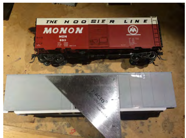
New weld lines are scribed using a modeling square; measurements were obtained from a 40-foot PS-1 kit.
