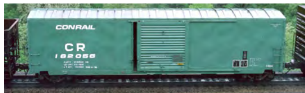
Conrail 162056 formerly NYC 215206 is at Altoona, PA in June 1976. Notice how the roof support brackets are missing from the center of the car. (Lynn Roberts photo courtesy FallenFlags.org)
