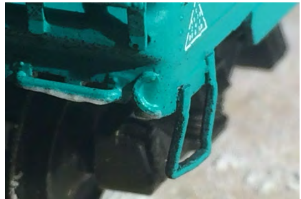
A small crescent of styrene was formed to represent the polling pocket.
