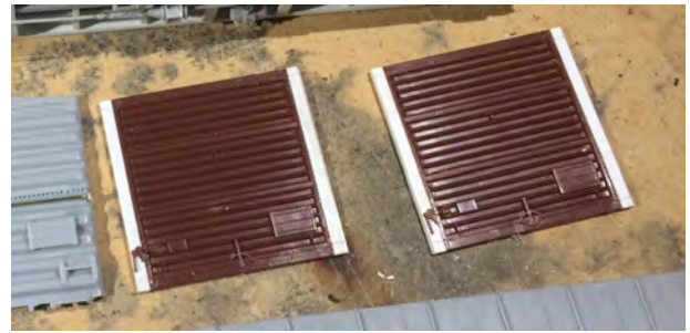
The car's doors were modified by adding styrene strips to the sides.
