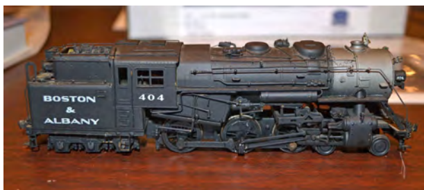
Bob Keeler's HO-scale B&A 4-6-6T-tank locomotive 404 (B&A class D1a) on the NYCSHS display tables. This locomotive class was built to power Boston area commuter trains.
