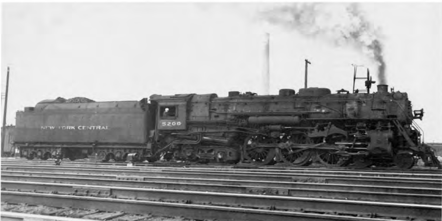
The first Hudson, J1a #5200, at Cheektowaga, N.Y. on February 3, 1952. Note that tender has had auxiliary surge tank applied, to rear of coal space. Photo by Joseph Brauner, C.M. Smith collection
