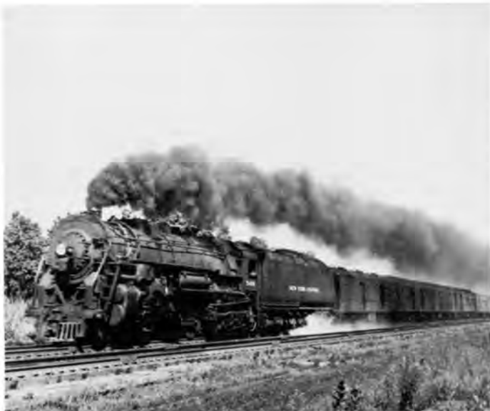
N.Y.C. Hudson 5410 takes on water Westbound at the Corvna, Indiana track pans in 1946. Note working overflow vents on the PT tank. — Bob Lorenz Collection
