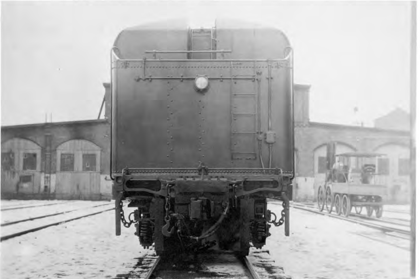
Rear view of tender, showing construction of the auxiliary surge tank back of the coal space. The "Dewitt Clinton" 1831 loco & tender on other track.
