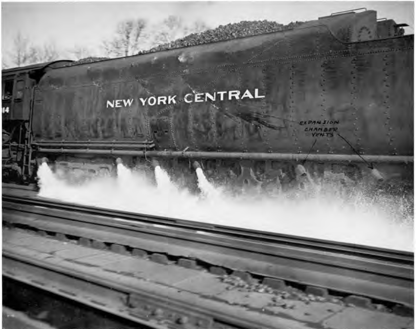
This is a close-up of a locomotive PT tender scooping water. This tender is equipped with overflow control and excess water is discharged from four of the forward end overflow-vent pipes each side, indicating that interior construction of tender permits scooped water to be carried to the extreme forward end of tender instead of cresting in the rear portion of tender. Note the paved gutters between tracks onto which the overflow water is directed so that no damage is caused by same. 6,000 gallons in 17 seconds creating the effect of jet propulsion, speed 85 M.P.H.
