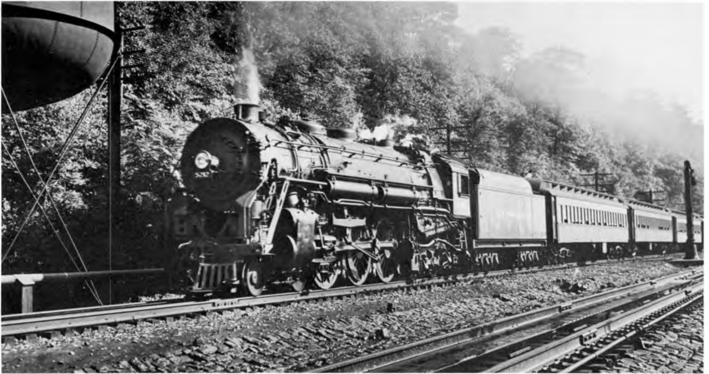
N.Y.C. J-1b 5212 at Tivoli, N.Y. approaching the track pans on August 30, 1941 with a Westbound extra train. Track pan shows up well in foreground. Edward L. May Collection
