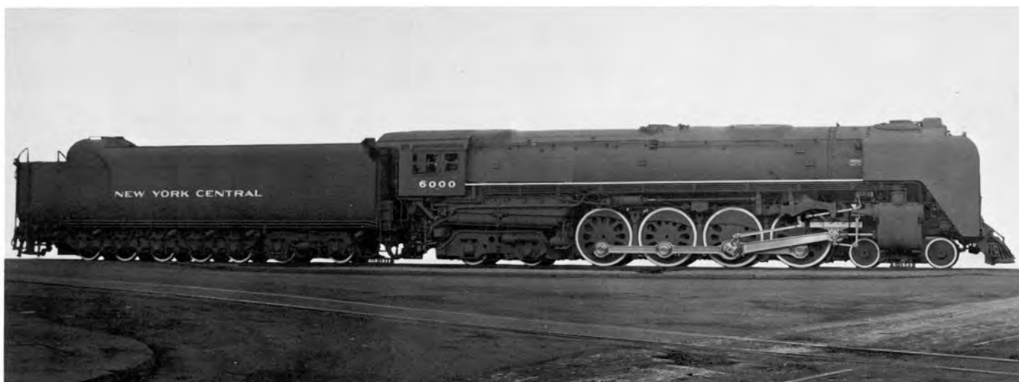
Class S1a locomotive #6000, Niagara type, with 14-wheel PT tender. Tender equipped with high speed water scoop, auxiliary surge tank and six overflow vent pipes on each side. Carl F. Kantola
