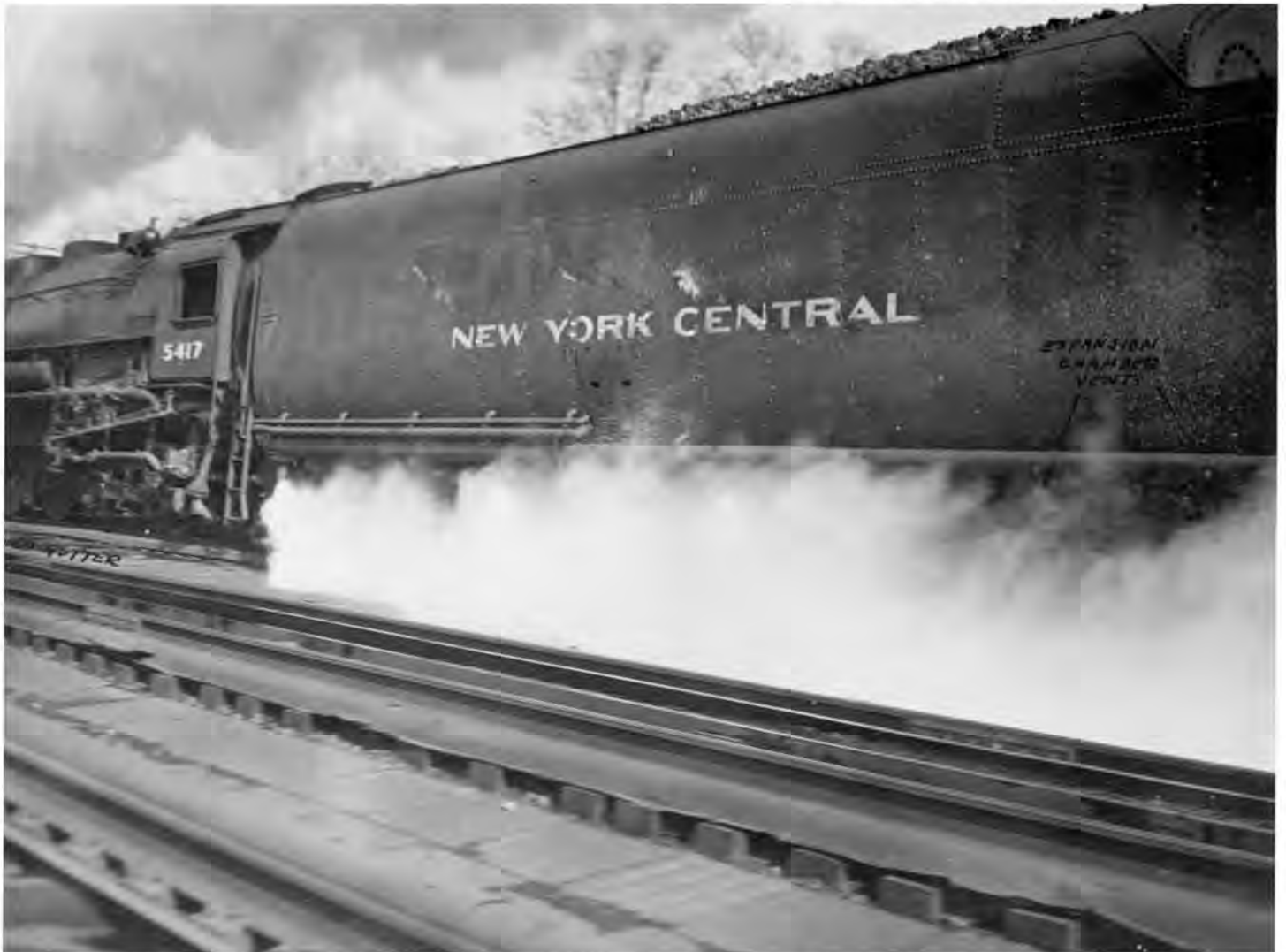
This is a close-up of a locomotive tender scooping water. This tender is equipped with overflow control and excess water is discharging from overflow vent pipes throughout the length of tender except the pipe which vents from the top portion of expansion chamber, indicating that the tender has filled with water but has not yet surged up to the highest part of the expansion chamber. Note the absence of any overflow from top.
