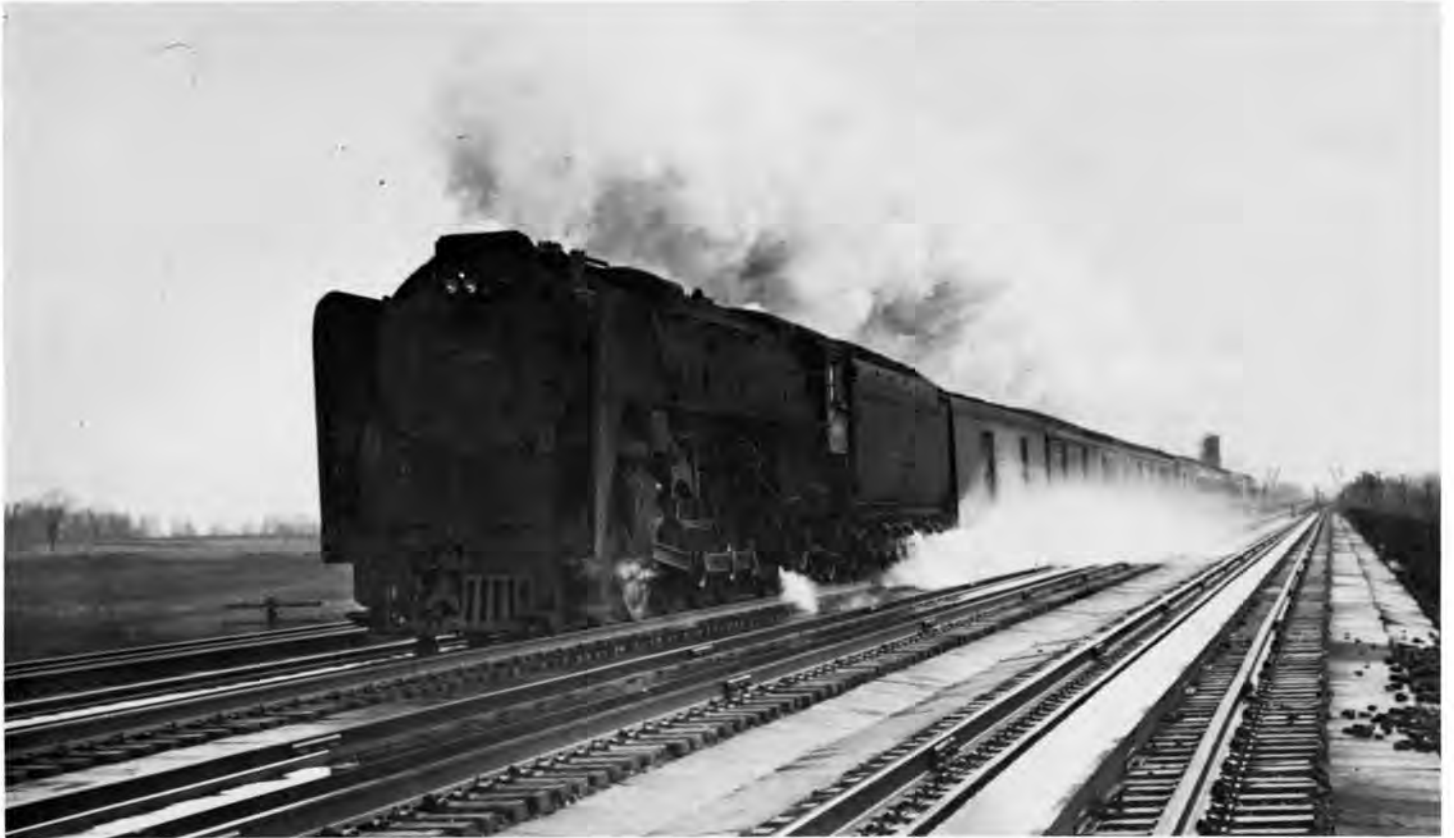
N.Y.C. Niagara 6020 with train No. 43 scoops water from the Silver Creek, N.Y. track pans on a rainy February day in 1949. Much testing and design work went into equipment to make this operation possible. Photo by H. L. Vail Jr.
