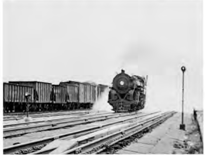
No. 5328 scoops water on test with the old design scoop. Note the excessive spillage of water from the track pan. To the left and right of picture are the purple light standards indicating the end of the pans.
