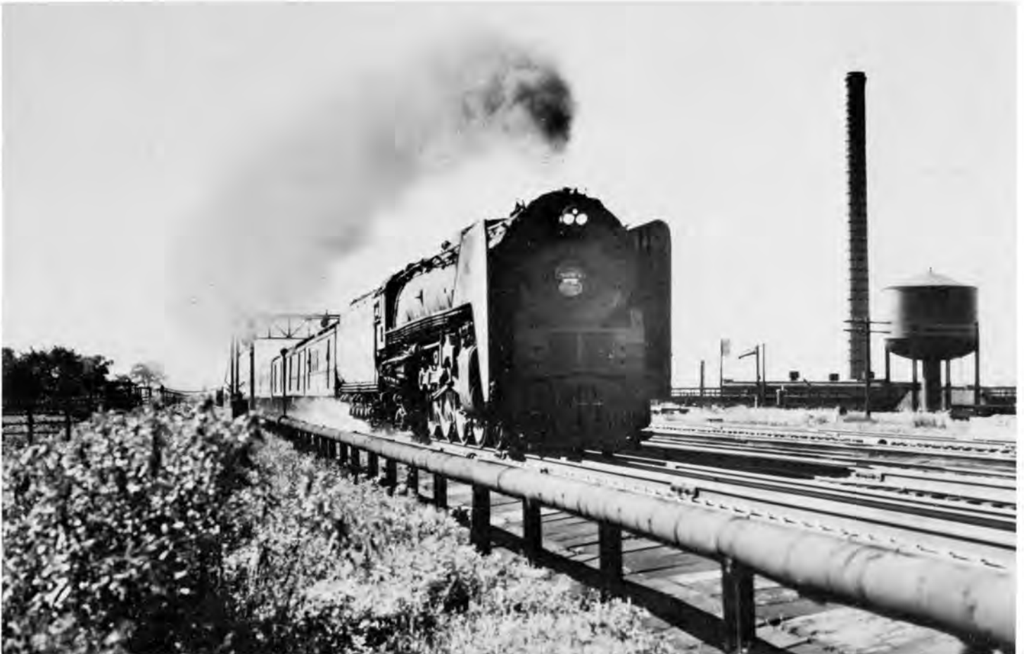
N.Y.C. Niagara 6005 scooping water into her 18,000 gallon, PT-5 tender at Rome, N.Y. in 1951 while pulling the "Empire State Express." Note test result data gathered using this locomotive and tender dated November 14, 1945. Bob Lorenz Collection
