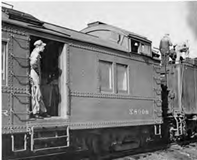
Dynamometer car coupled to tender. Carl Kantola and Fred Beach on top of tender tank, locomotive #5328. Carl F. Kantola
