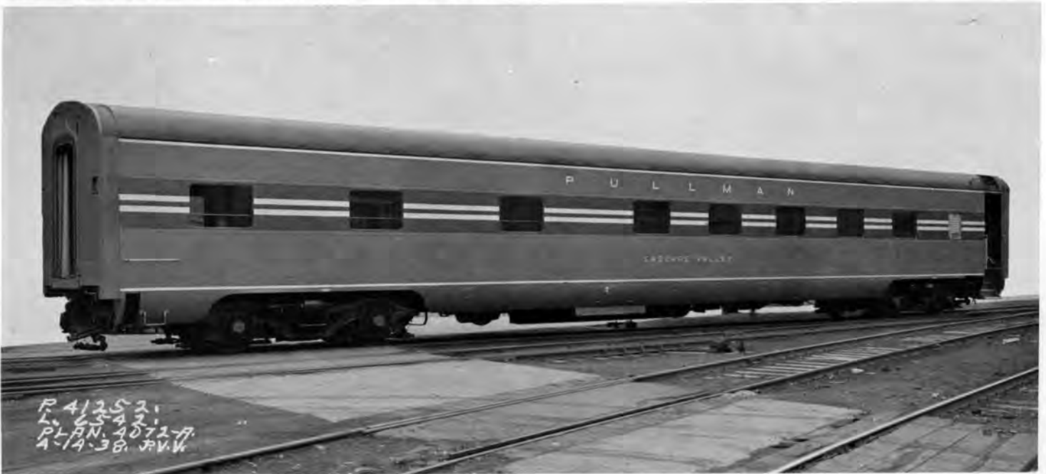
1938 "Century" Pullman "Cascade Valley", 10 Roomette - 5 Double Bedroom, corridor side original paint and striping. New at Pullman plant 4/14/1938. Pullman Photo, Collection A. K. Bush
