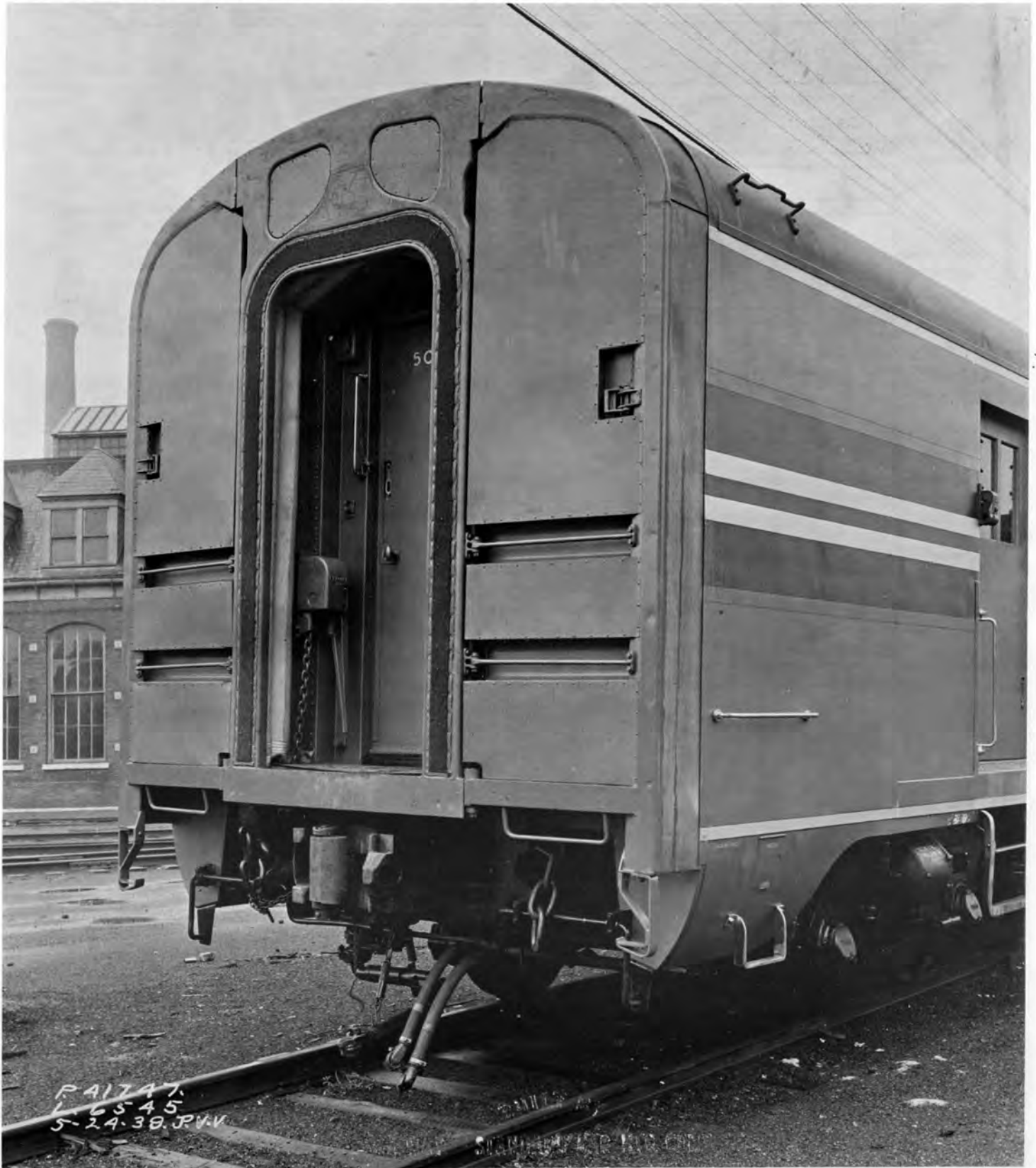
NYC Baggage Mail Lot 2130, showing Striping as built 5/24/1938. Note that the "Danger" notices on the ends have not been applied. Pullman Photo NYC SHS Collection
