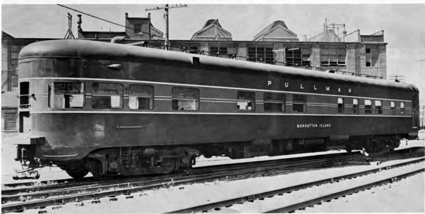
Pullman "Manhattan Island" for the "Century", shown as re-built to Pullman Plan 4079A, 4 Double Bedroom, Buffet, Lounge, Observation, with "1943" striping and with Pullman 41HR trucks. Car was originally built in May 1938, Pullman Std. Lot 6547, to Plan 4079, 1 Master Room, 1 Double Bedroom, Buffet, Lounge, Observation, equipped with Pullman 43-R trucks. Photo Collection George E. Votava
