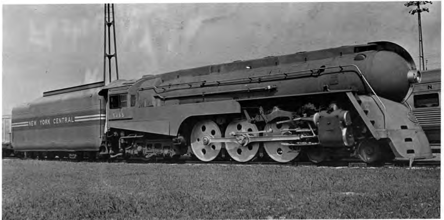
Power for the 1938 Twentieth Century Limited was provided by 10 Alco J-3a Hudsons that were given beautifully designed streamlining by Henry Dreyfuss to match the new passenger cars. Locomotives 5445-5454 were considered by many to be the best appearing streamlined steam engines ever built. Hudson 5453 shows her graceful lines for her proud owners at Flushing, N. Y. on August 6, 1939, at the Worlds Fair of 1939-40. The streamlined shrouds were removed from all of these locomotives by 1947.
