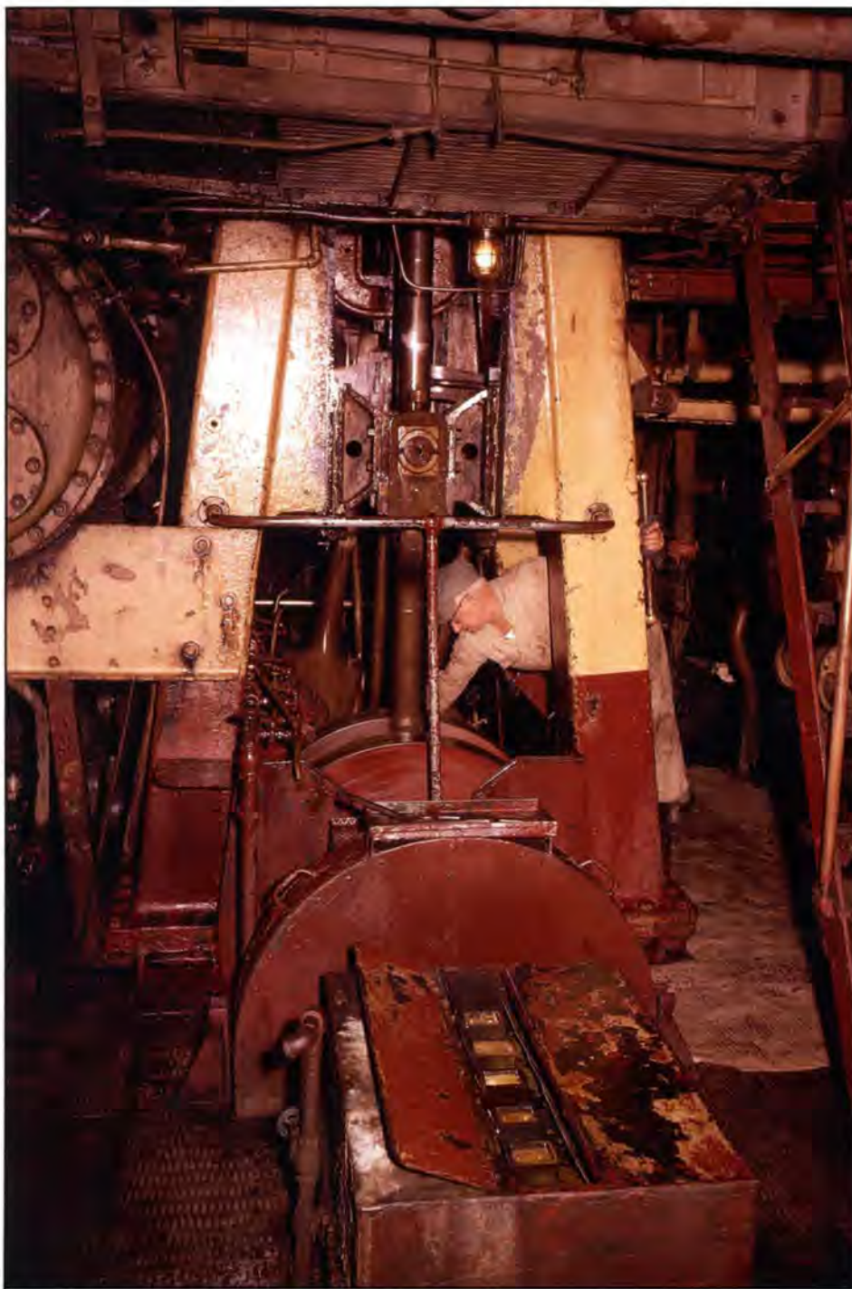
On the lower deck of Tug No. 32 , the oiler checks the temperature of the steam engine's crankshaft bearings by feeling them as they rotate. This sounds incredibly dangerous, but it was part of the oiler's daily routine. At left is the condenser, and in the foreground is the thrust bearing. The cylinders are out of sight on the deck above. November 1966 photo by Conrad Milster.
