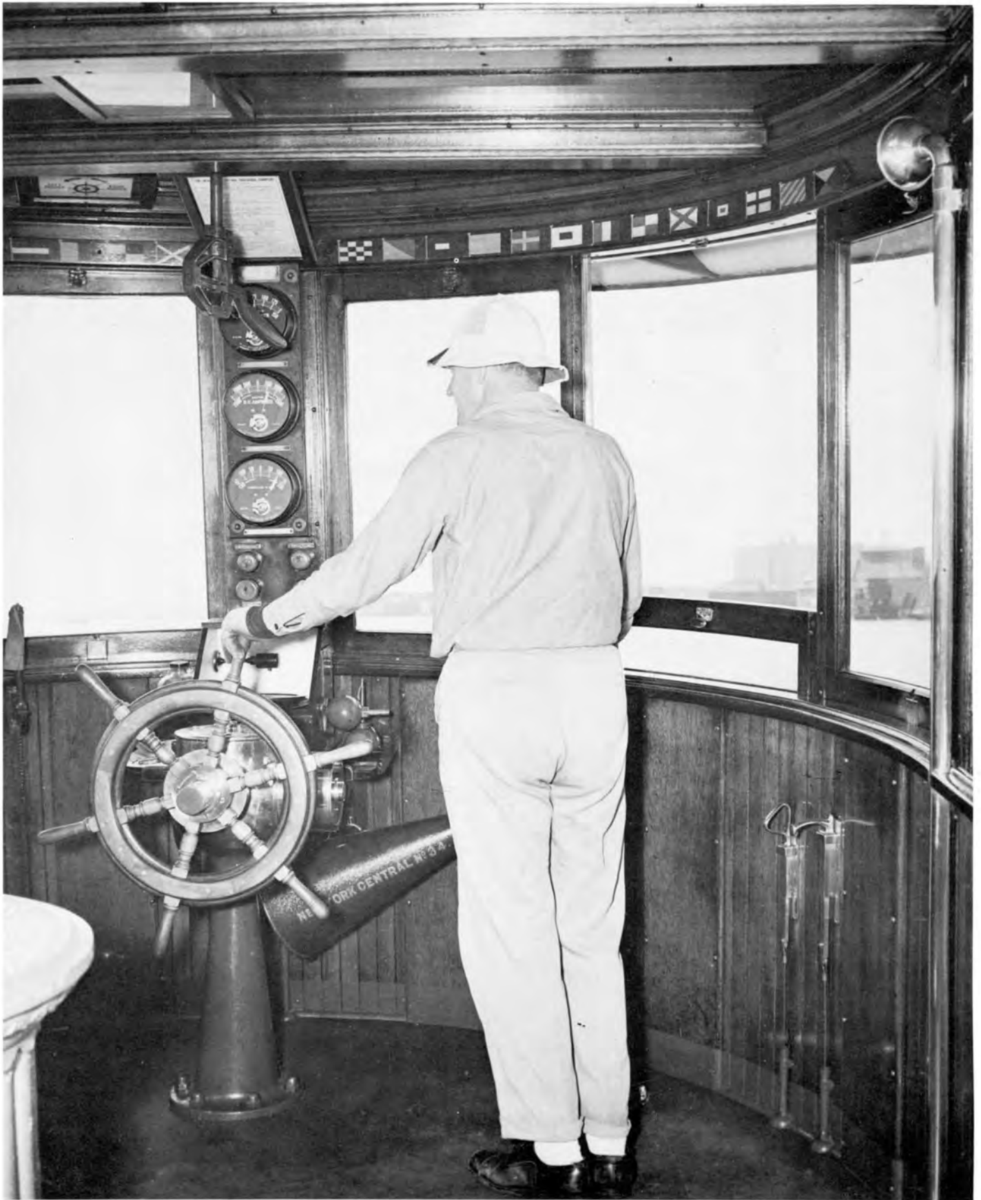
A later view of the wheelhouse of NEW YORK CENTRAL NO. 34, with a small wooden wheel in sharp contrast to the huge brass one shown on page 7 of the brochure, and the master's garb equally far from the business suit and fedora of old. Only a bit of the base of the engine control is visible here, and the floor tile has been replaced with plain linoleum. New York Central System photo, from Collection of Robert G. Herbert, Jr.
