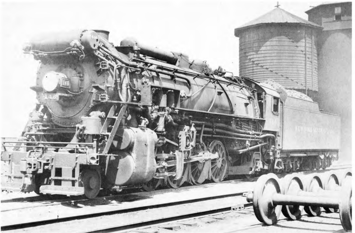
The earliest available photo of H10a #146, later #2246. 8" Roman lettering on the tender indicates that it was taken after 1928. Headlight is an 18" size by Sunbeam Electric Mfg. Co. Photo by G. Grabill, Jr., Rail Photo Service, Curl collection.
