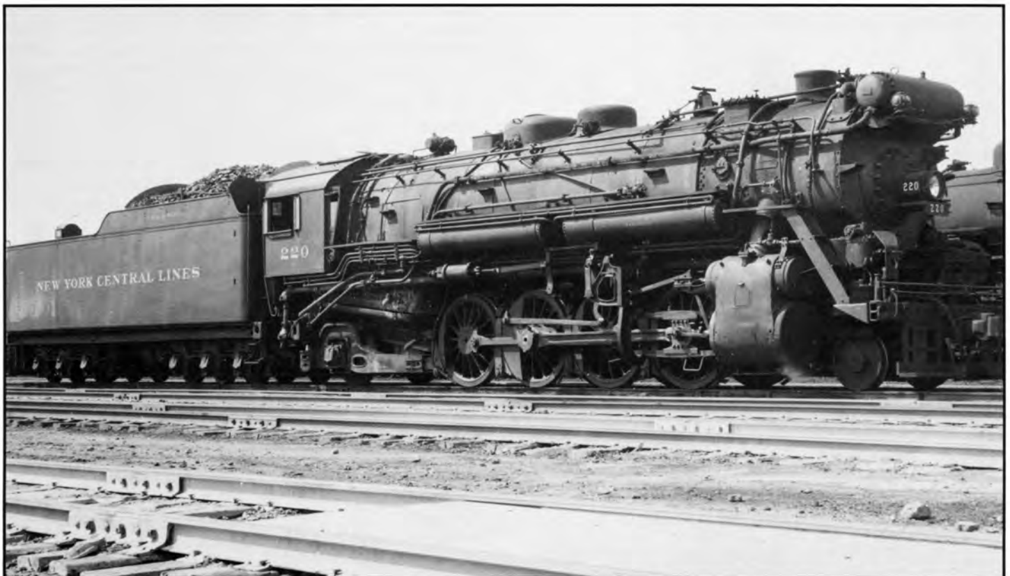
H10b 220, later 2320-2078, at Indianapolis, Indiana, August 16, 1936. Note tender lettering is 8" Roman and is the "Lines" configuration, with "CCC&StL" on the coal board. Photo by J. H. Westbay.
