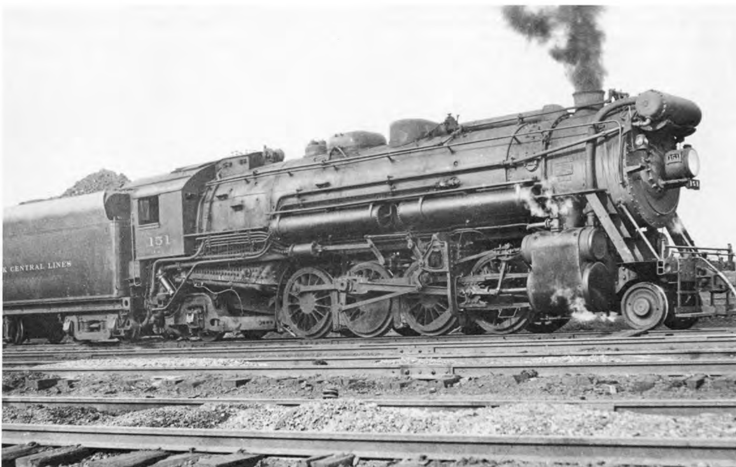
H10a #151 in her early years. Note the 18" Dressel headlight and the 8-wheel tender, R. S. Curl collection.
