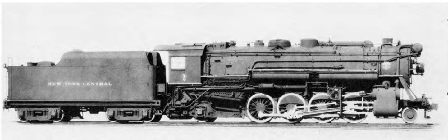
Right side builder's photo of the first production H10a #1. Built by Lima in September 1922, B/N 6357.
