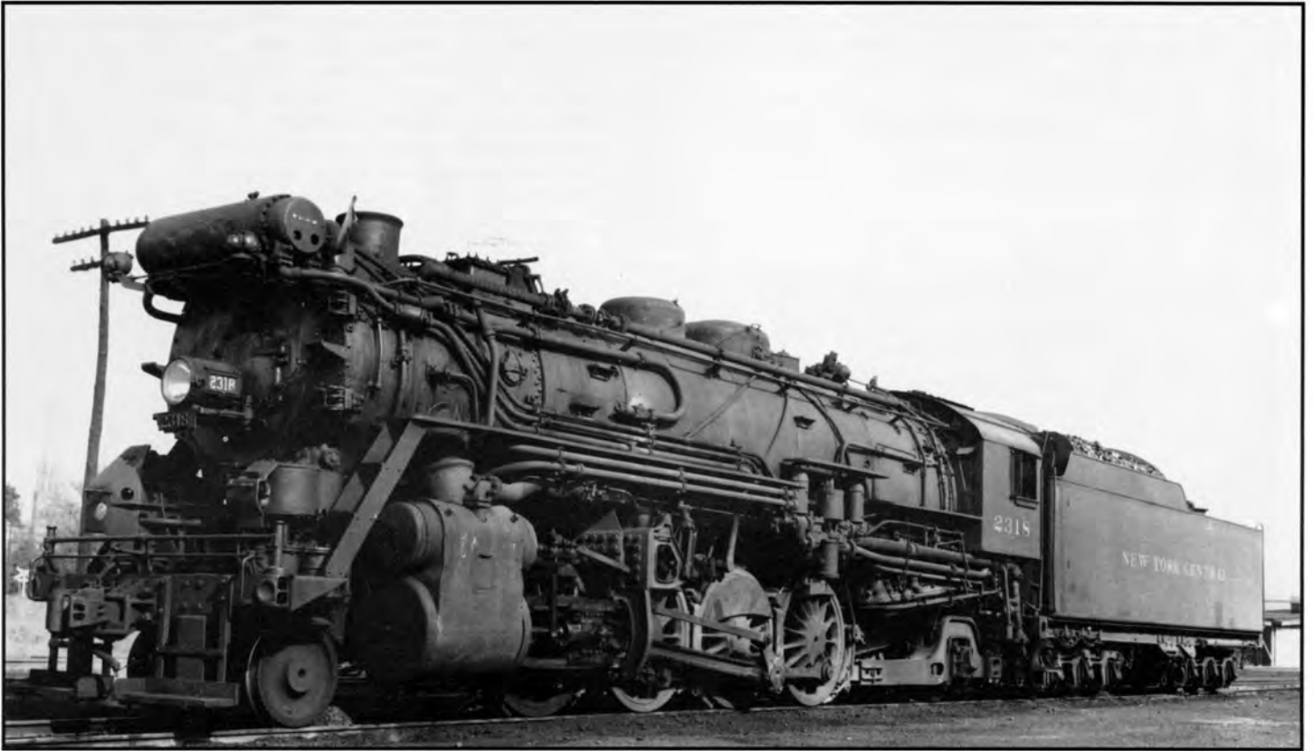
H10b 2318, later 2076, May 1940. Note that engine is still equipped with external pipe to supply superheated steam to turret. Photo from Joseph Brauner collection.
