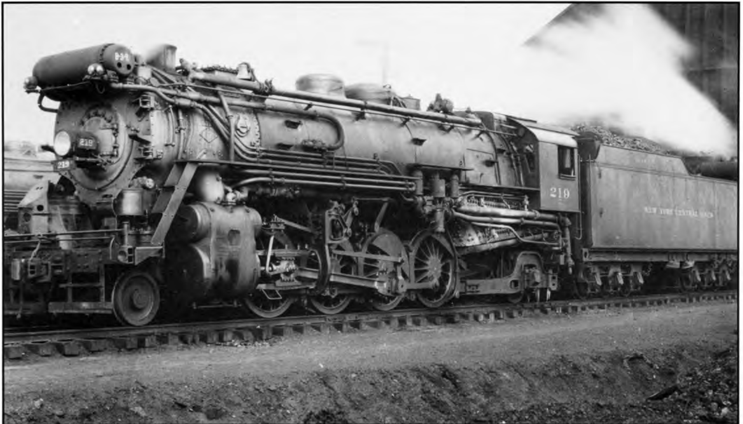
H10b 219, later 2319-2077, was less than a year old when photographed at Bellefontaine, Ohio on March 31, 1925. Note that tender lettering is the then-standard 5" Roman. Photo by J. H. Westbay.
