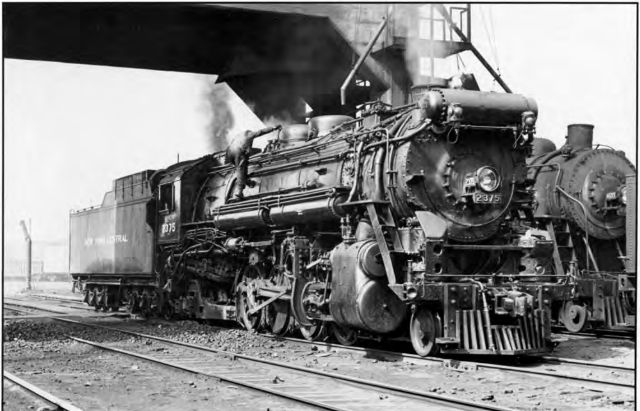
H10b 2375 at West Detroit, Michigan in 1947. Note auxiliary coal boards on tender. Photo by Robert A. Hadley.
