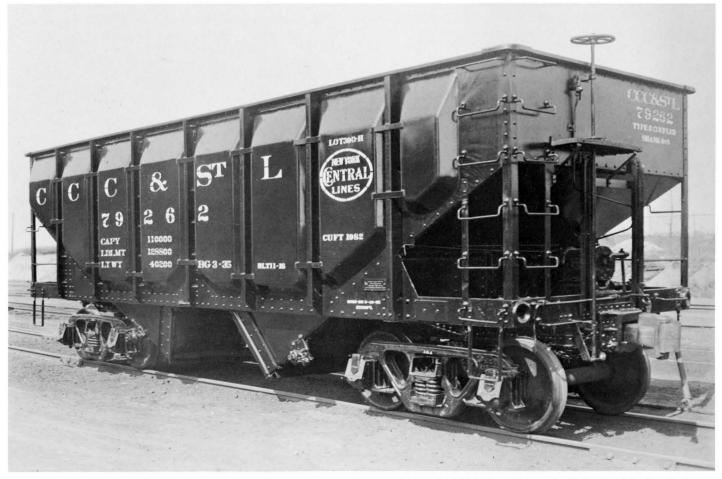
CCC&StL 79262, Lot 390-H, is shown after rebuilding at the Beech Grove, Ind. shops in 1935. New sides are the Union Metal Product Co.'s pressed panel design with integral stakes. Note the stencilled cubic footage of 1982, which is increased from the 1880 cu. ft. of the as-built car. Trust plate has been reapplied below the oval, just above side sill.
