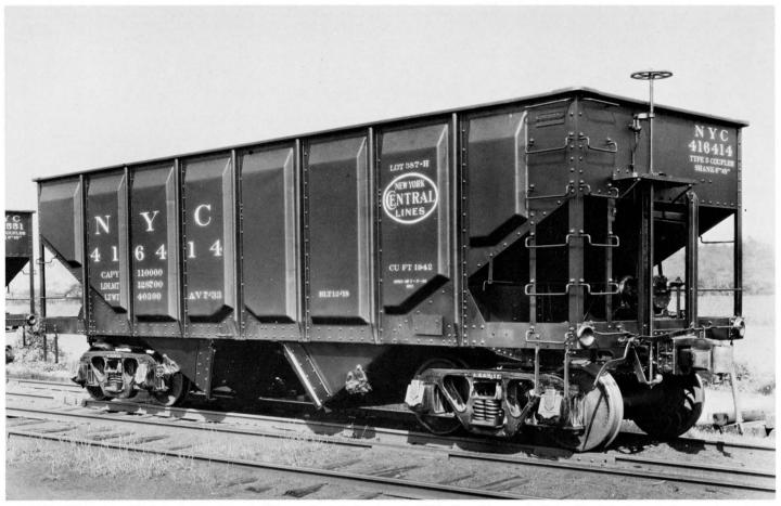
NYC 416414, Lot 387-H, is shown after rebuilding at the Avis, Pa. shops in 1933. New sides are the Union Metal Products Co.'s pressed panel design with separate stakes. Note the stencilled cubic footage of the 1942, which is increased from the 1880 cu. ft. of the as-built car. Trust plate has been reapplied at the right corner, below top ladder round.
