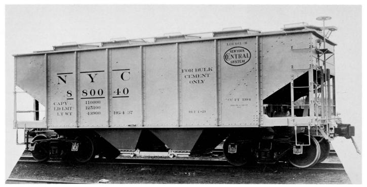
NYC 880040 was one of 105 cars from Lot 449-H which were converted to covered hoppers at Beech Grove in 1937 and assigned Lot 661-H. Note the row of rivets marking the location of the new and steeper slope sheet required for the handling of cement.
