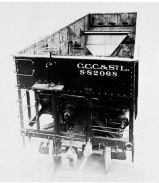
View of Big Four S-82068 showing B-end and interior detail. Note that this car has a wheel-type hand brake as built, and two interior crossties and a crossridge in lieu of the three crossties used on earlier cars.
