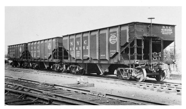
These three cars from Lot 387-H (416152, 416414, 416551) were rebuilt at the Central's Avis, Pa. shops in 1933 using the Union Metal Products Company's pressed steel paneled sides with separate stakes. Note also that the original drop lever hand brake has been replaced with a wheel type.
