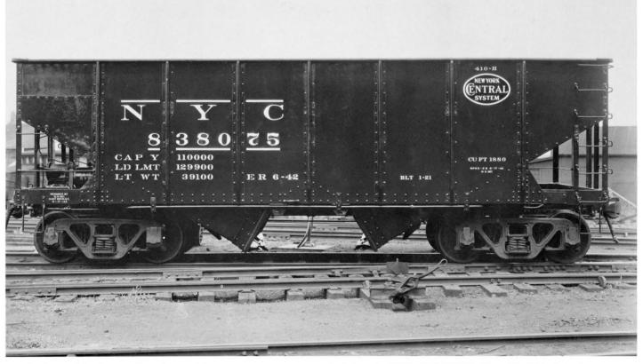
Ready to rejoin the war effort after receiving repairs at East Rochester, N.Y. shops in 1942 is NYC 838075. The original side design has been retained, and note that some side sheets have been only partially replaced. The "K" type brake appears to have been retained on this car.
