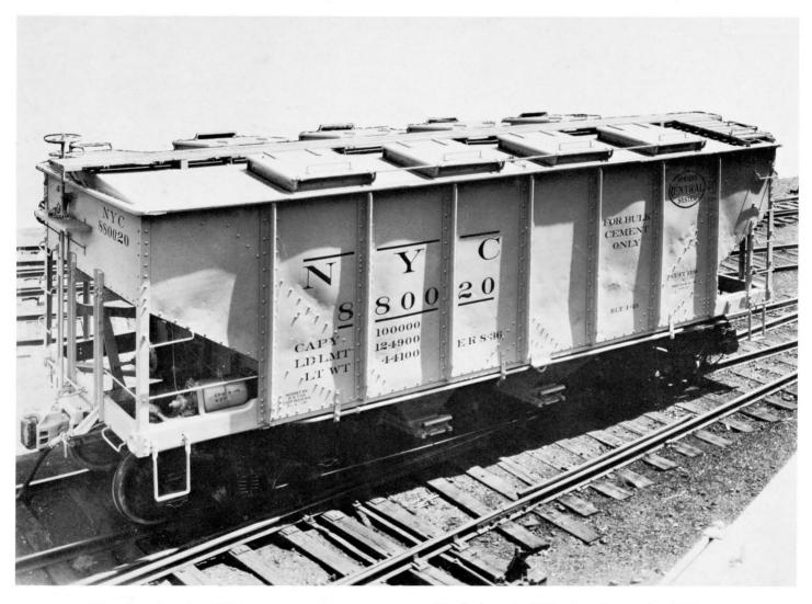
Twenty additional cars from Lot 449-H were converted to covered hoppers at East Rochester in 1936 and reassigned to Lot 647-H. These cars are painted gray and carry the new system number series assigned in that year.
