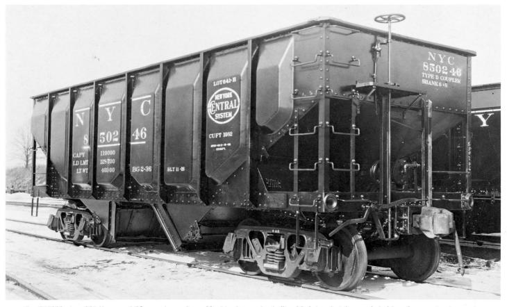
Car 850246, Lot 641-H, one of 90 cars drawn from 12 older lots and rebuilt with integral stake paneled sides of copper-bearing steel at Beech Grove in 1936.
