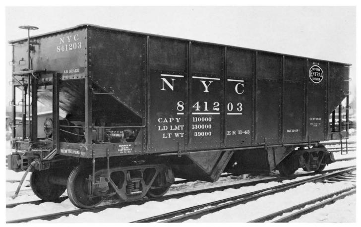
B end view of NYC 841203 after application of "AB" brake equipment at the 1943 shopping. Also note support angle remaining on ladder stile and originally used for brake step of lever type hand brake.
