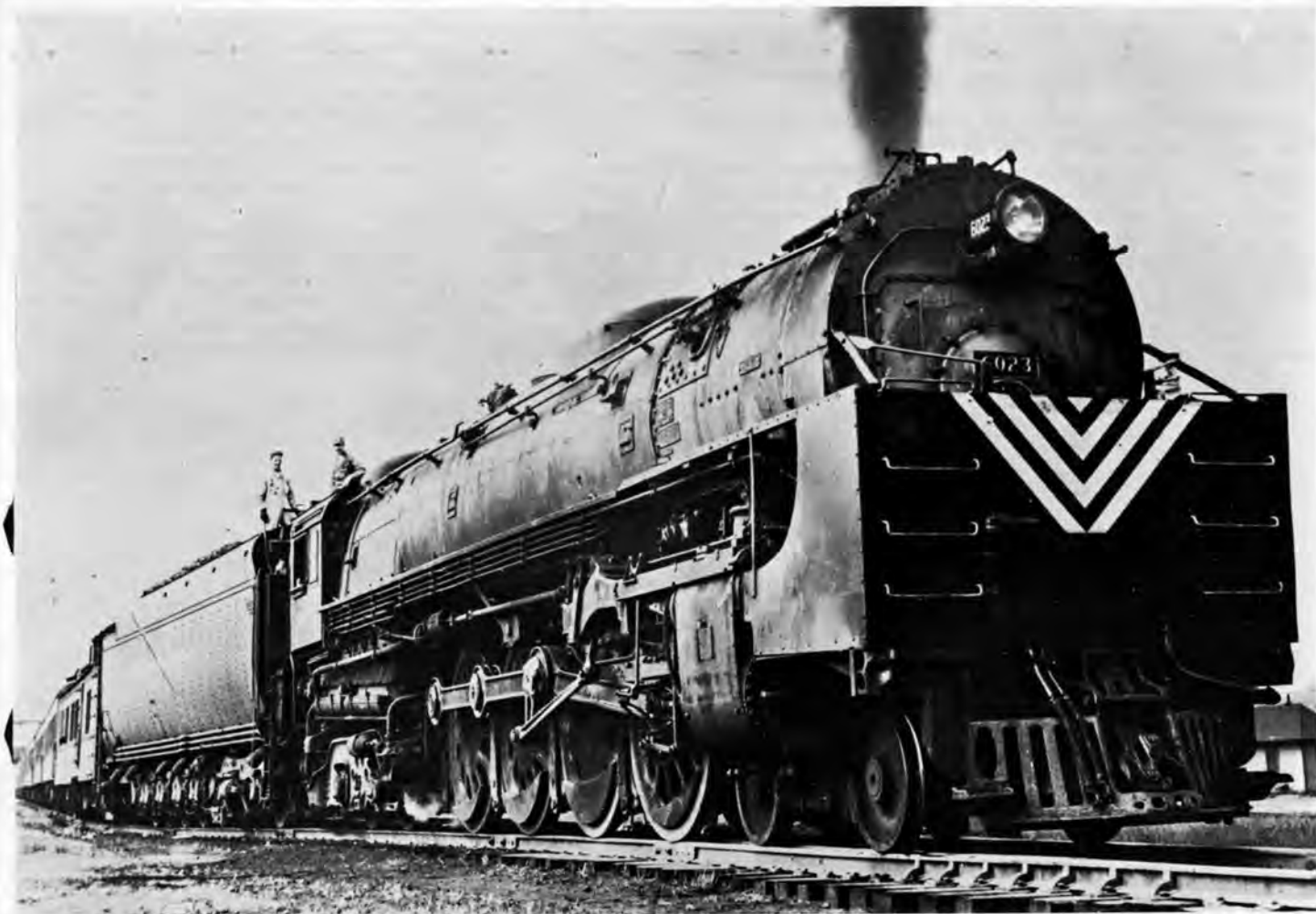
Niagara 6023 pauses after the August 1946 test in which she pulled 22 Pullmans. The crew seems to be taking a well earned rest atop her cab and giant PT-5 tender. Arnold Haas - NYC - Charles E. Winters Collection
