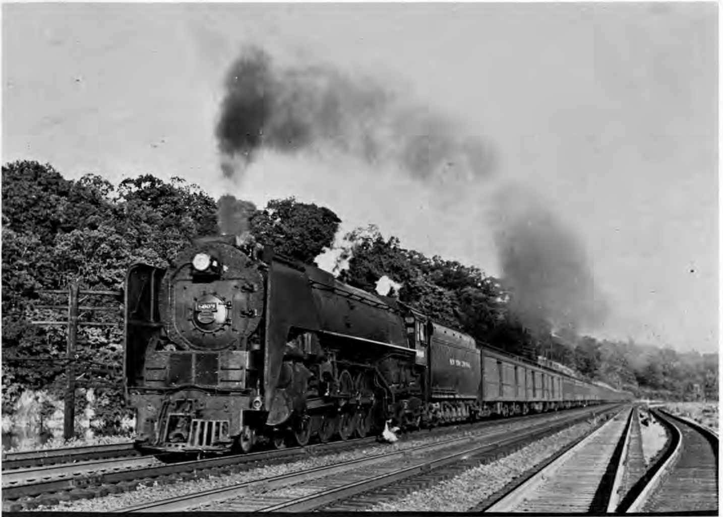
These engines were built with the most advanced technology possible in 1945. To save weight, aluminum was used for fabricating the cabs and running boards. Axles were made of carbon-vanadium steel, and crank pins of Timken high - dynamic steel, while main and side rods were manganese vanadium.
