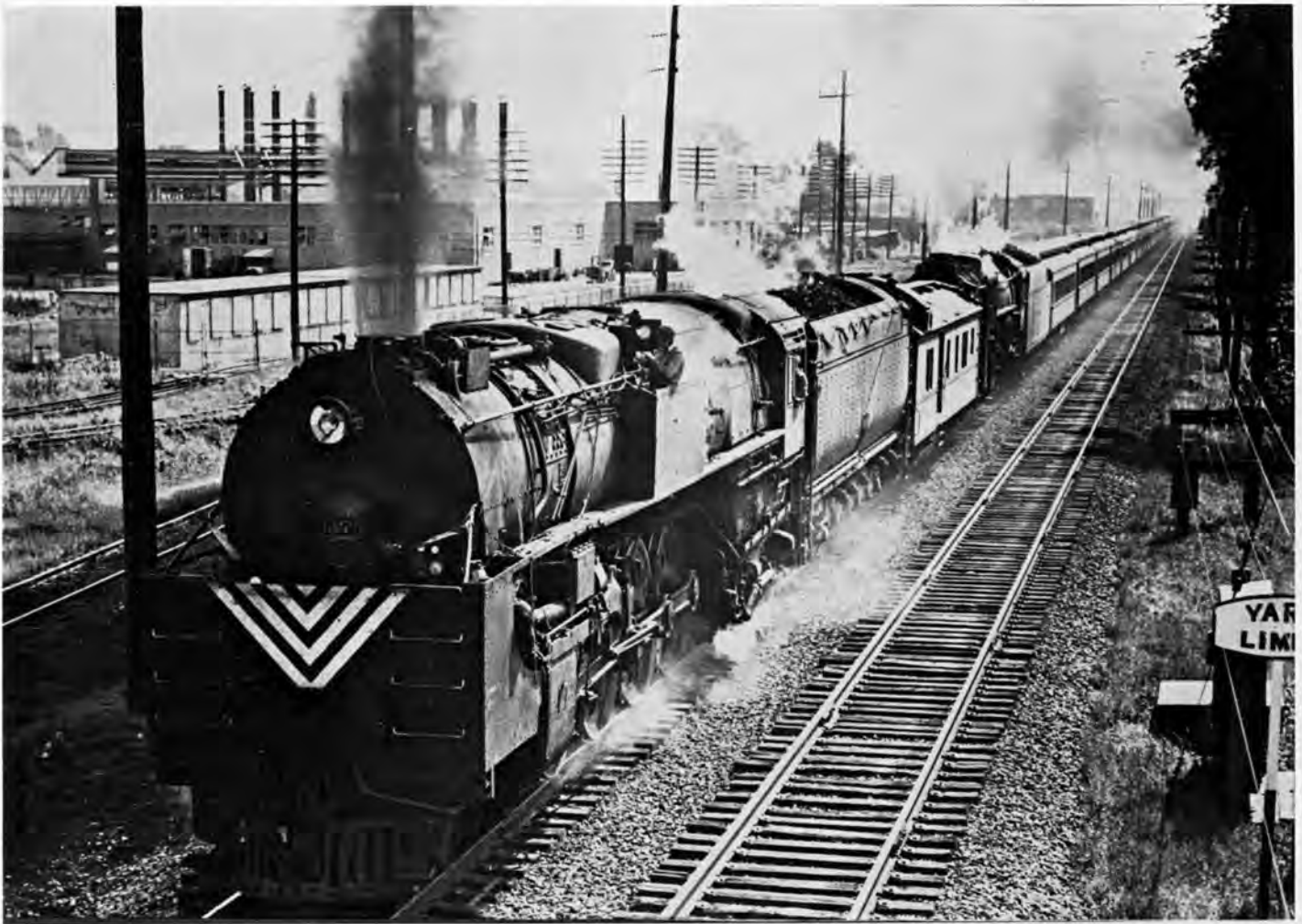
N. Y. C. 6023 with test train including a 4-8-2 Mohawk coupled on behind Dynamometer car X-8006. Note test crew in position behind special enclosures on pilot deck and running board and absence of smoke deflectors. Arnold Haas - NYC Charles E. Winters Collection
