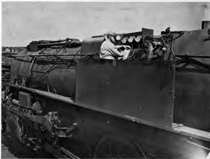
Operator prepares left side indicator for testing. Note string which rotates card mounted on cylinder back and forth.
