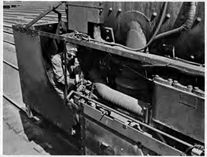
Running board enclosure and instruments. Note locking link which holds valve gear at predetermined cutoff setting for entire run. Linkage driving indicator and steam line to indicator from crank end of cylinder are also visible.
