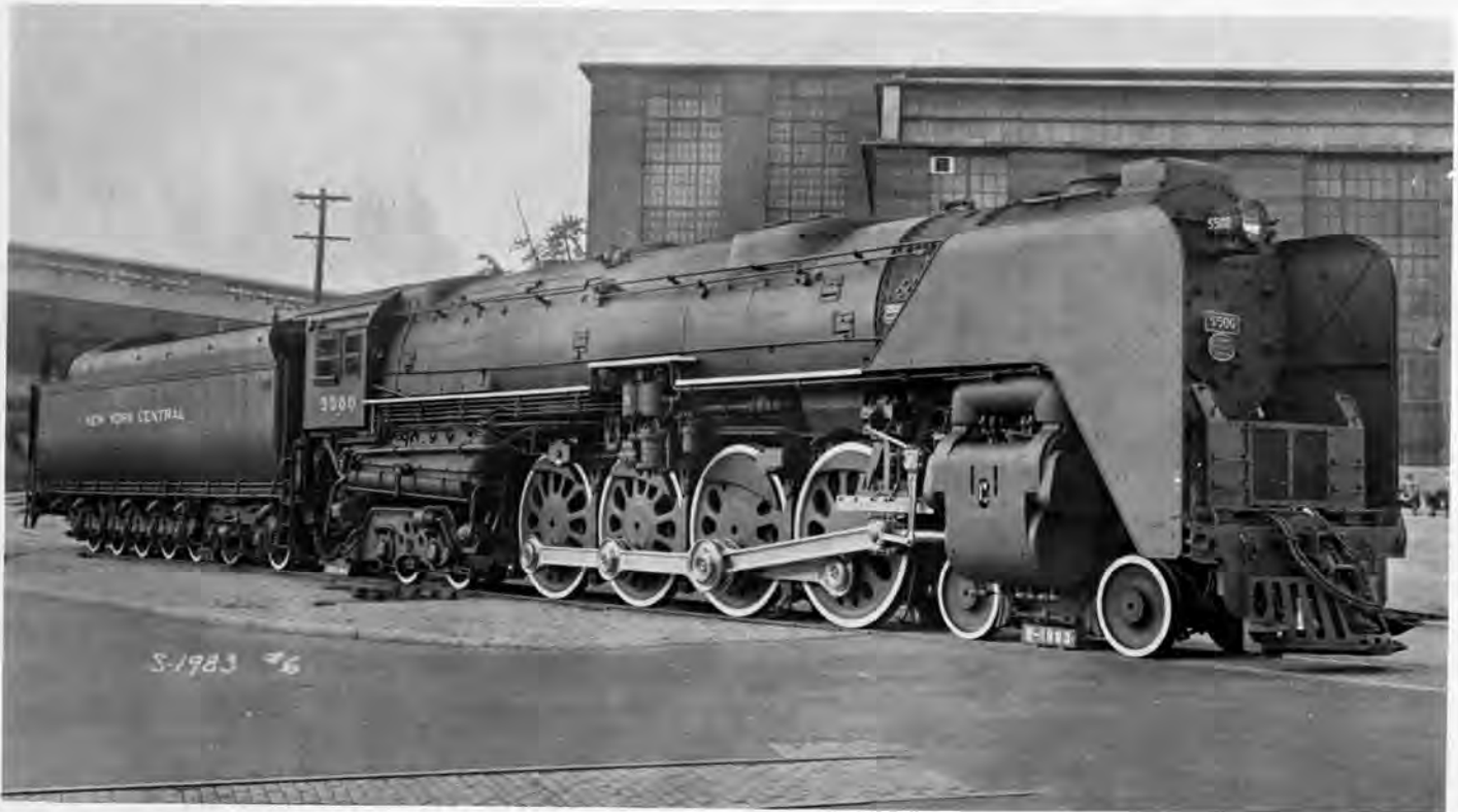
A great experiment that was born too late. No. 5500, Class S-2 displays an unusual location for a "Niagara" air pump, a relocation that was necessitated by the front mounted Franklin poppet valve gear.
