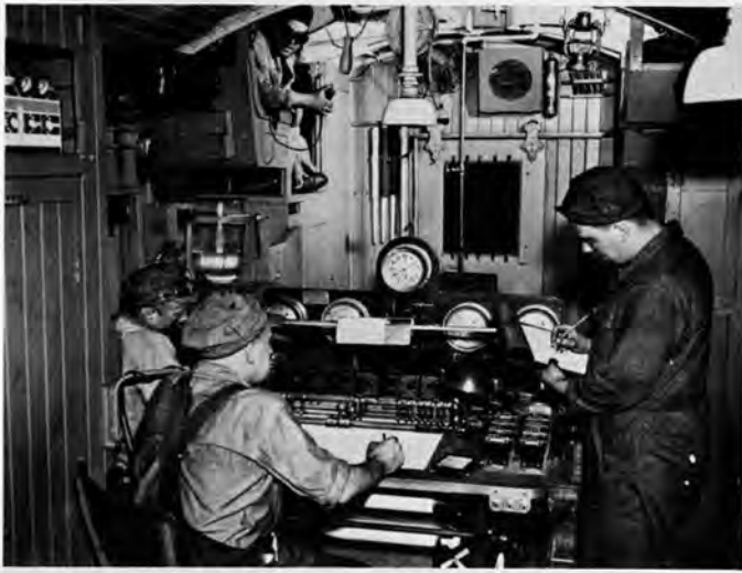
Interior of the X-8006 showing members of the test crew at the recording table. Man seated in cupola has push button to activate milepost indicator on chart.
