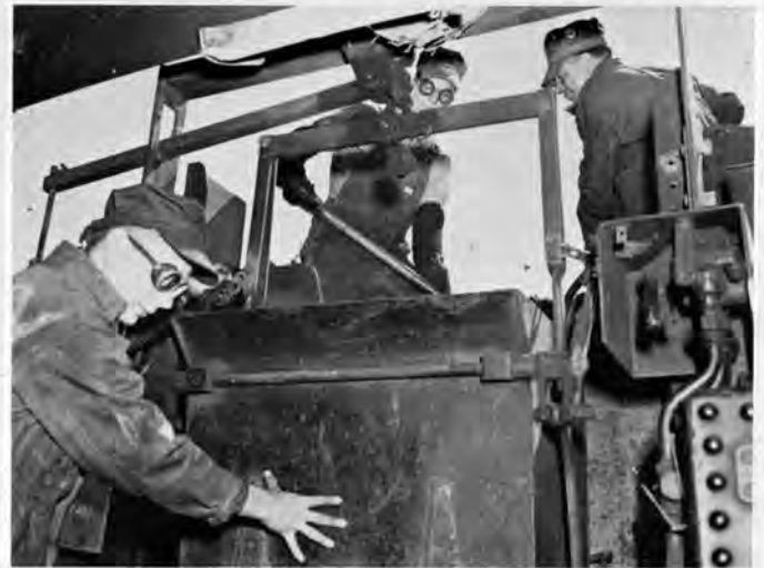
Extra firemen shovel coal into calibrated bucket as member of test crew prepares to dump coal into stoker trough when scale indicates proper weight has been loaded.
