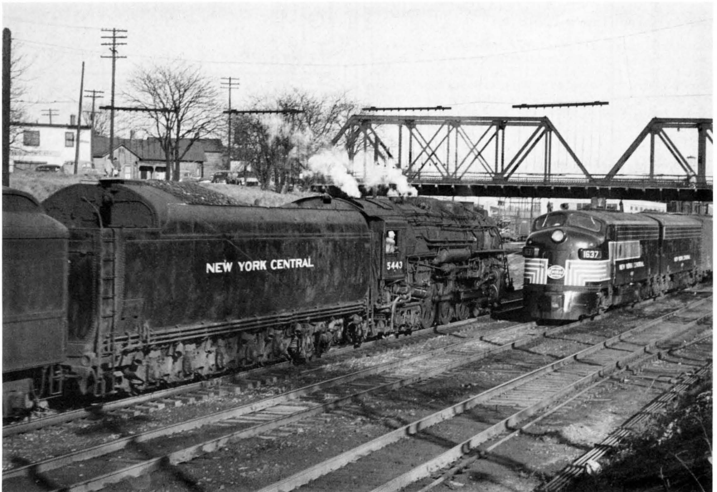
Class J3a #5445 with PT-5 tender #T-3122 near Toledo, Ohio station, 1950. Note no booster, but that #1 overflow pipe is intact. Photo from Bob Lorenz collection.
