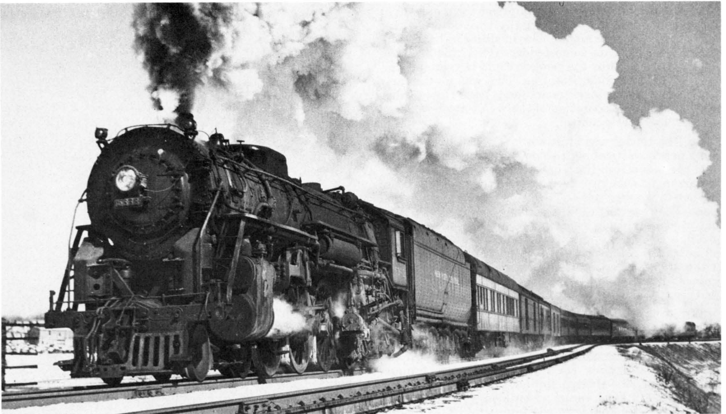
Class J1e #5333, the only J1e other than 5344 and 5401 to receive a PT tender, on train #415 westbound out of Lafayette, Ind. in February 1950. Although there is no Lima diamond builder's plate or trust plate on the tank side, the record indicates that this is a PT-4. The LLW #T-1041 was damaged 5-2-45, repaired and applied to 5333 in 9-1946, which may account for the missing plates. However, the high location of the tender lettering for a Niagara may indicate that the tender was recently changed. Note also the slightly high headlight position. Photo by H. D. Lewis.
