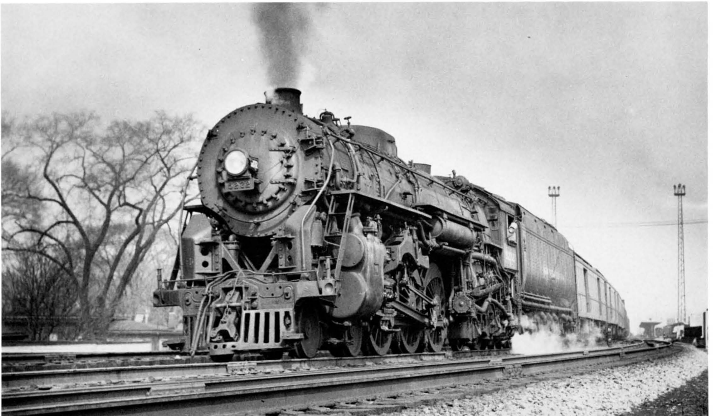
Class J1c #5272 leaving Syracuse, N.Y. with train #9, 2:55 P.M., May 5, 1950. The tender is a PT-4, although the records do not indicate that 5272 had one. The PT-3 tender previously on this engine was off by 10-49. Photo by Tom Mulaniff.
