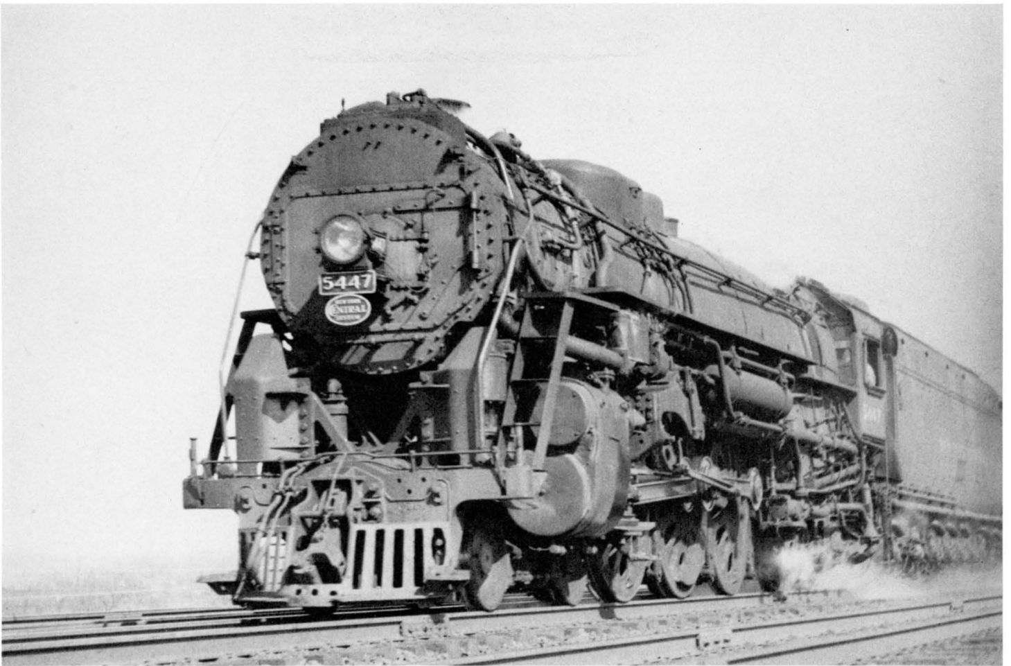
Class J3a #5447, destreamlined with original flat smokebox front, Worthington feedwater heater, booster, and PT-4 tender, on the "Advance Empire State Express." Since the photo is not dated tender could be LLW T-1078 or T-4157. Note well the Boxpok drivers and Timken rods. Neither the photographer nor the print owner noticed this, but it is the only such driver-rod combination that the author has ever seen on a Hudson. Photo by Robert Whitbeck.
