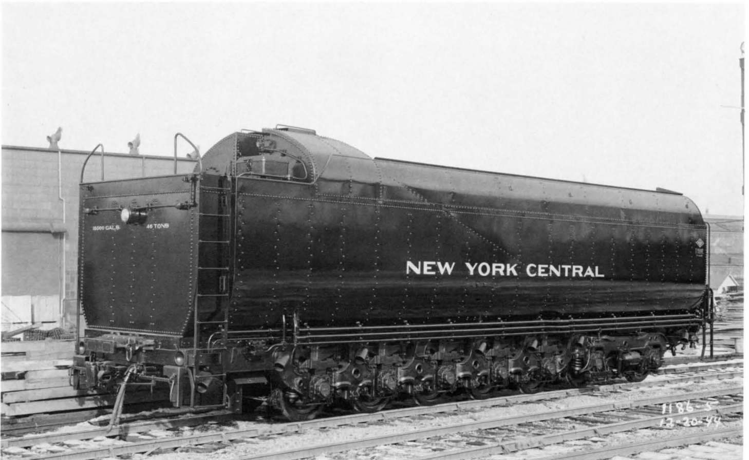
Right side/rear view of PT-4 tender. Note train control equipment box on top of tender tank, behind expansion chamber. Lima Locomotive Works photo.
