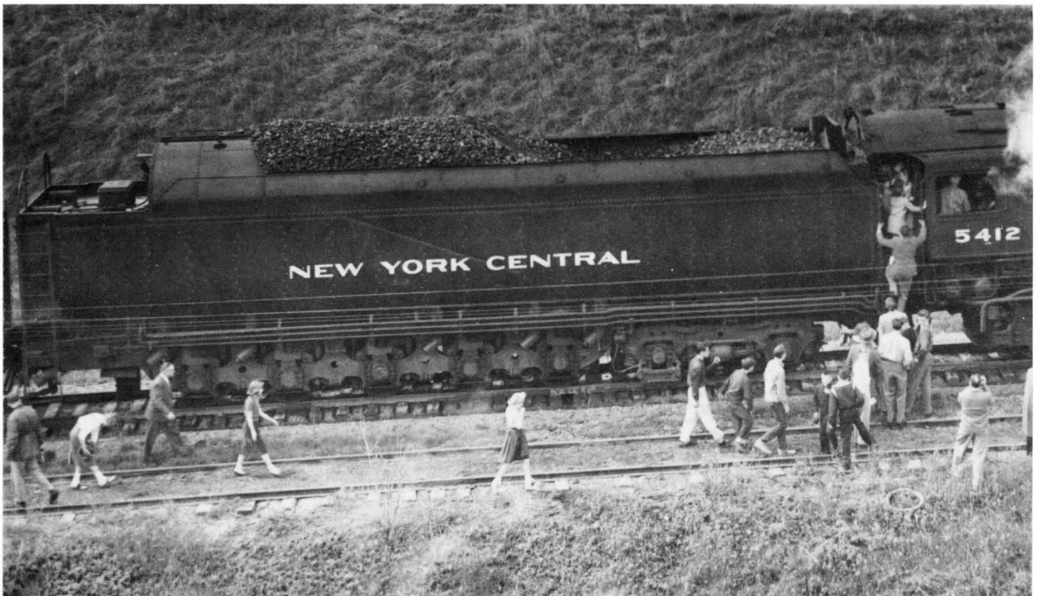
The last PT-1 (T-3113) with "overflow control," showing the expansion chamber behind the coal space, the booster exhaust pipe hole on its top side, and no Elesco skimmer since the feed water heater was the Worthington type. Note also the overflow pipes external to the tank, and the outward joggle in the conduits and pipes along the frame to clear them. Class J3a #5412 on a railfan special at Goose Lake, Mich., 10-17-54. Photo from M. D. McCarter collection.
