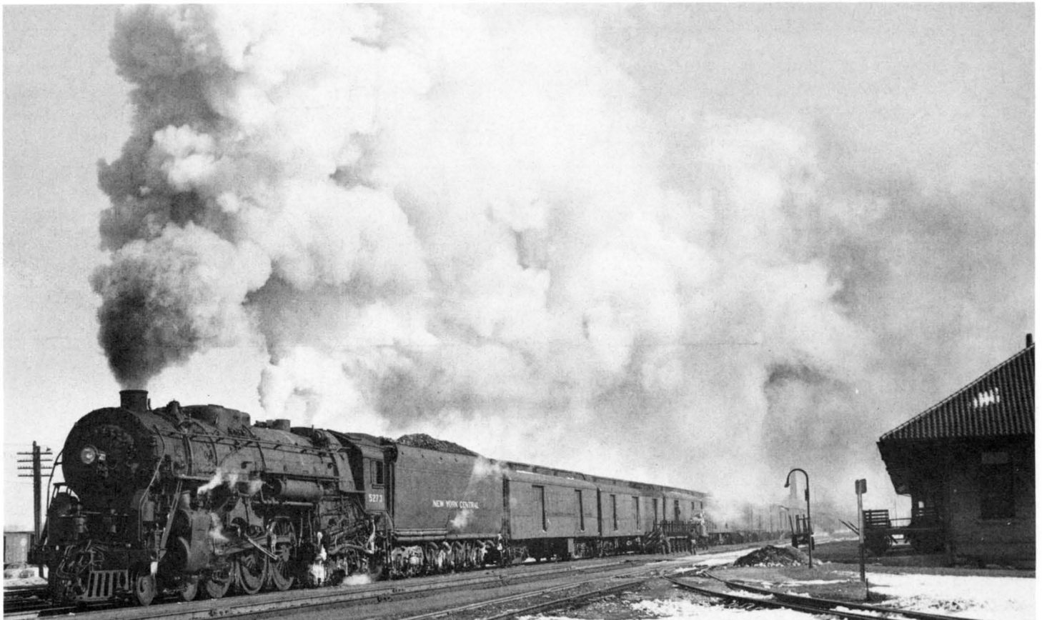
Class J1c #5273 leaving LaPorte, Ind. on 3-19-56. Tender is PT-3 #T-3598 originally applied in July 1945 when new, and never changed. Booster and #1 overflow pipe have been removed. Photo from M. D. McCarter collection.
