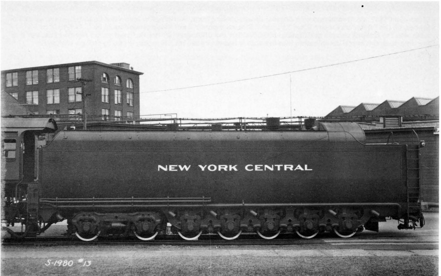
Left side of PT-5 tender built by the American Locomotive Co. Note stoker engine compartment below letters "ORK." Photo from Alco Historic Photo collection.
