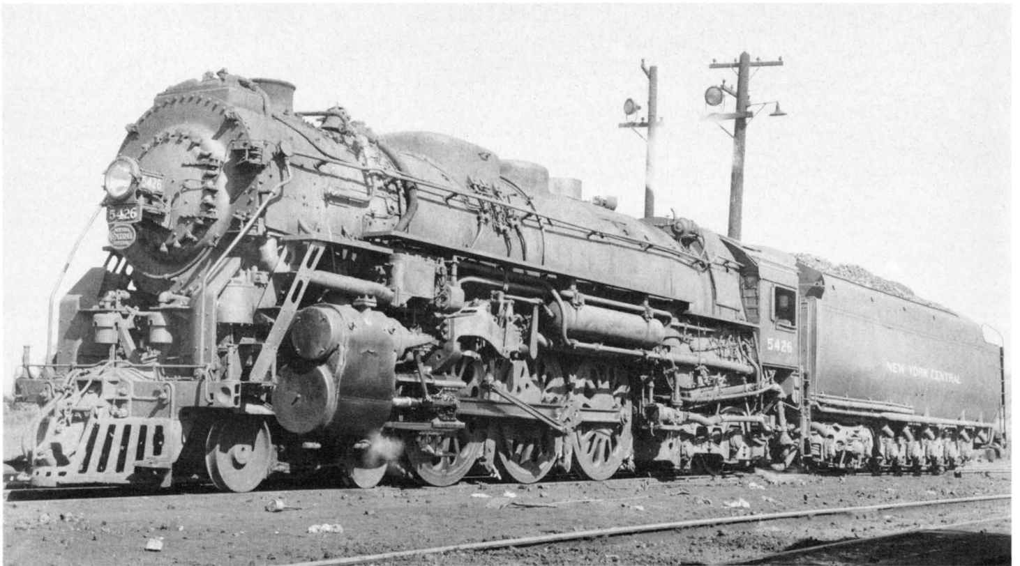
The second PT-1 (T-3635) with "overflow control." Note the overflow pipes descending from the tank side just above the steam train line, which has been moved outward, and the syphon breakers on the collar. On class J3A #5426 at Harmon, N.Y., 8-5-51. Robert J. Foster photo, from R. S. Curl collection.
