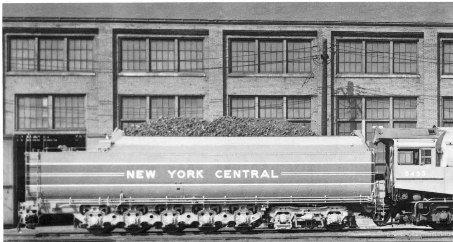
The second PT-1 tender, as new. First applied to class J3a #5453. Note no expansion chamber or overflow pipes. NYC RR photo, 5-26-43.
