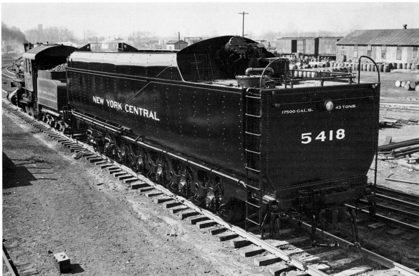
The first "PT" tender, PT-1 for 5418 at Beech Grove Shop where it was built. Note the oil skimmer for the Elesco feed water heater return on the near rear corner of the deck, and the booster exhaust muffler to the right of the coal pusher cylinder. The Pyle-National light is mounted on the muffler. NYC RR photo, 4-30-43.
