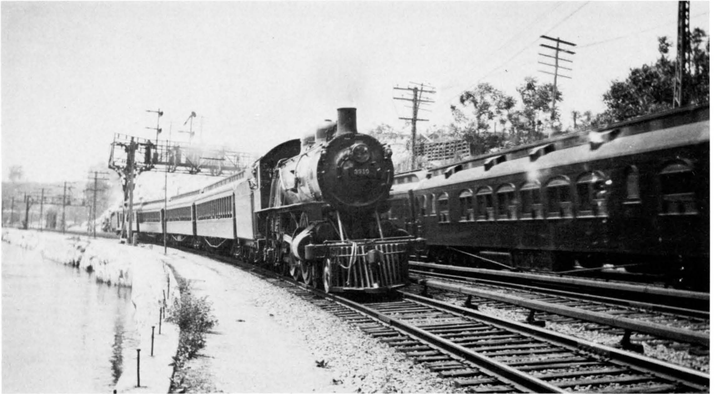
An eastbound passenger train powered by class 1d Atlantic #3910 meets a westbound at Marble Hill in New York City, about 1907 or 1908, on the then-new cutoff. "FH" tower is in the background. Note that although third rail is in place both trains are steam-powered. Photo by Emil Buchert, from the collection of his son, Philip E. Buchert.
