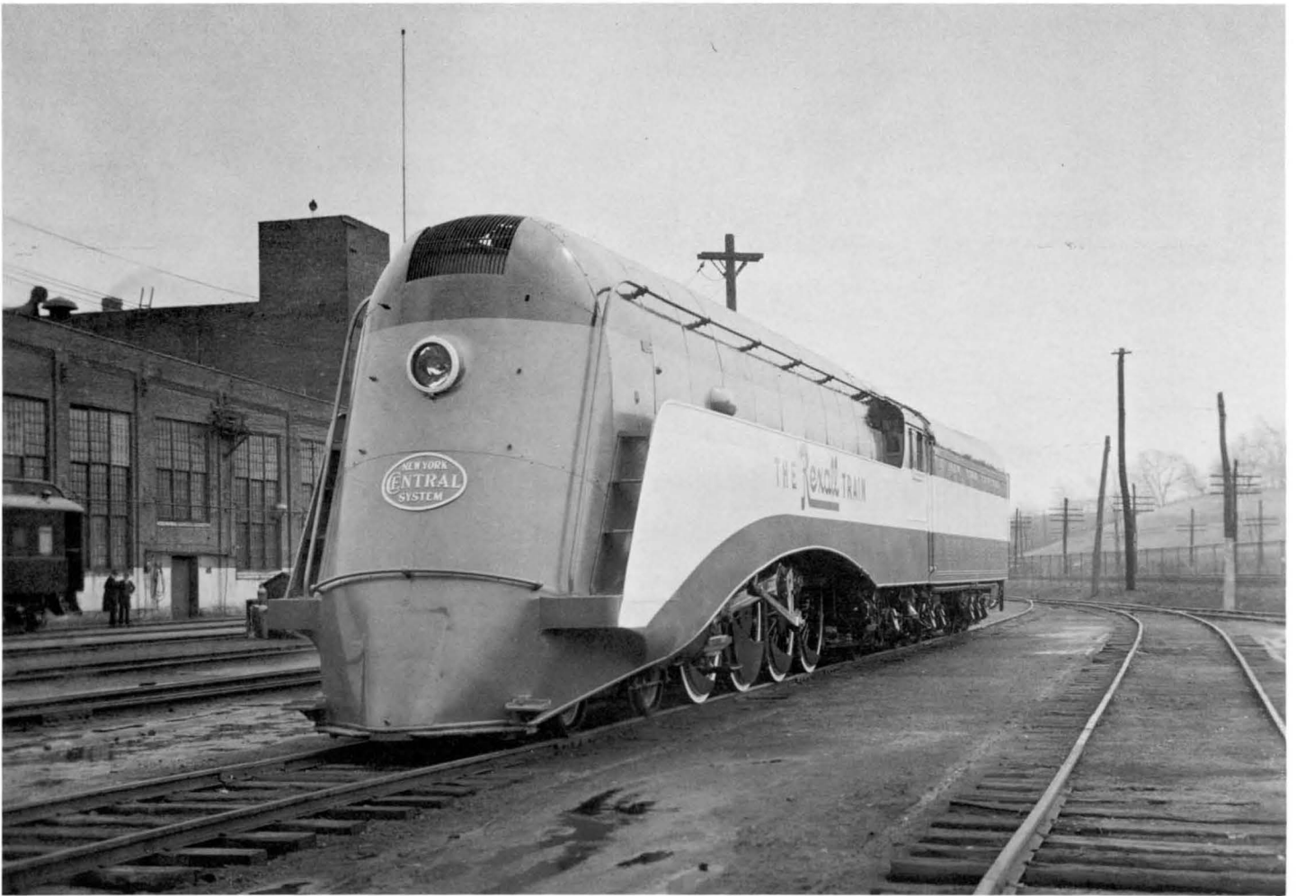
N.Y.C. L-2c "Mohawk" converted to an oil burner and streamlined for the Rexall train in 1936.
