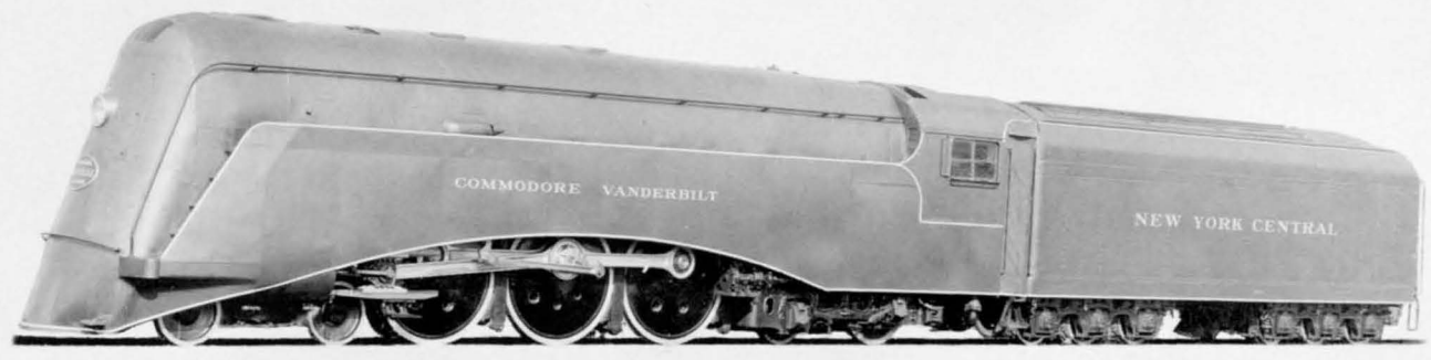
WORLD'S FIRST STREAMLINED HIGHPOWERED STEAM LOCOMOTIVE USED ON TWENTIETH CENTURY LIMITED
