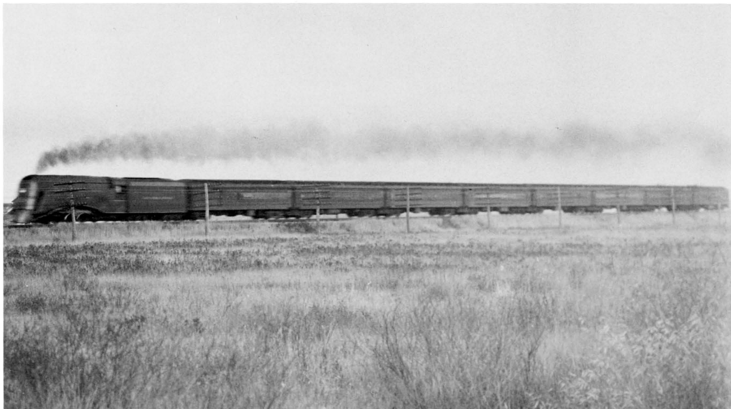
"Commodore Vanderbilt" 5344 on test run in the Albany, N.Y. area at high speed. Note the effect of the wind scoop at smoke stack lifting the smoke clear of locomotive and train. Carl F. Kantola Collection
