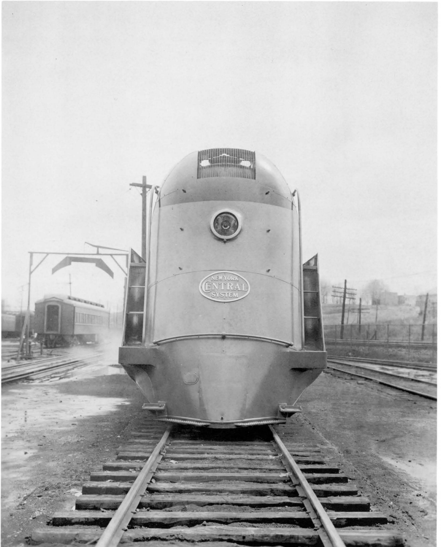
Front view of the "Rexall Mohawk" 2873 showing air scoops back of side steps and at stack.
