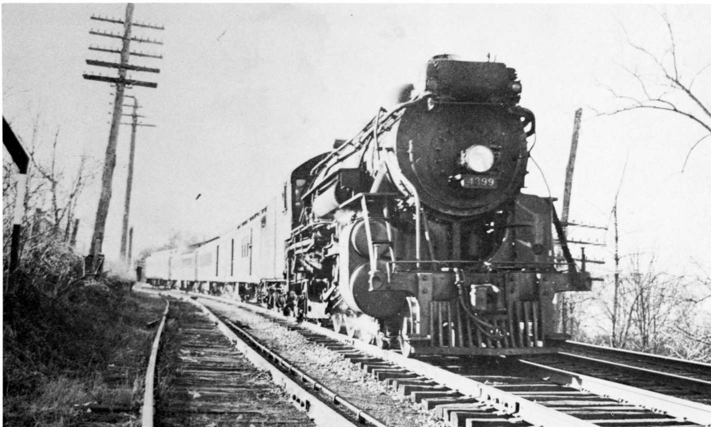
For you boys west of Buffalo, N.Y. No, this is NOT a K-5 on the Big Four or the Michigan Central! It happens to be the 4399, a K-14f leading Harlem Division train No. 5 out of North White Plains on the run to North Adams, Mass. on January 14, 1941. This locomotive was rebuilt at West Albany Shops in 1925 from K-11f No. 3193.
