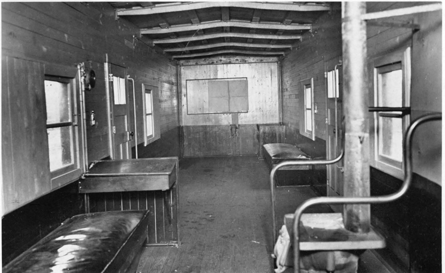
Interior shot of #18671 reveals conductor's desk, coal stove and bunks. This could hardly be considered cozy.
