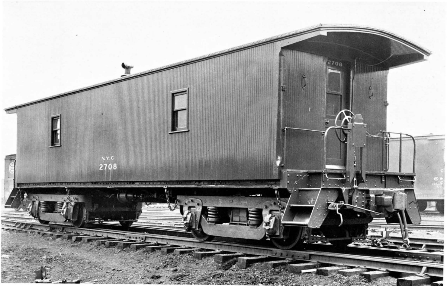
N. Y. C. rider car No. 2708, lot order No. 2168 was built in 1943. There were 20 cars in this series 2708 - 2727. This side of the car shows two windows, there were four windows on the other side as per the diagram at the top of the opposite page.
