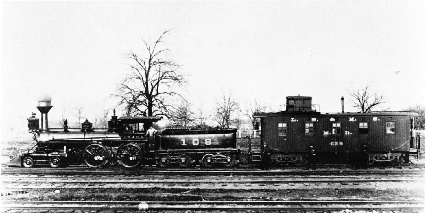
L. S. & M. S. caboose C-39 seems to almost dwarf 4-4-0 No. 108 in this early photo. The locomotive was originally named "Appachee" when it was built in 1869 by Mason Machine Co. It was retired between 1893-99. The caboose, unless it was destroyed by fire or train wreck probably survived longer. Note elaborate outside equalized trucks under the C-39.
