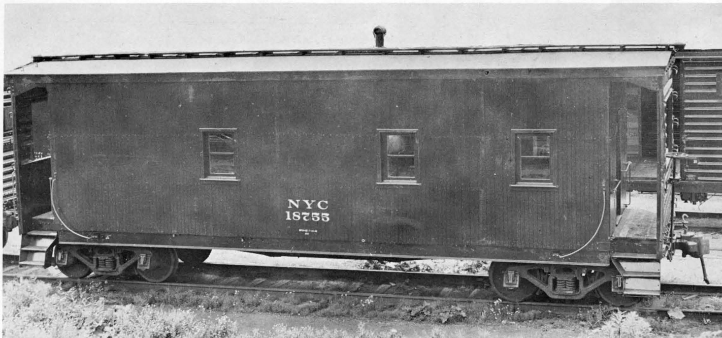
Wartime caboose #18755 shows an attempt to make the end platform steps safer by giving them more "slant". Note smooth roof without rib reinforcements showing.
