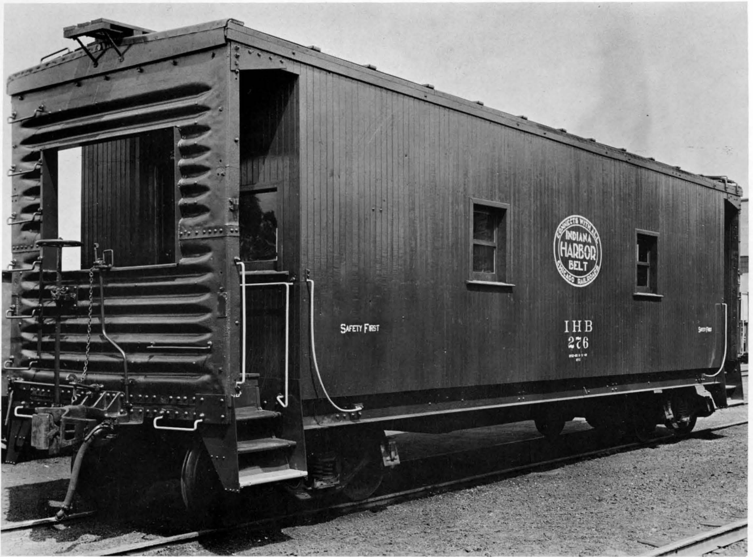
Official "Re-Builders" photo of I. H. B. temporary caboose #276. Box car ancestry is quite evident in this view.
