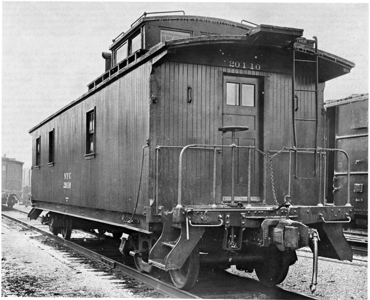
Caboose No. 20110 stands for its "builders" portrait at East Buffalo, N. Y. where it was rebuilt in 1944 from a 1910 era box car. Notice how closely this series of cars follows the general lines of the "standard" N. Y. C. caboose shown in "The Caboose Classics (Part One)". There were 50 cars in this series; No. 20100 thru 20149. Most of these, (45) were painted box car red as shown above. Five were painted Vermillion and Gray to match N. Y. C.'s "Pacemaker" high speed freight service equipment. All were built as lot order No. 732, their overall weight was 30 tons. W. D. Edson Collection
