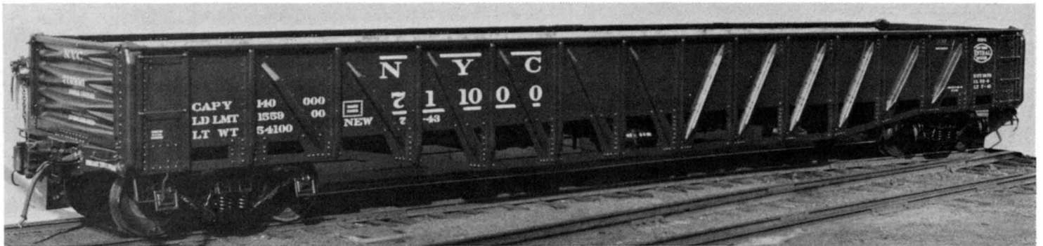
N. Y. C. 711000, 50' Composite Gondola, Lot No. 723-G, Red Car with 28 1/4" x 19 1/8" Oval.
