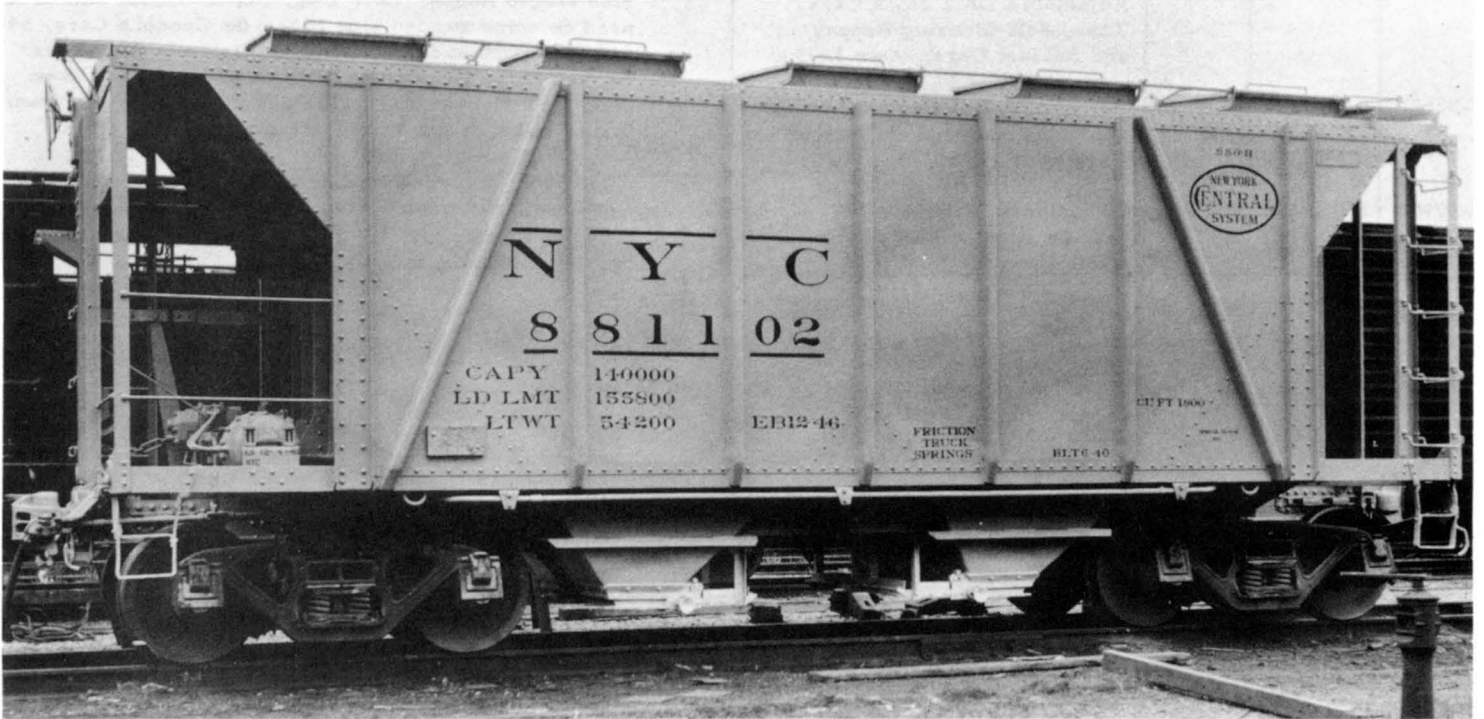
N. Y. C. 881102, 70 ton Covered Hopper, Lot No. 680-H, Gray Car with 28 1/4" x 19 1/8" Oval.
