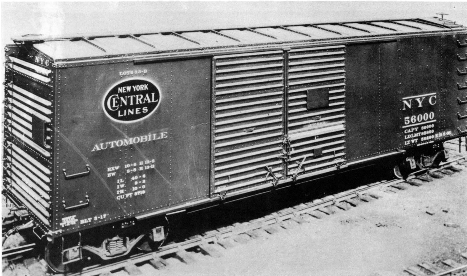
N. Y. C. 56000, 40' Auto - Box Car, Lot No. 633-B, Red Car with 48" x 32 1/2" Oval. Note reversed lettering layout because of double door design.
