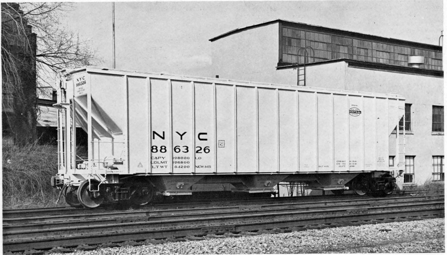
NYC 886326 is a 100 ton, 4700 cu. ft. covered hopper, part of Lot no. 959H built by Despatch Shops Inc. in April 1965. Entire body painted light gray with black trucks. Special small herald measured less than 2'-6" wide. Note that this is the only lot of cars with this herald.
