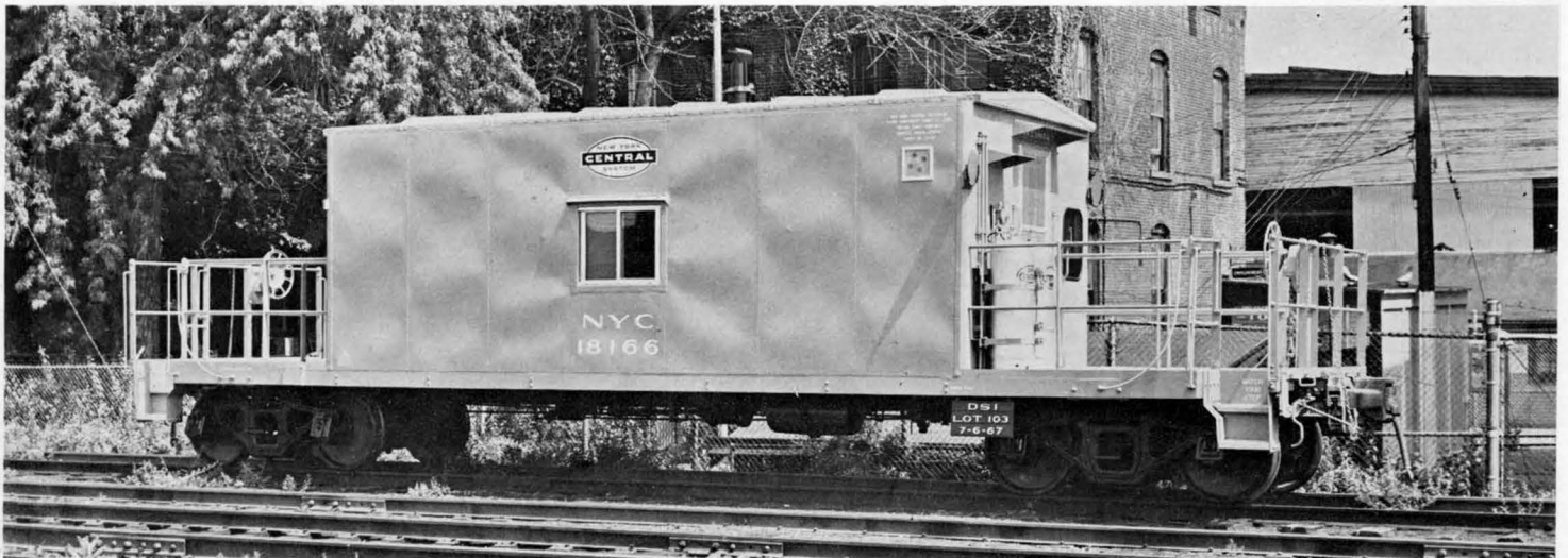
NYC transfer caboose 18166 was part of Lot no. 121, built by Despatch Shops Inc. in July 1967. Caboose was painted green with black underframe and trucks. The Oval herald size was a 33 1/8"x 15 5/8" "Scotchcal" application. These cabooses carried road numbers from retired wood cabooses.
