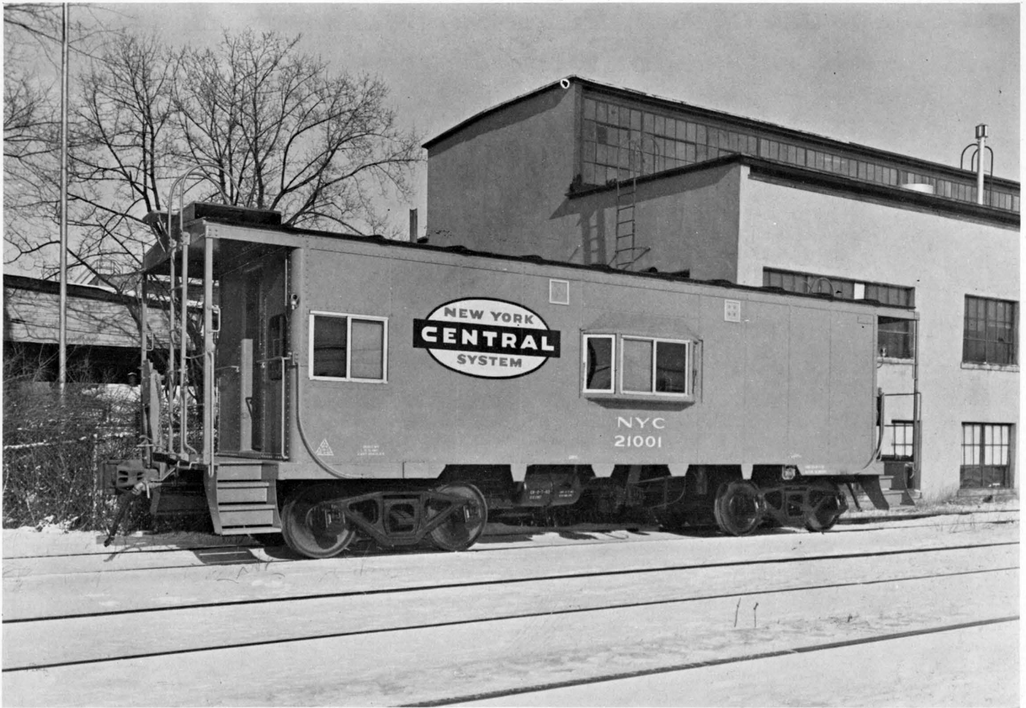
NYC caboose No. 21001, was built by Despatch Shops Inc. in February 1963 as Lot no. 919 which consisted of 100 cabooses (21000 - 21099). Car has green sides and ends, with black roof and underframe. Oval herald size is 6'-6"x 3'-1".
