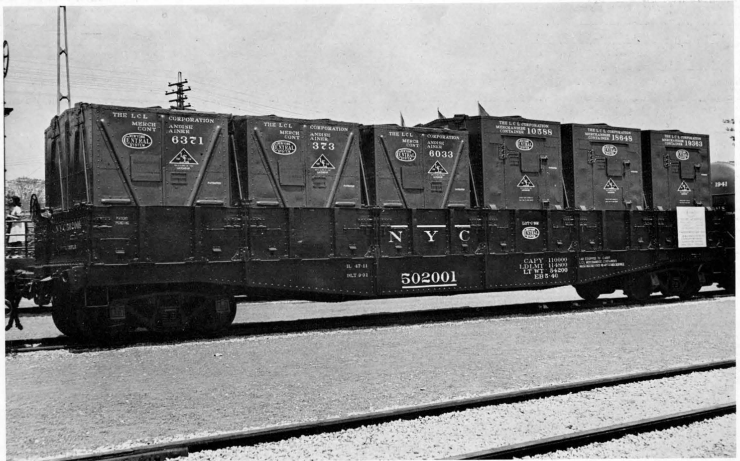
NYC 502001 was a container car from Lot no. C102 and was built in September 1931, it is shown here while on display at the New York World's Fair on June 3, 1940. Oval size was 18"x 9" (V-13532), See page 3, "CENTRAL HEADLIGHT", July 1974. Note the two different sizes of L. C. L. containers and locations of Oval heralds. George E. Votava Collection
