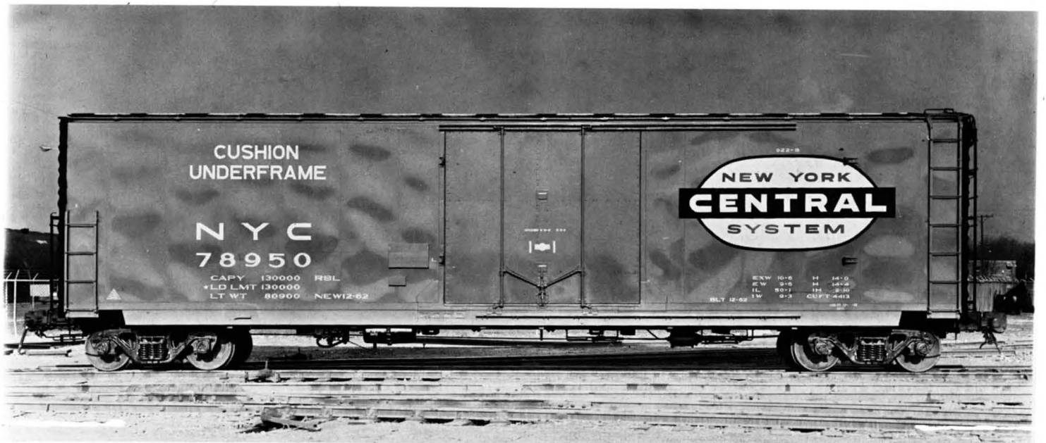
NYC 78950 is a 50'-1" box car from Lot no. 922B, which was built in December 1962. Car has green sides and roof. Body ends and underframe were painted black. Odd shaped "flat top and bottom" Oval herald measured 12'-0" wide.
