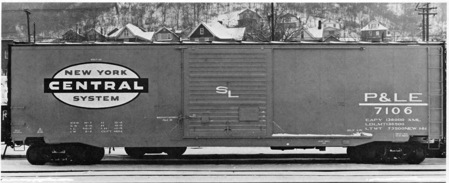
P. & L. E. 7106, a 50'-6" box car, Lot no. 897B, built in January 1961 by Despatch Shops Inc. Green sides, black roof, ends, and underframe. 12'-0"x 5'-4" size Oval herald applied.
