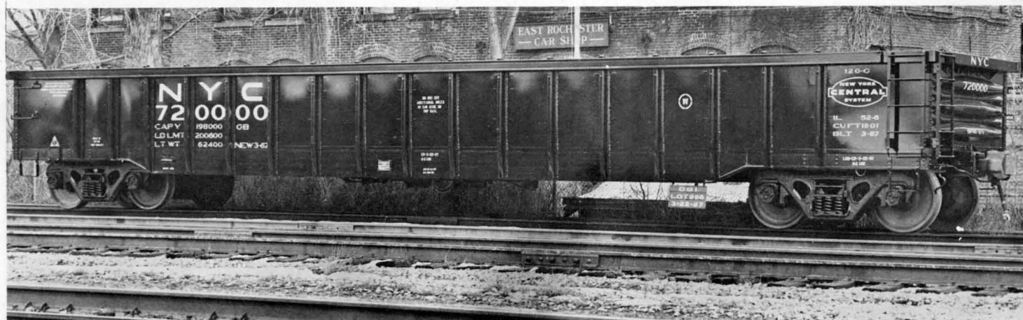
NYC 720000 is a 52' gondola, Lot no. 120G, built by Despatch Shops Inc. in March 1967. Entire car painted black with white "outline only" stencil without bands across oval, it measured 2'-8 1/4"x 14 5/8". (X-59354)
