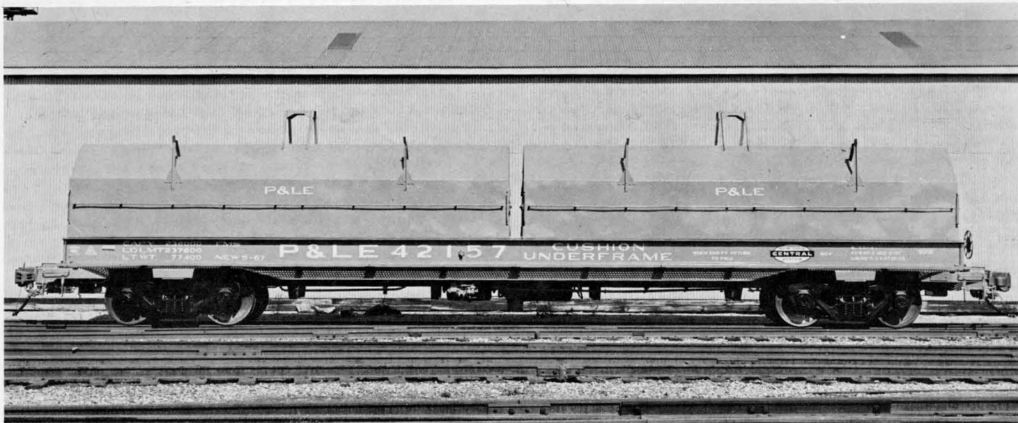
P. & L. E. 42157 is a 125 ton "coil car" from Lot no. 110F built in May 1967. Entire body is green with black trucks. The Oval herald size is 2'-8 1/4"x 14 5/8" (X-58726).
