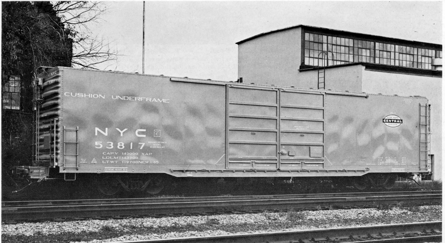
NYC 53817 is a 60' box car, Lot no. 979B, built by Despatch Shops Inc. in November 1965. Entire body is painted green with black underframe and 4'-4"x 23 1/2" herald.
