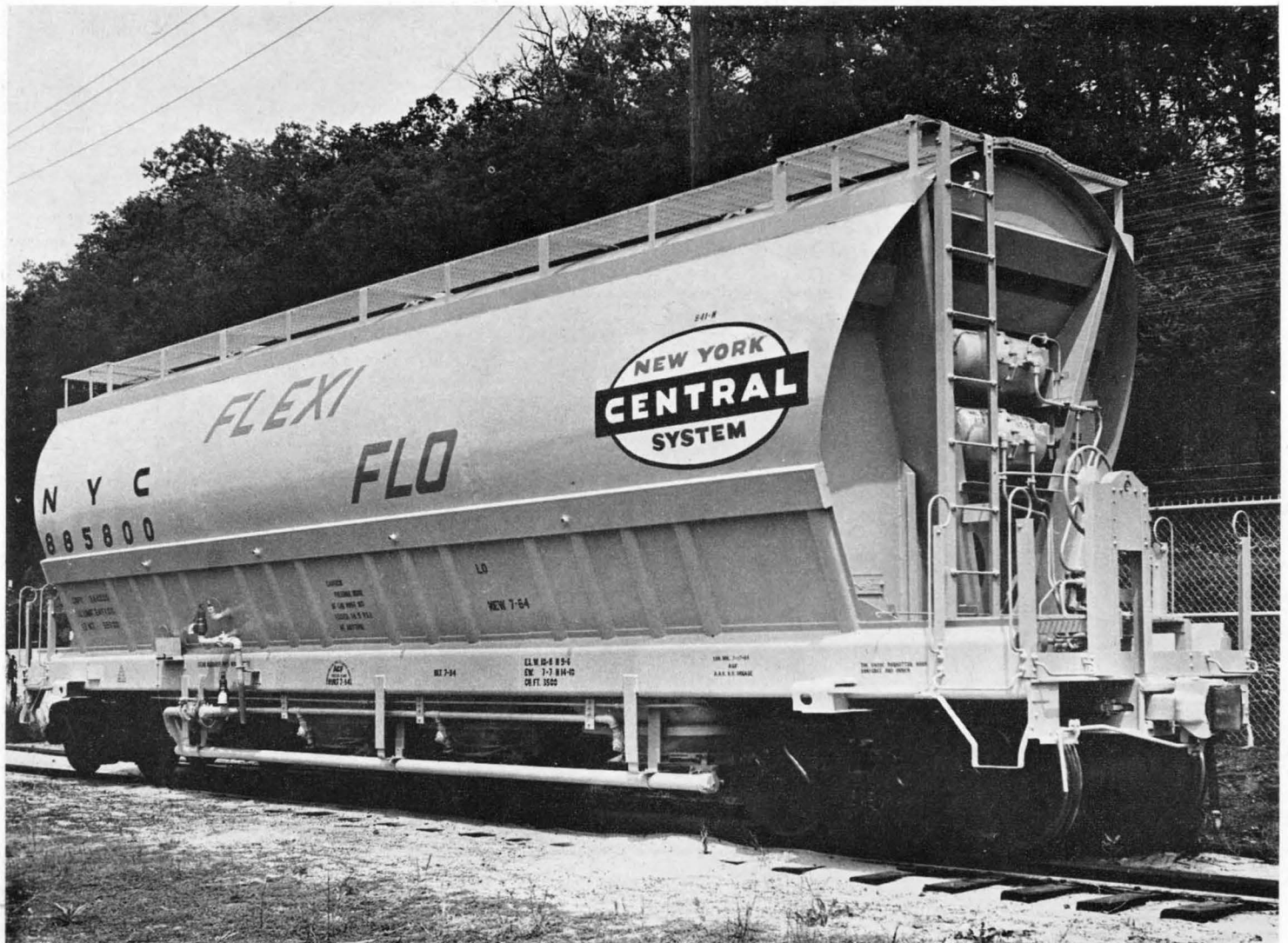
NYC 885800 is a 125 ton "Pressure Discharge" covered hopper, part of Lot no. 941H, built by A. C. F. in July 1964. Car has light gray body with black trucks and a 6'-6"x 3'-1" Oval herald.
