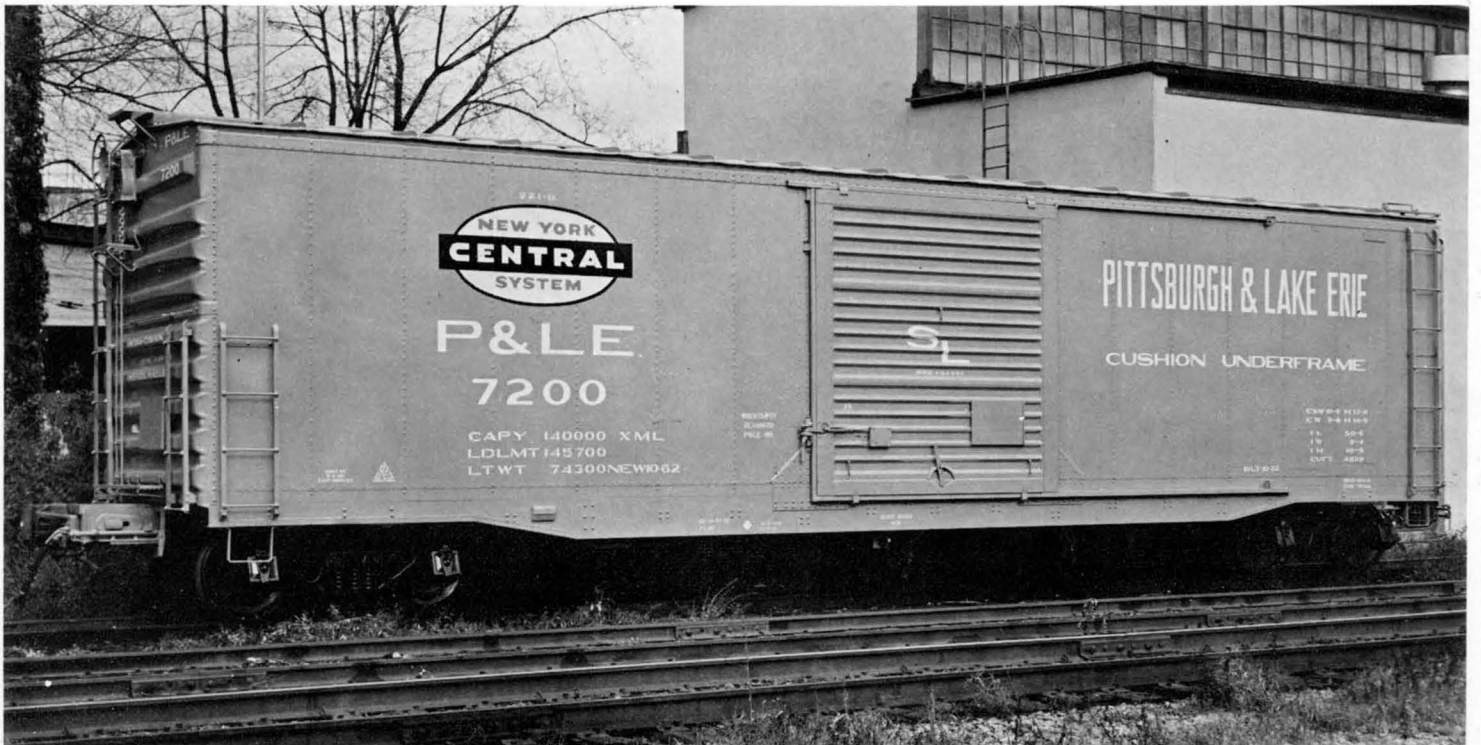
P. & L. E. 7200 is a 50'-6" box car, Lot no. 921B, built by Despatch Shops Inc. in October 1962. Entire body painted green with black underframe. Oval herald size was 6'-6"x 3'-1". This car lot pre dates herald drawing U-58823 and general use of this paint scheme.
