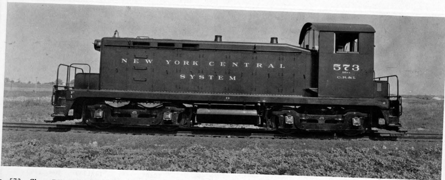
No. 573, Class DEs-4 (Chicago River & Indiana). This E. M. C. model "SC" locomotive was built in July 1936. The 600 hp. switcher was painted gray instead of the usual black and was scrapped in January 1962.
