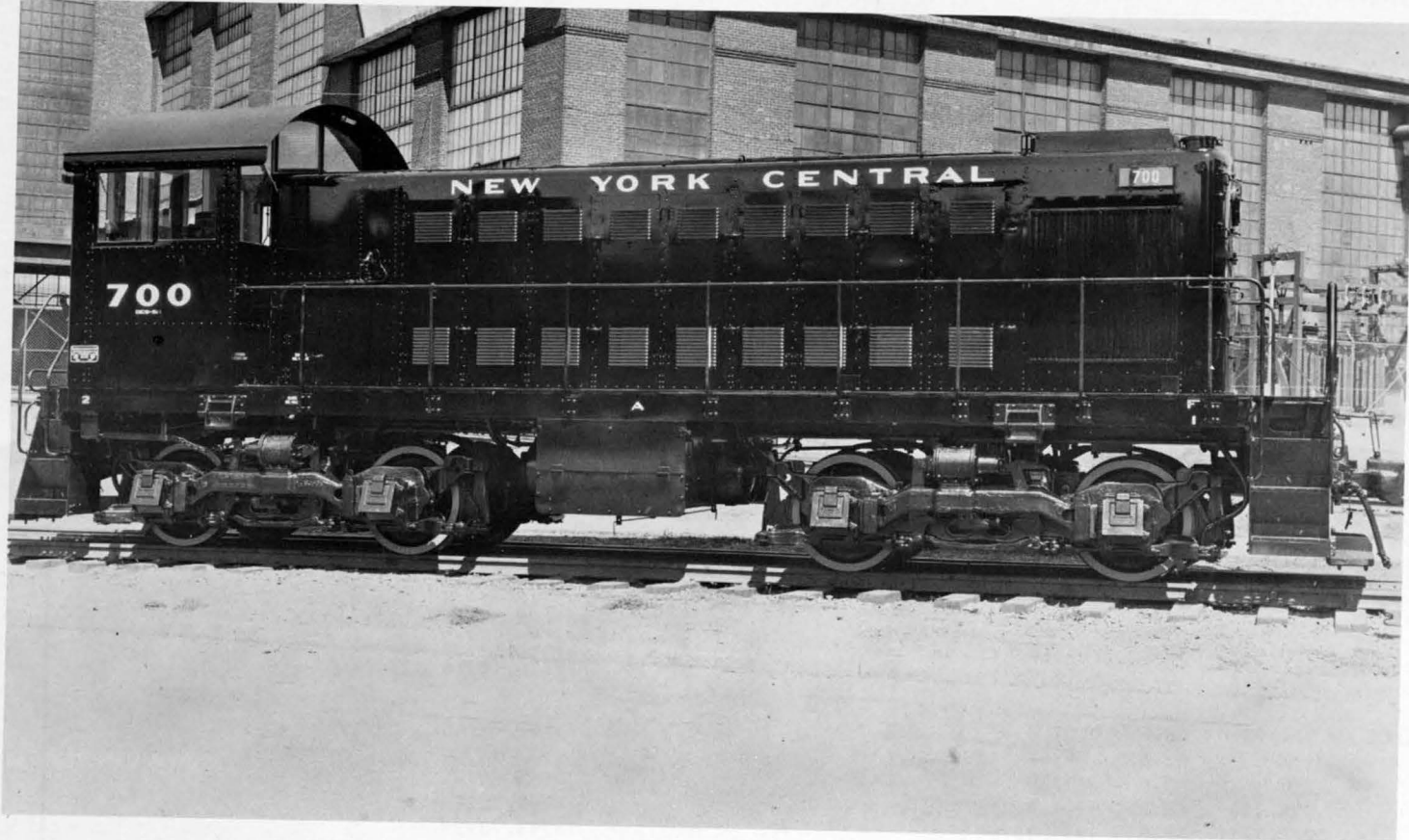
No. 700, Class DES-8b Built by Alco-GE in July 1943 was a 660HP model S-1 switcher. It was renumbered 819 in June 1948 and renumbered again in April 1966 to 9307. Note the older style horizontal radiator shutters.
