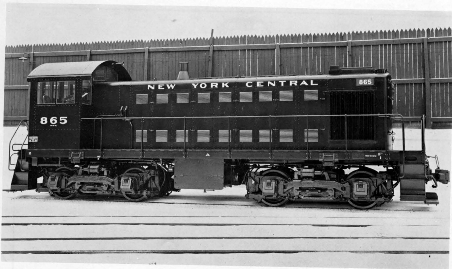
No. 865, Class DES-8d was a model S-1 switcher built by Alco in March 1950 and was renumbered 9341 in March 1966. This 600 hp. locomotive was retired and sold to General Electric in May 1967.
