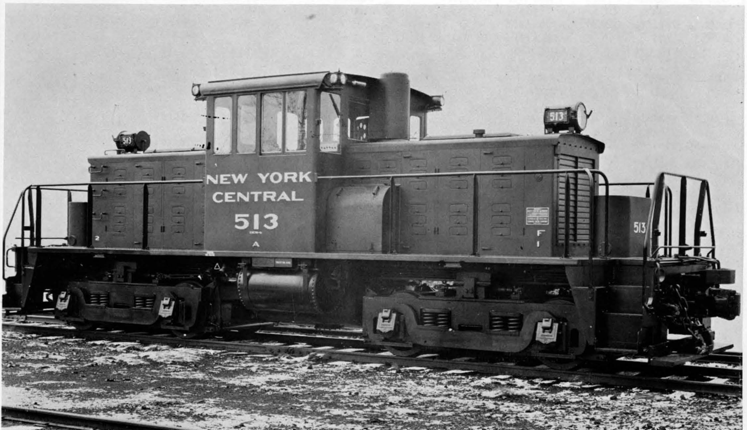
No. 513, Class DES-1c Built by General Electric in November 1942 and powered by two Cummins 6 cylinder diesel engines rated at 165HP each. This 70 ton switcher was withdrawn from service in November 1952 and later sold to Cambria Slag Co. in Sharpville, Pa.
