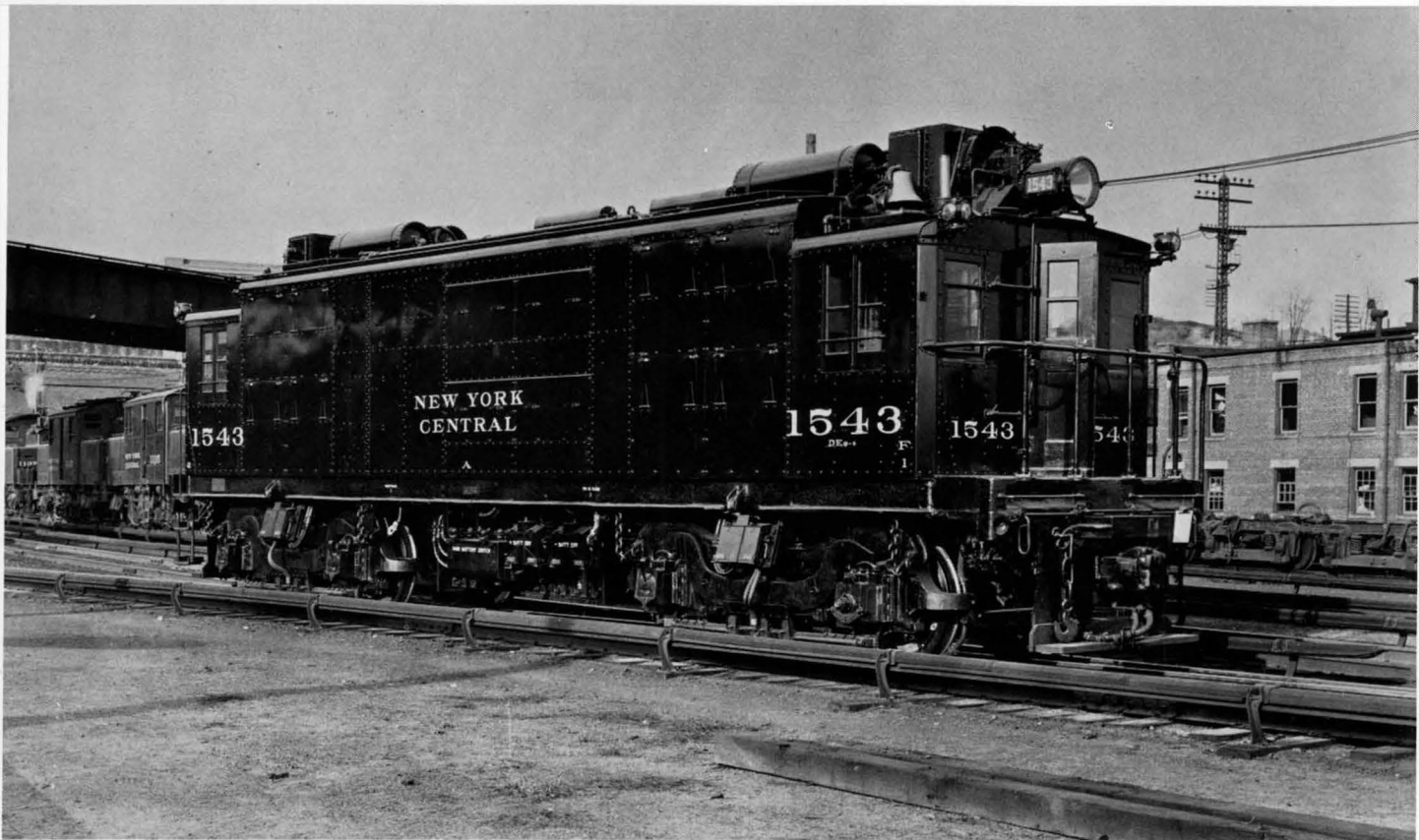
No. 1543, Class DEs-3 Built by Alco-GE-IR in November 1930, this "3 power" locomotive was rated at 300 hp. when used as a diesel-electric and 1665 hp. when used as a "straight" electric. It is shown here shortly after delivery at Harmon, N. Y. It was renumbered 543 in 1936 and withdrawn from service in 1954 and scrapped about a year later.
