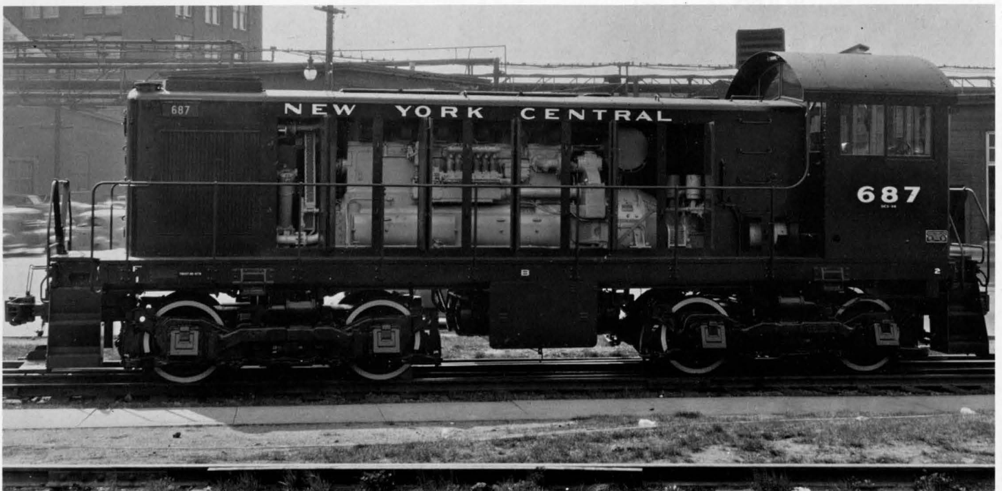
No. 687, Class DES-9b was a model S-1 switcher built by Alco in May 1941, here shown with its hood doors open to display the 660 hp. model 539 engine. This locomotive was renumbered 902 in June 1948, then 952 in July 1950 and finally 9406 in May 1966.
