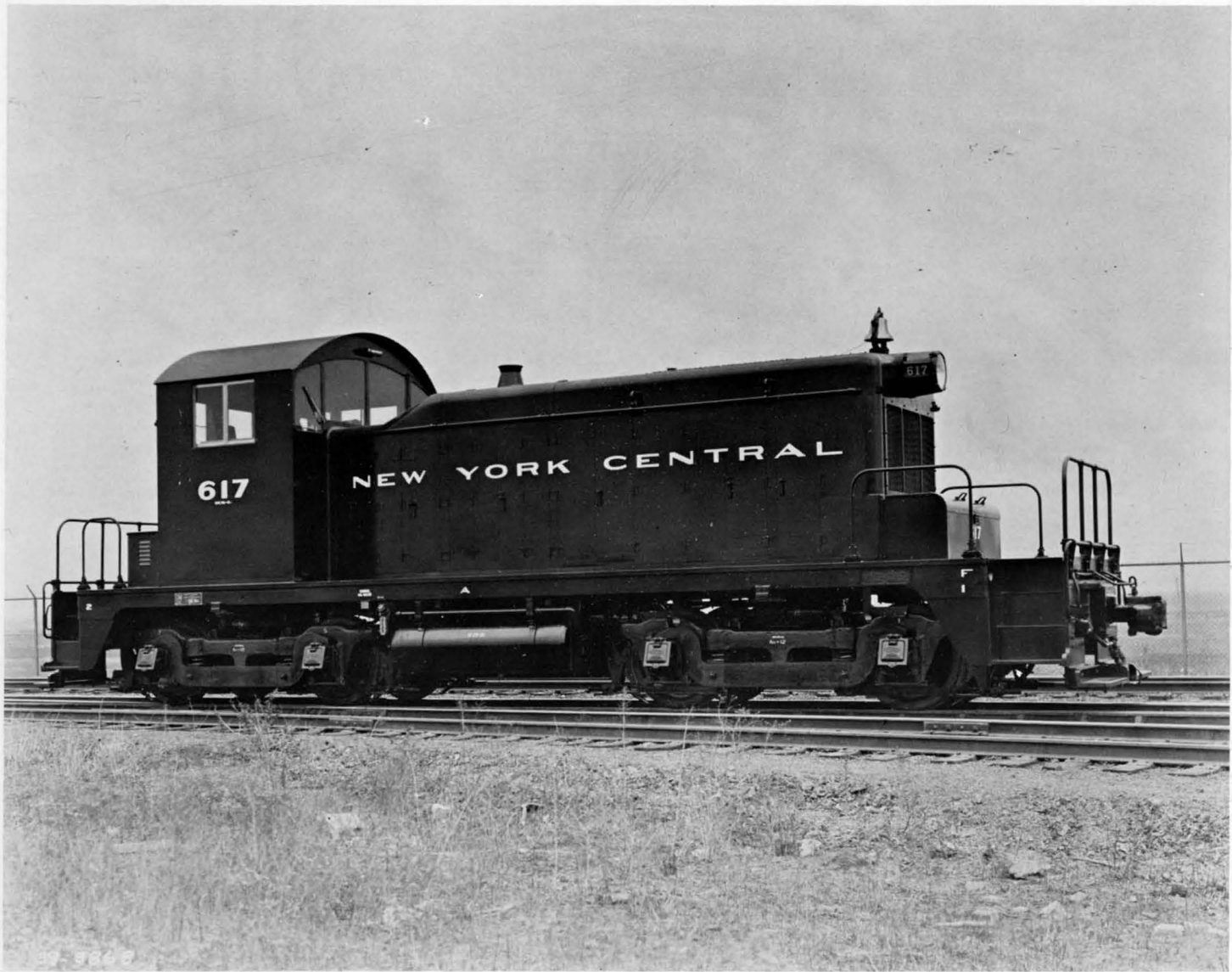
No. 617, Class DES-6c Built by E. M. D. was a SW-1 model locomotive built in December 1939. This 600HP switcher was renumbered 667 in 1949 and was retired in January 1963.
