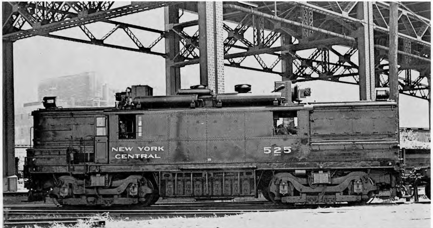
N. Y. C. 525, DES-2 Combination, Diesel-Battery-Electric is shown switching at the 72nd. St. Yard in New York in August 1940. It had been renumbered from it's original number (1525) in 1936 and was rebuilt into Diesel Hump Trailer No. 470 (DHT-2b) in November, 1946 at the Harmon, N. Y. Shops. Diagrams on Pages 12 (original) & 44 (rebuilt).
