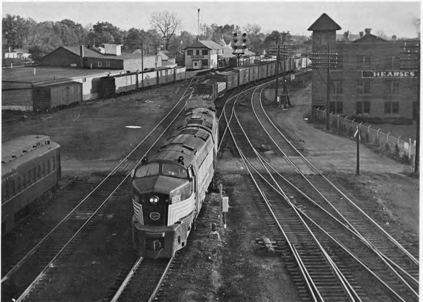
N. Y. C. 3813, DFA-8a leads a "Big Four" (C. C. C. & St. L.) freight through Bellefontaine, Ohio. These Baldwin-Lima-Hamilton RF-16's were used mostly on the old "Big Four" and were noted for their low speed pulling ability on long freight "drags". As with most Baldwins, these RF-16's had their share of nicknames. To "Central" men they were known as "Cabbage Cutters" or "Space Ships"- because of their pointed noses and odd shaped bodies. Diagram on Page 64. Bob Lorenz Collection
