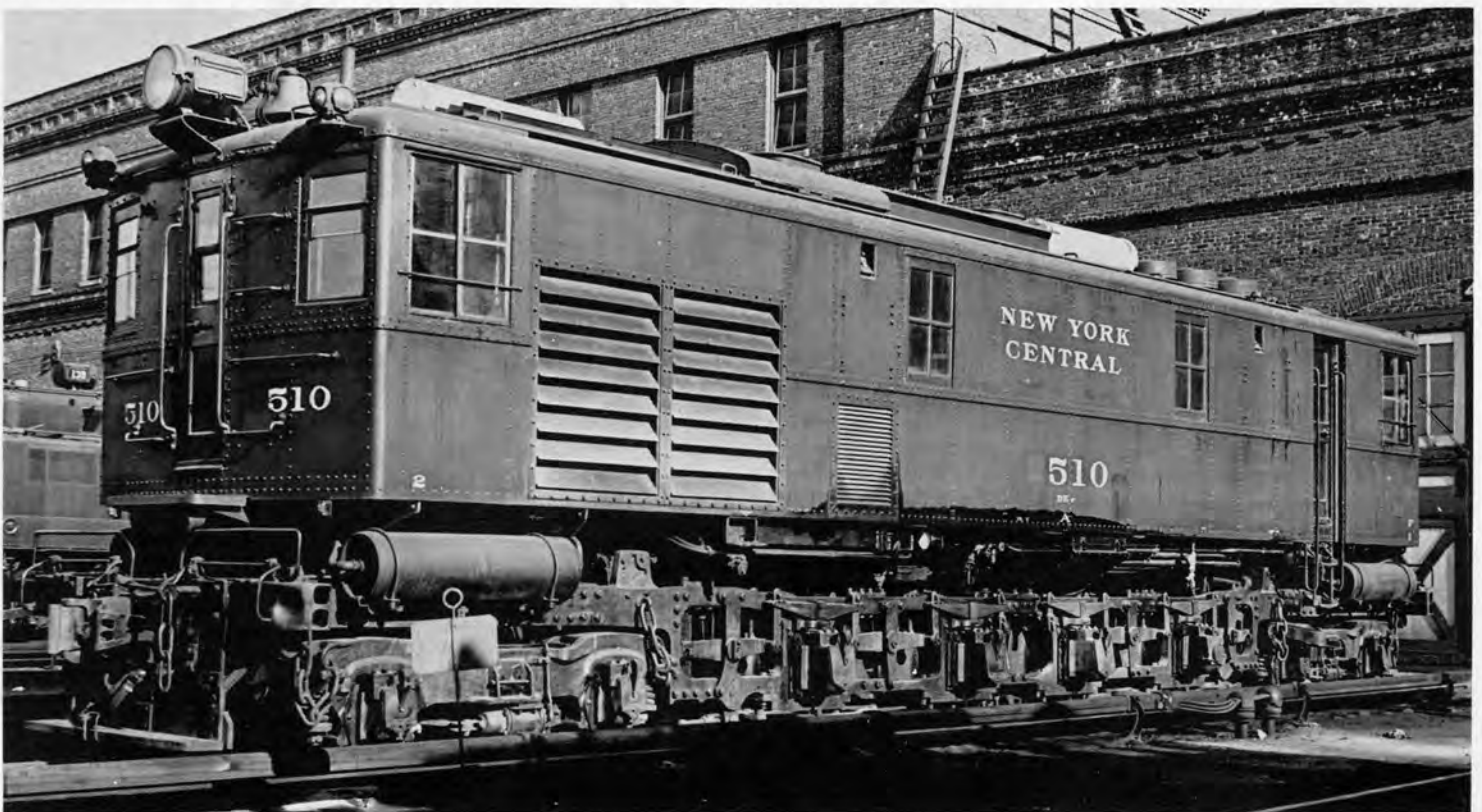
N. Y. C. 510, Def is shown outside the shops at Harmon, N. Y. on May 30, 1938. Its original road number was 1550 when built in June, 1928. See diagram on Page 10. Carbody was later cut down and locomotive was converted to Diesel Hump Trailer 469, DHT-2a. Diagram on Page 44. George E. Votava Collection
