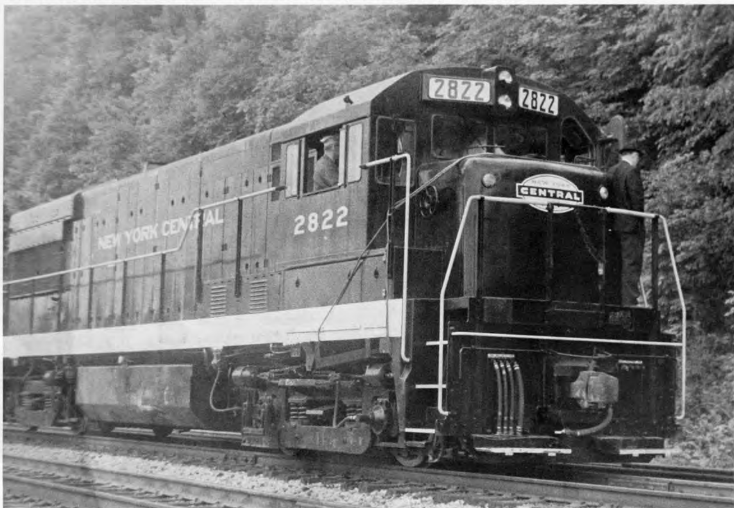
N. Y. C. No. 2822, Class GF-28 was a 2800hp U-28B locomotive built by General Electric in May, 1966 and shown here undergoing service trials. Note that while both locomotives on this page are U-28B's, only the N. Y. C. 2822-2823 have the "conventional" U-28B carbodies. Lighted number boards are now black on a white background and test cables are strung over short hood and lower cab side.
