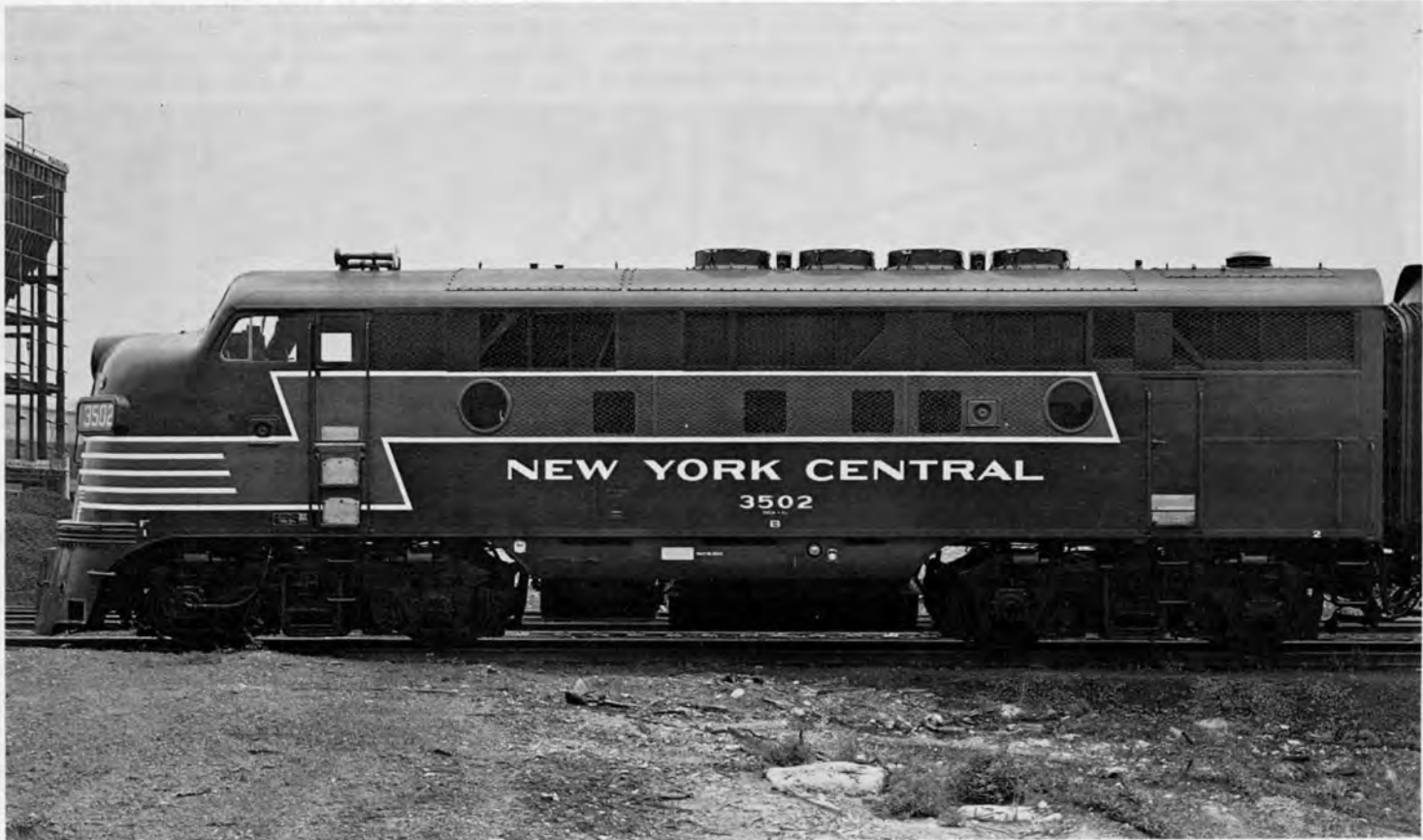
N. Y. C. 3502, DCA-1a clearly shows the lack of a dynamic brake fan on the hatch behind the cab. Instead, water for the steam generator was carried in tank attached to the inside of the hatch roof. Color is two tone gray with black trucks. 3502 was sold to EMD in 1961 without being renumbered as were sister units. Diagram on Page 68.
