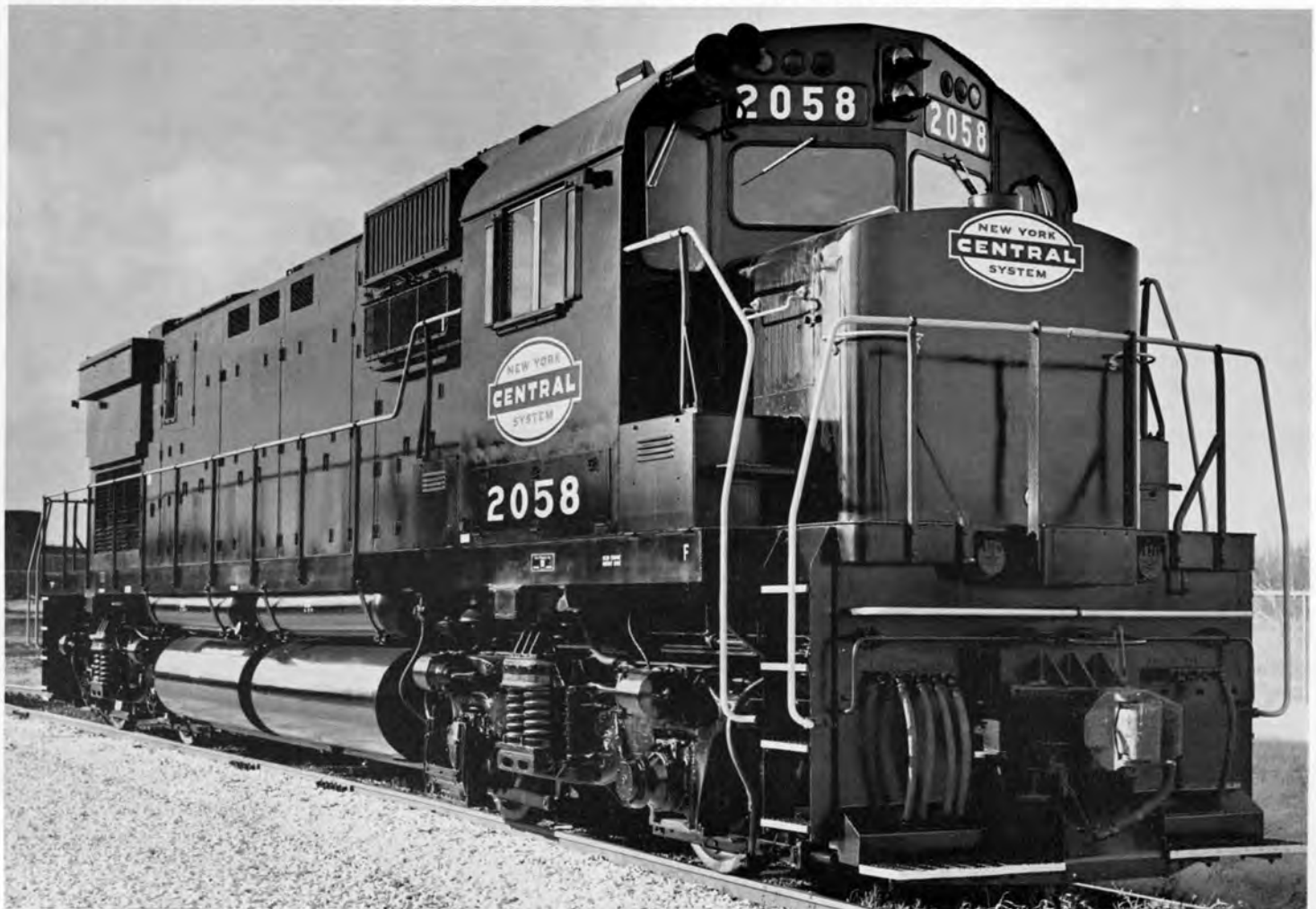
N. Y. C. No. 2058, Class AF-30 was a 3000hp Alco C-430 "Century" locomotive built in November, 1967. Besides the lack of "New York Central" lettering on the long hood, the usual wide white stripe along the frame side sills has not been applied to this last series of locomotives acquired by the New York Central System.
