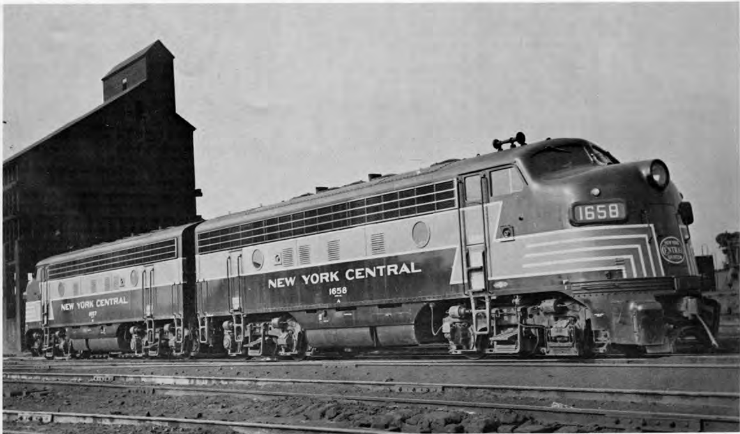
N. Y. C. 1657 & 1658, DFA-2d wait for a call to service on an engine terminal ready track. Note that the enclosed pilot coupler doors have been left open. In later years these doors were removed and a metal plate welded in the resulting open area. Notice that grab irons have not yet been applied to nose and cab roof above windshield. Diagram on Page 50. Paul W. Prescott Collection
