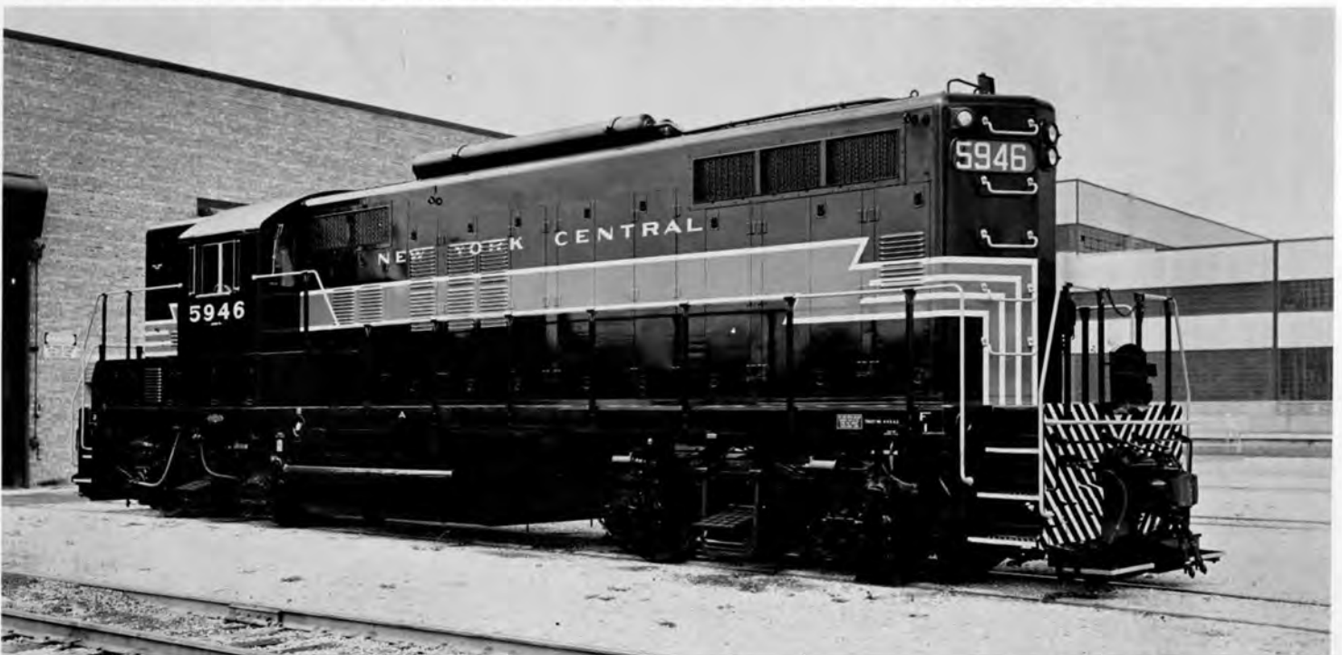
Back from the dead! N. Y. C. 5946, DRSP-9c was severely wrecked at Wellington, Ohio in 1960. It was returned to EMD for rebuilding and emerged as shown here WITHOUT steam generator equipment and reclassified DRS-9c for freight service only. Body color is black as compared with "before" photo of same locomotive on page 97 which was dark gray.
