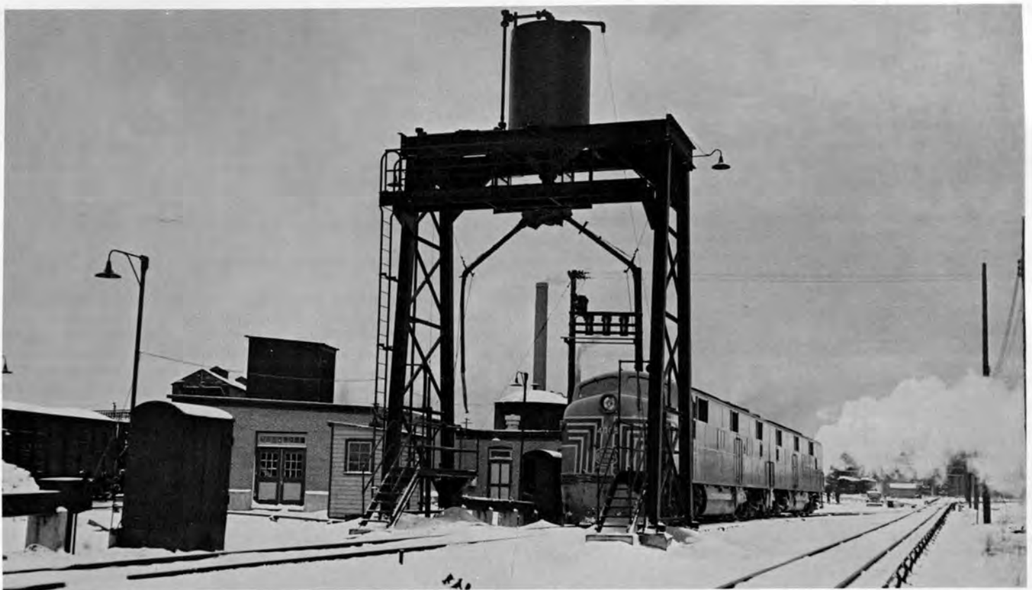
N. Y. C. 4005, DPA-1a and an unidentified EMD E-7 "B" unit ease up into the sand tower at Harmon, N. Y. on March, 3, 1947 through a carpet of snow. Note the steam behind the "B" unit. This was done deliberately during cold weather as it was necessary to "crack" the steam heating train line valves when not in use to keep them from freezing up solid when not connected. Diagram on Page 70.
