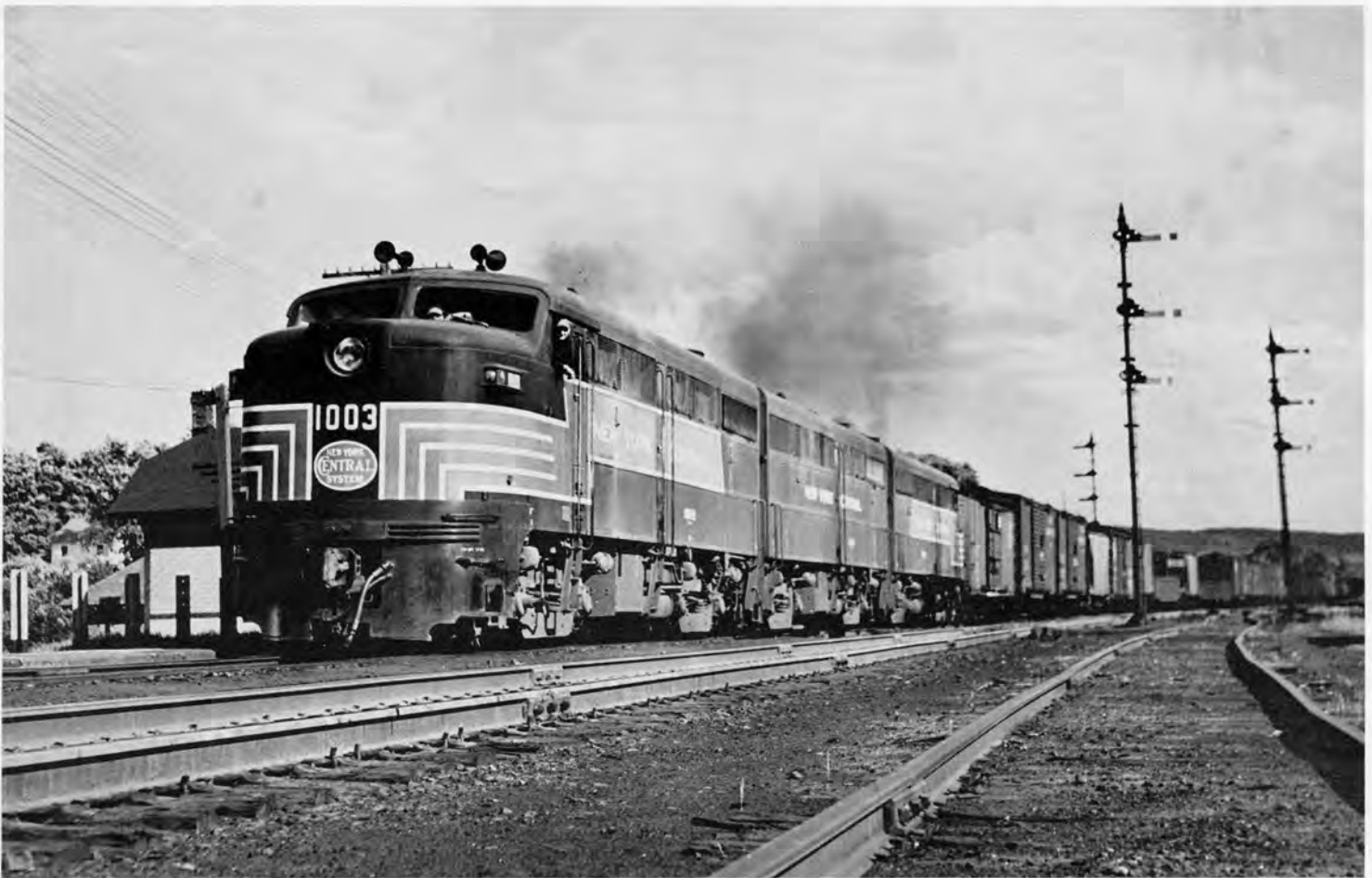
N. Y. C. Alco FA-1 1003, DFA-3a highballs through Hinsdale, Mass. on the Boston & Albany with a freight train in 1948. Typical of most Alcos is the plume of black smoke seen when the engine throttles were opened up. 1003 was traded in to General Electric in January, 1964 for U-25B credit. Diagram on Page 52. Bob Lorenz Collection
