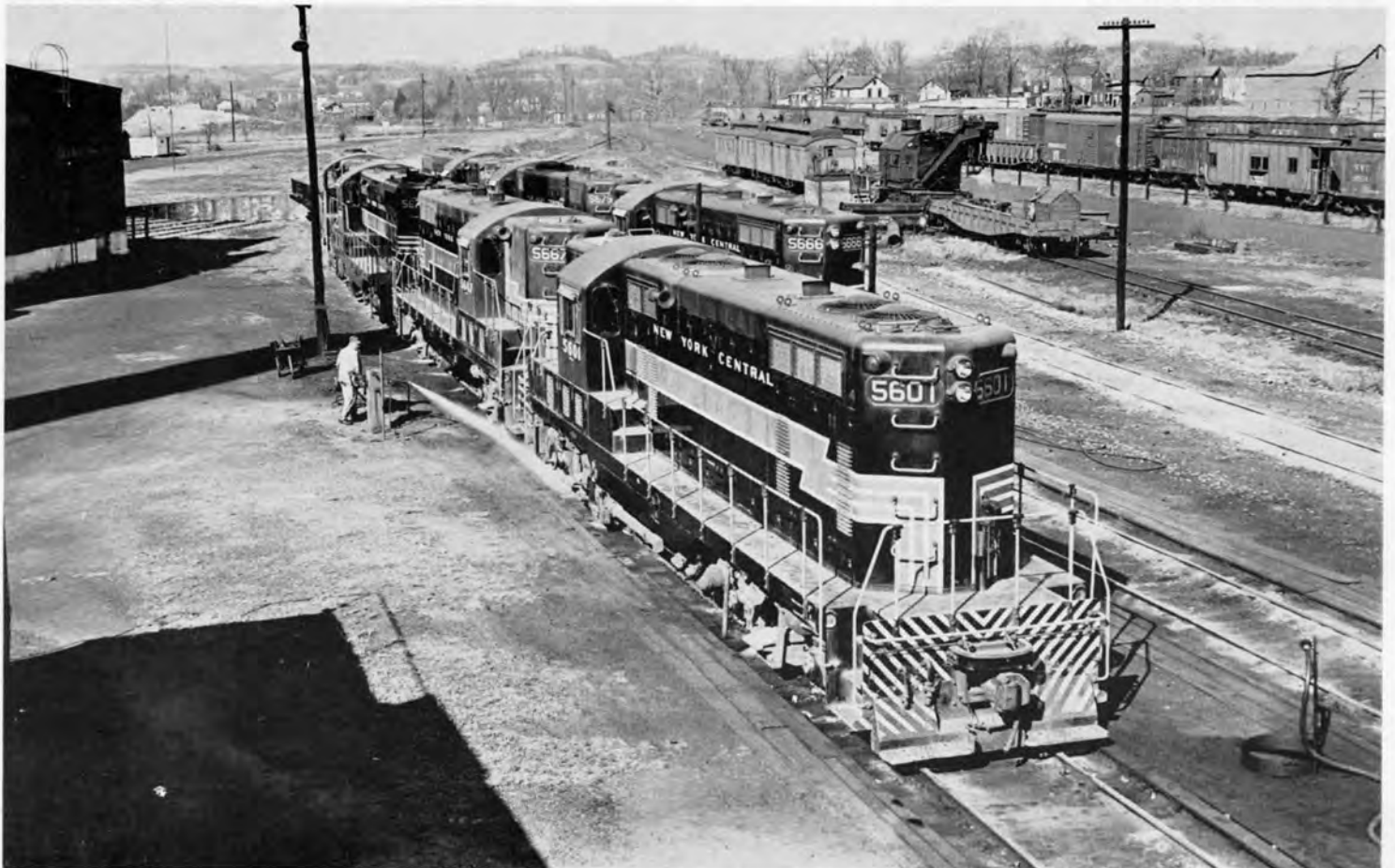
Interesting line up of GP-7 motive power on the ready track awaiting mine run assignments at Minerva, Ohio. Note that 5601, DRS-4a has not yet been equipped with M. U. controls on the # 1 end. Diagram on page 84.
