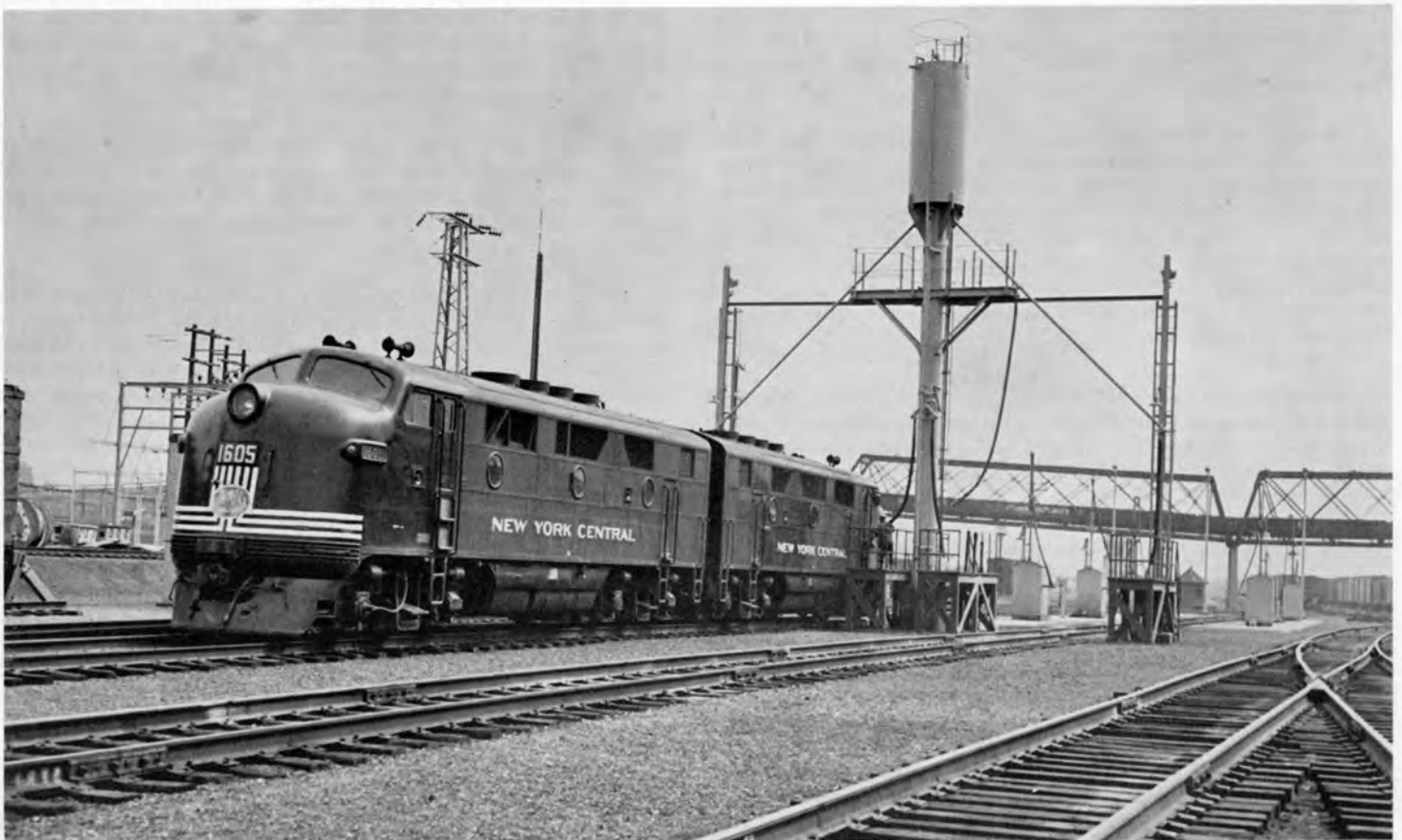
N. Y. C. 1605 & 1604, DFA-1b pause at the service track at Dewitt, N. Y. on August 24, 1949 as 1604 gets one of its four sand boxes filled. Note early style paint scheme and lack of painted road number under road name lettering on sides of locomotive. Diagram on Page 48.
