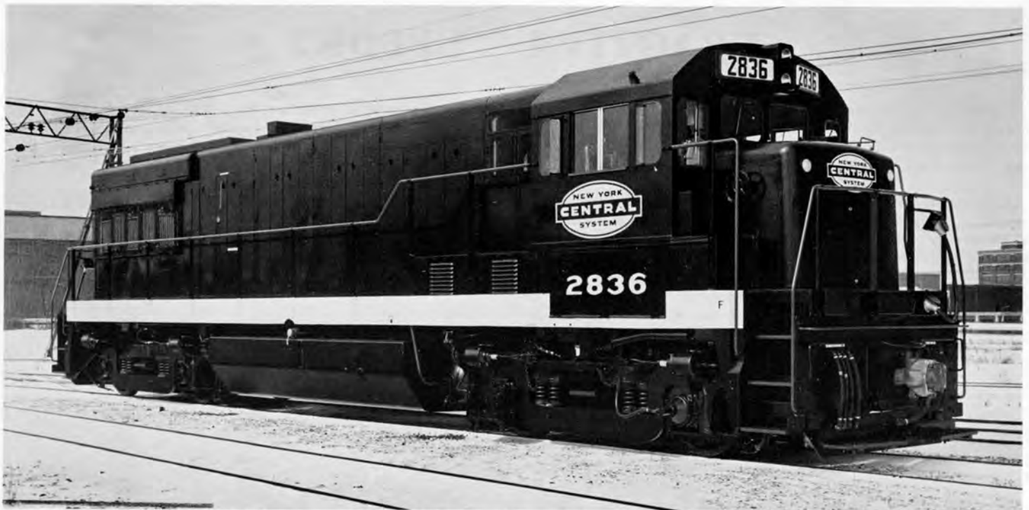
N. Y. C. No. 2836, Class GF-30 was a 3000hp U-30B locomotive built by General Electric in January, 1967. Locomotives 2830-2839 were built using "trade in" trucks from Fairbanks-Morse DFT-1 locomotives, (see diagram on page 78) with a wheelbase of 9' - 6". After the P. C. merger, the F. M. trucks were replaced with the standard 9' - 4" wheelbase Alco trucks because the odd axle size of the older trucks ment too much "down" time in the shops waiting for wheels. Note lettering "New York Central" no longer on side of long hood, but new style herald appears on side of cab.
