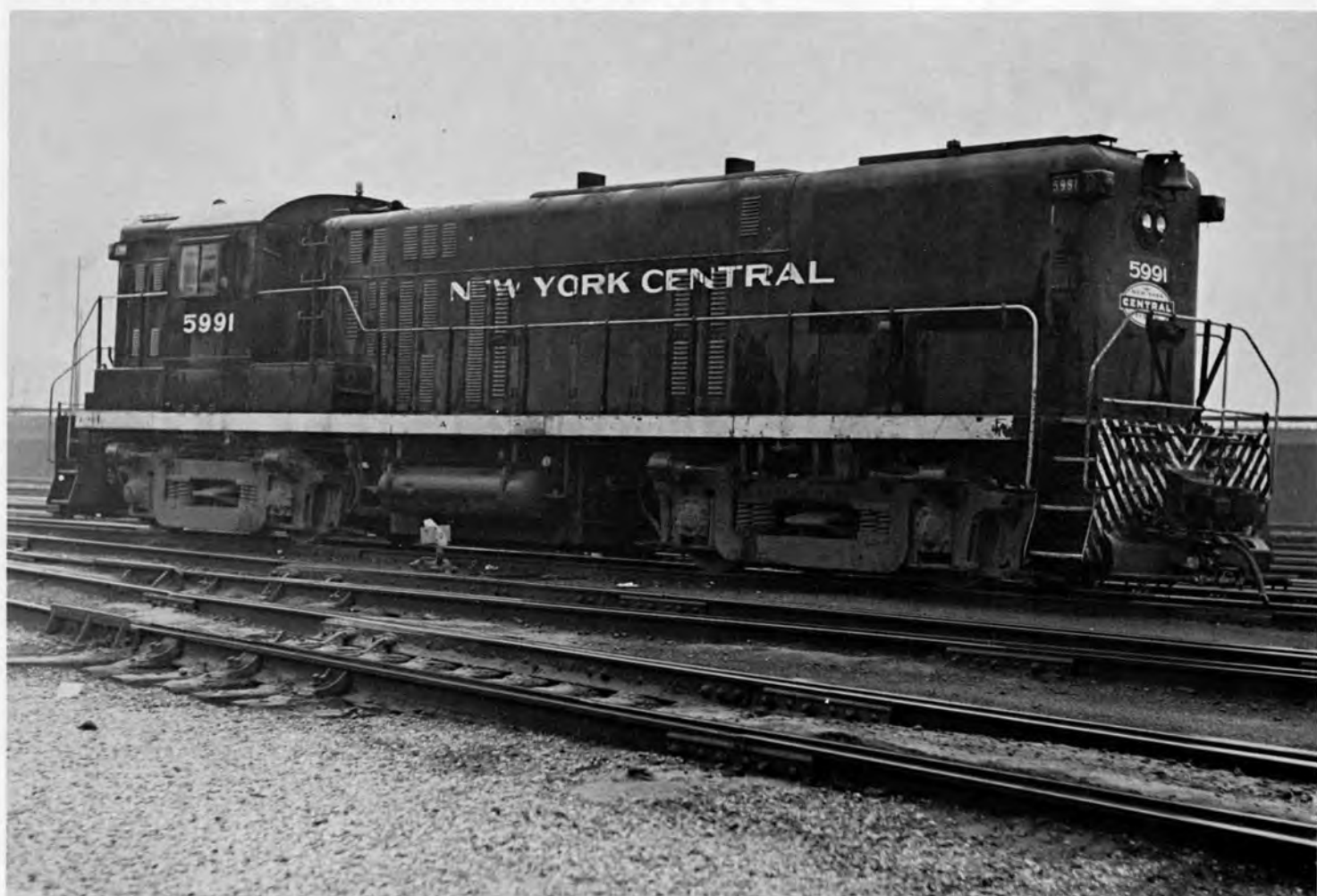
N. Y. C. 5991, DRSP-3a as it appeared in Chicago, Ill. on April 23, 1966. This road switcher was numbered 7301 prior to 1966 and was retired in August, 1967. Compare this more modern paint scheme with the two tone gray that appears in the photo of 7300 on page 83. Note the bay window addition to the cab side window. Jim Claflin Collection
