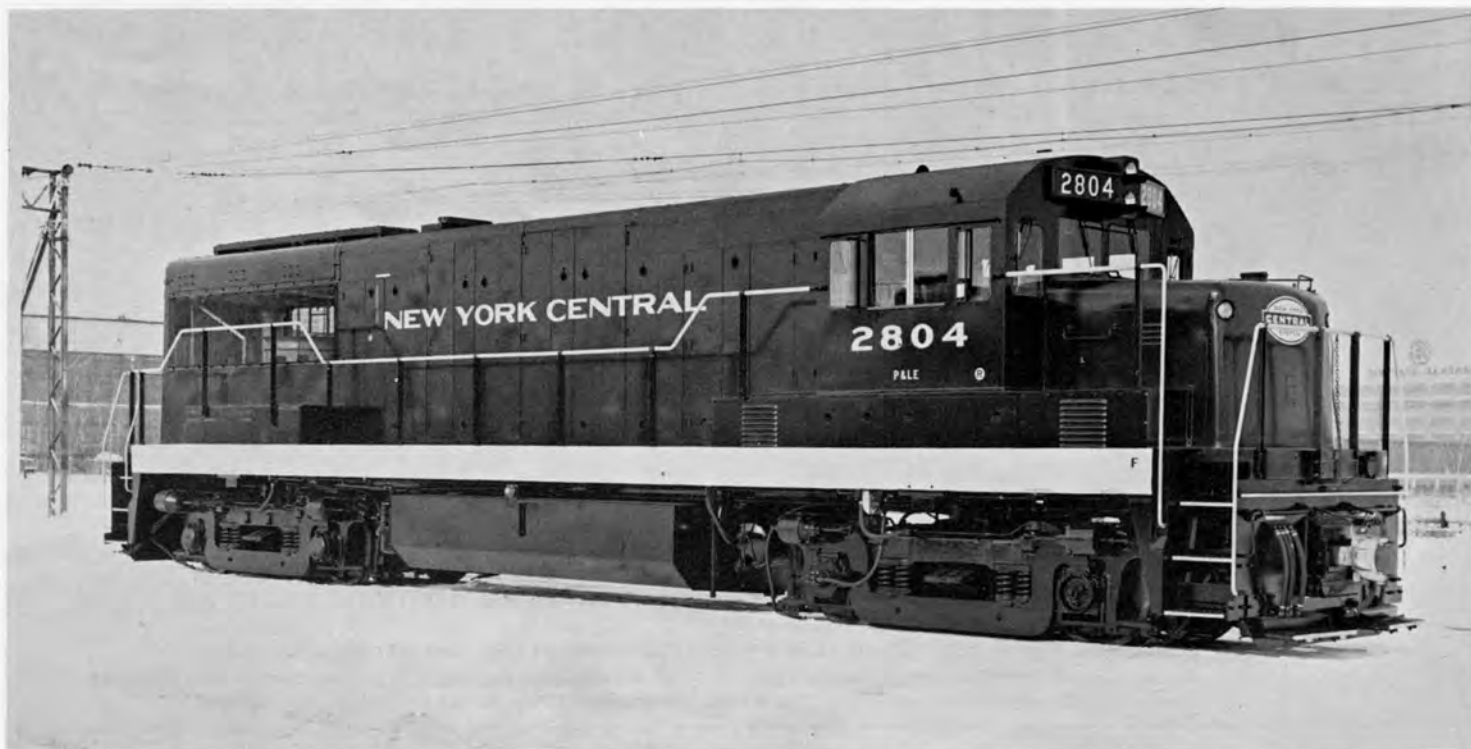
P. & L. E. No. 2804, Class DRS-17a was a 2800hp U-28B locomotive built by General Electric in February, 1966. The carbody for this series of locomotives was actually an earlier U-25B type (P. & L. E. 2800-2821), but all internal equipment was "U-28". This series of G. E. locos were the only ones without dynamic brakes.
