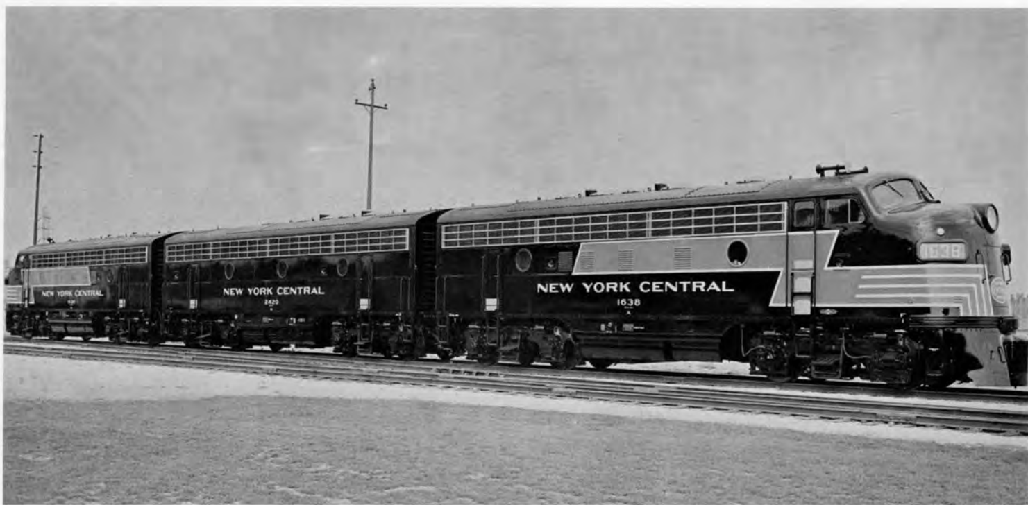
N. Y. C. 1636 & 1638, DFA-2c along with 2420, DFB-2c show the first version of the gray "lightning stripe" paint scheme (circa 1949) which did not extend the entire length of the "A" units. The "B" units were solid black with only white lettering for a contrast. Passenger units did not use this "abbreviated" scheme which was later extended along the middle strip of all A and B units on the N. Y. C.
