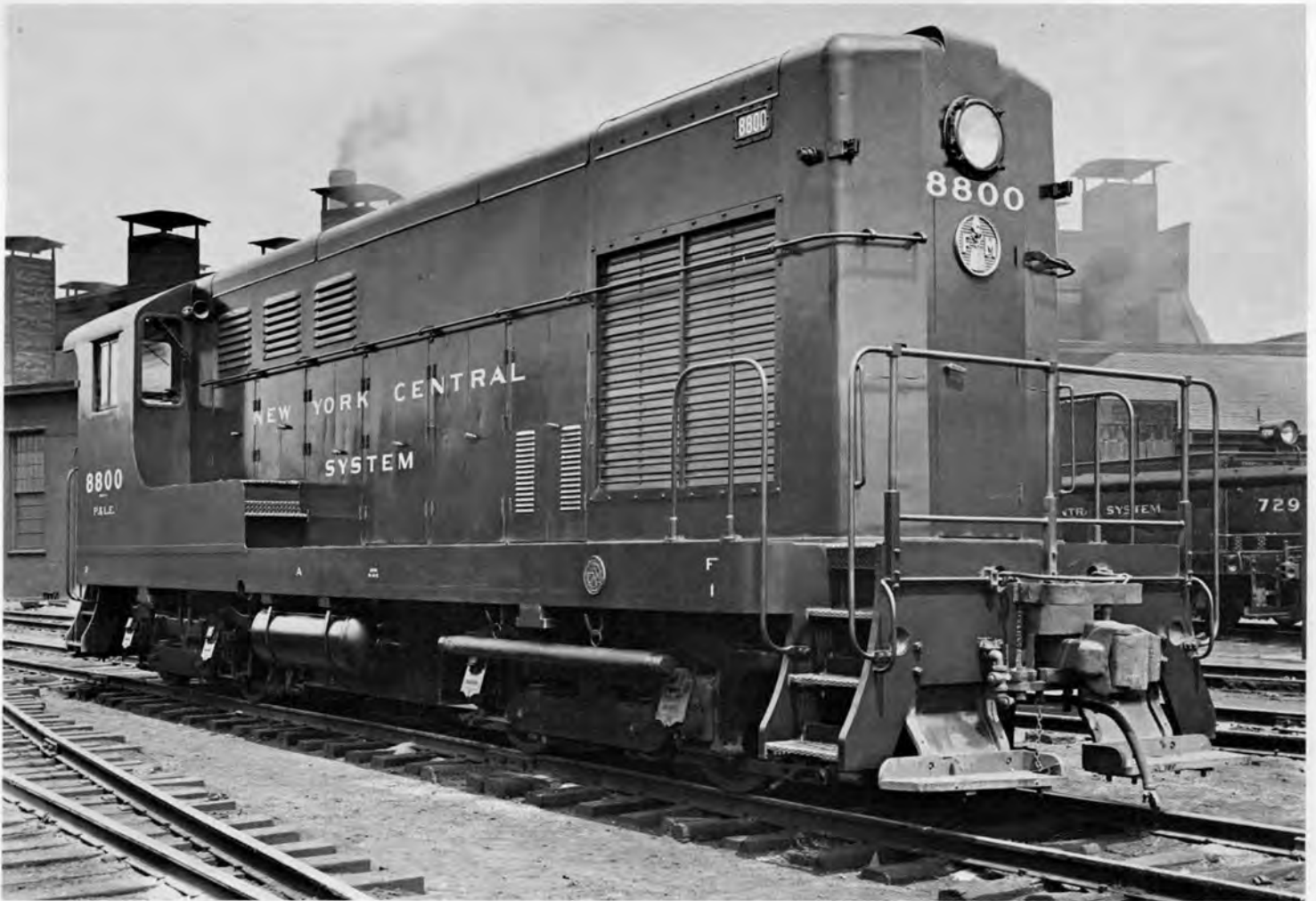
P. & L.E. 8800, DES-14a shortly after delivery in 1946. There were four Fairbanks-Morse diesel switchers on the Pittsburgh & Lake Erie, all of them were sold to the N.Y.C. in February, 1950. Carbody color is "Pacemaker" green with black trucks and underbody. Lettering is white. Handrails & grab irons are not yet painted yellow and no 2" wide stripes appear on the pilot plate. Diagram on page 32.
