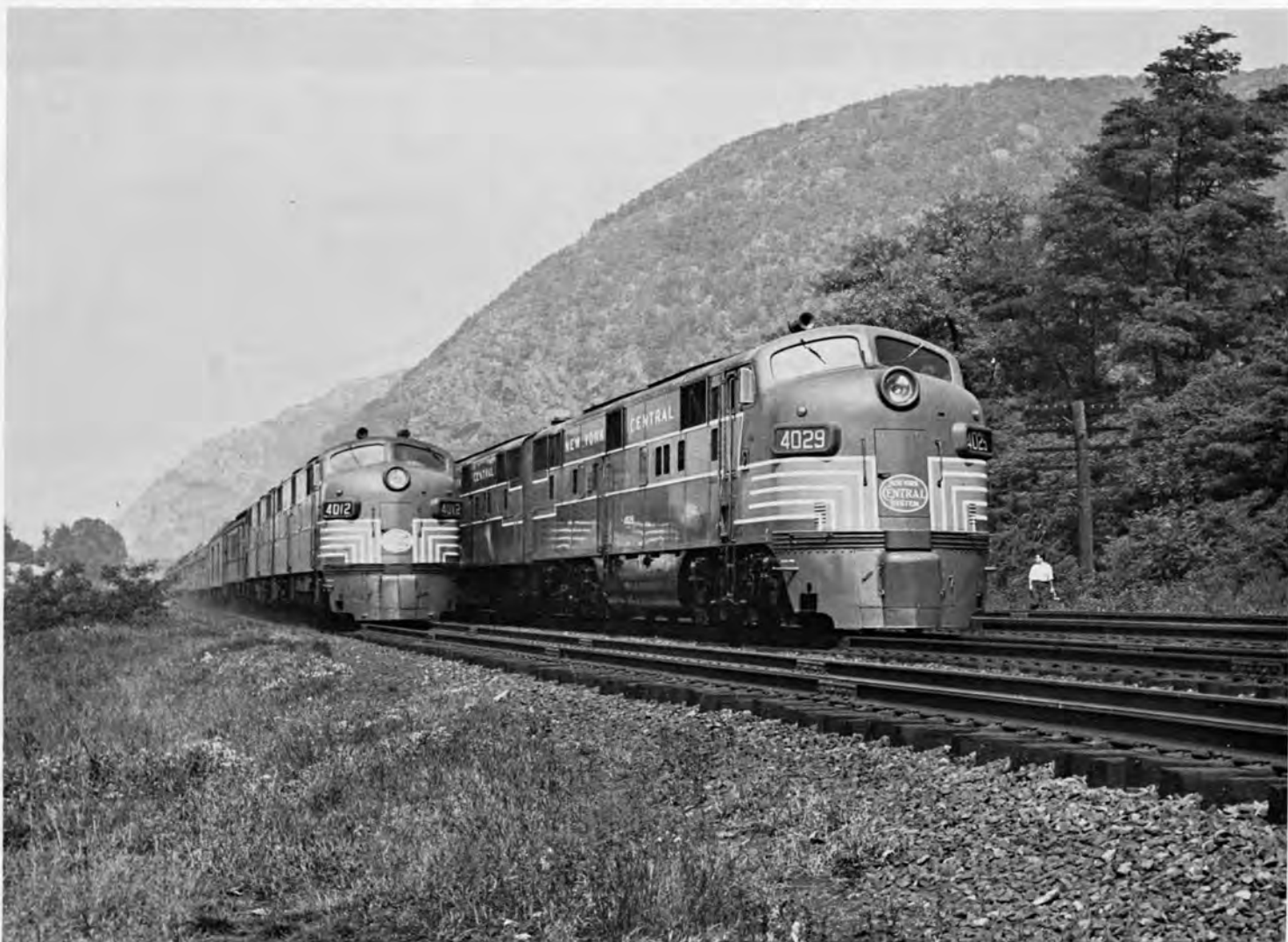
N. Y. C. 4012, DPA-1b & 4029, DPA-1c head westbound passenger trains at Cold Spring, N. Y. about 1948. Note that front pilot enclosed coupler doors are still in place and upper nose and windshield grab irons have not been added.
