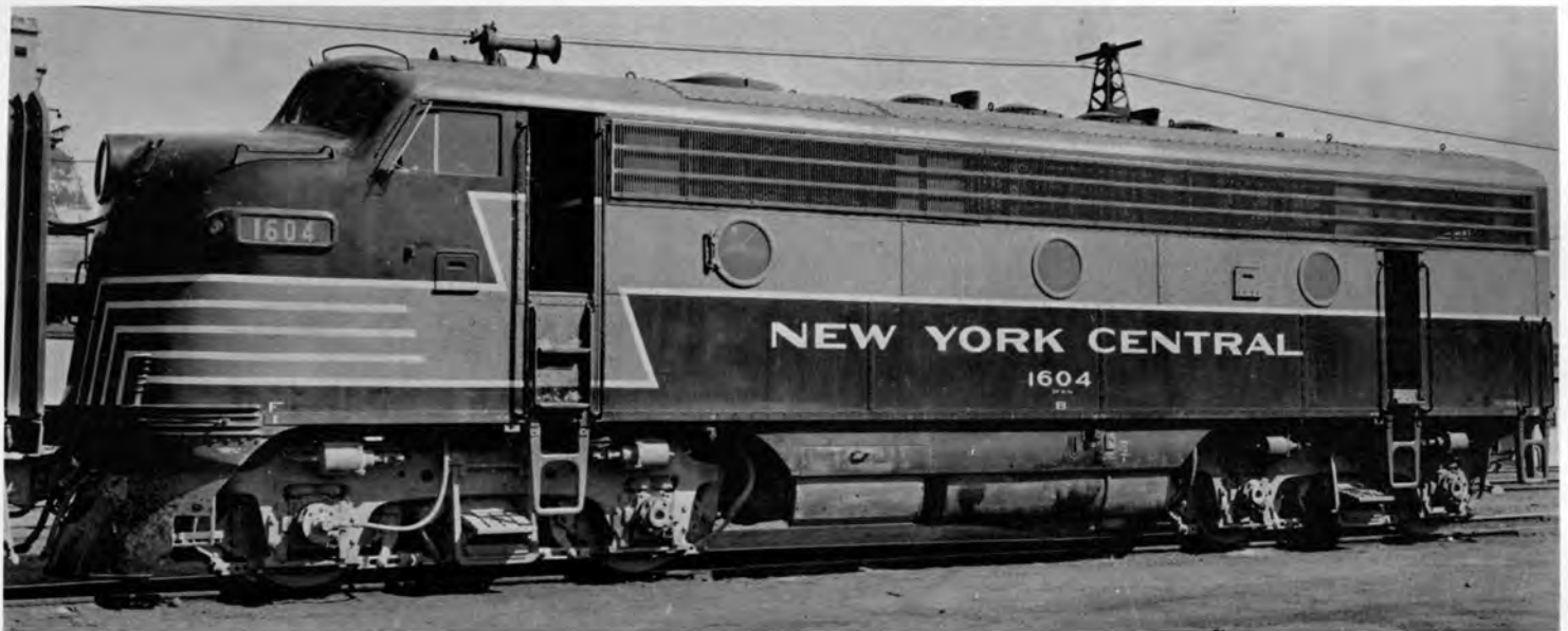
N. Y. C. 1604, DFA-1b as it appeared on July 31, 1960. If you compare this view with the photo of "sister" locomotive 1605 on page 49, you will notice a number of modifications. Stainless steel grilles have been applied over radiator intake openings instead of the original wire mesh, all roof mounted fans, including the dynamic brake fan, have been replaced later style types. Extra grab irons have been added to the front end as well as front end M. U. electrical controls which can be seen by the cable below the headlight extending to the unit in front of the 1604. This locomotive was traded in to EMD in December, 1965. Diagram on Page 48. Paul W. Prescott Collection.
