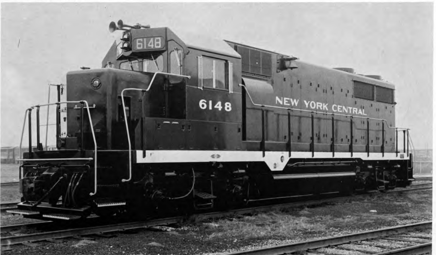
N. Y. C. No. 6148, Class DRS-14C was a 2500hp GP-35 locomotive built by E. M. D. in January, 1965. It was renumbered to 2392 and reclassified EF-25 in 1966. Note that last style N. Y. C. herald is not yet been applied to short hood.
