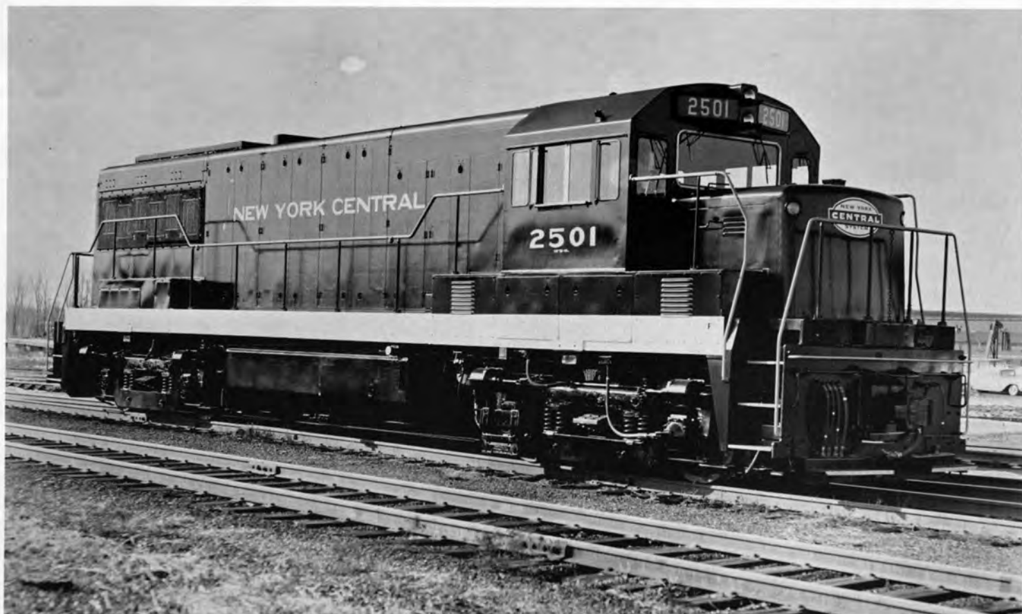
N. Y. C. No. 2501, Class DRS-15A was a 2500hp U-25B locomotive built by General Electric in January, 1964. It was later reclassified GF-25 in 1966 while retaining the same road number.
