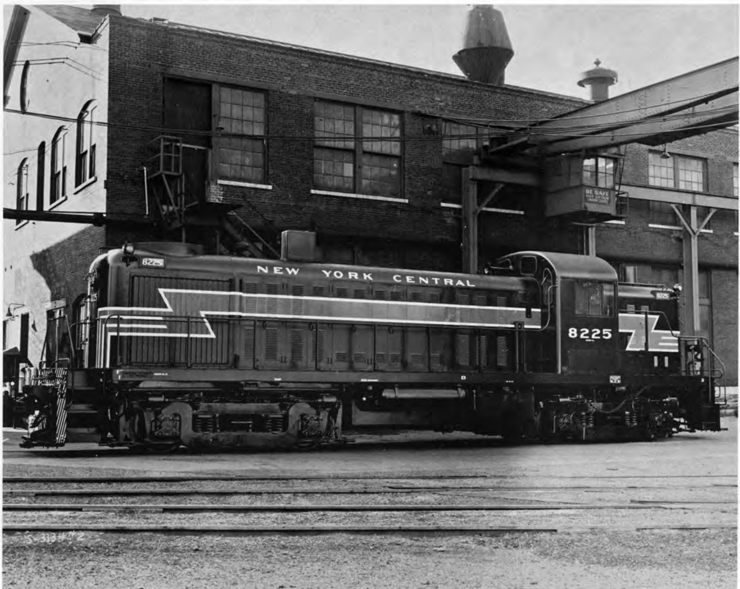
N. Y. C. No. 8225, Class DRSP-6A was a 1600hp RS-3 locomotive built by Alco in August, 1950. It was later reclassified to DRS-6A with the removal of steam generator equipment and was sold to General Electric in September, 1965.
