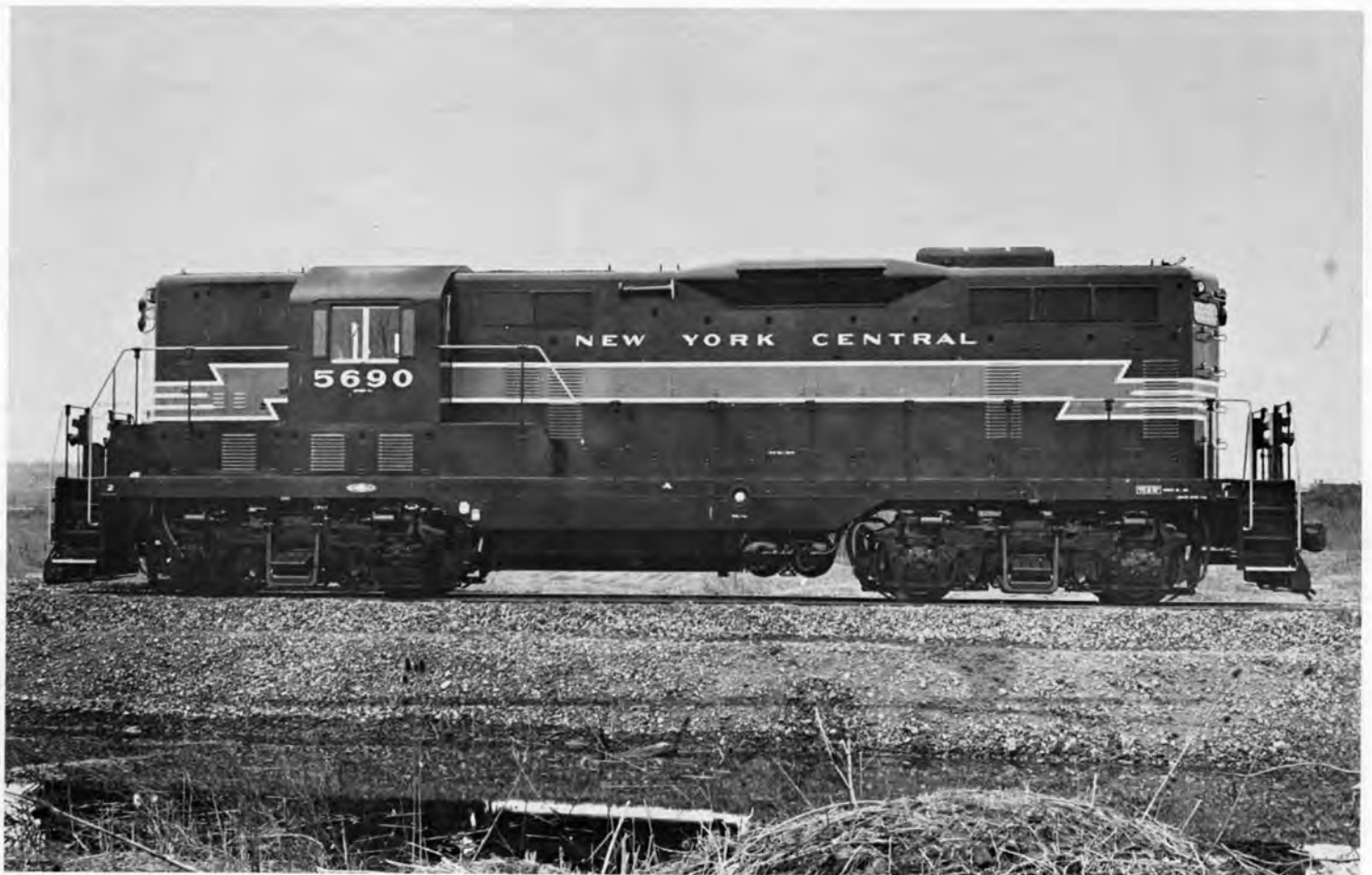
N. Y. C. No. 5690, Class DRS-4H was a 1500hp GP-7 locomotive built by E. M. D. in March, 1952 and was reclassified to ERS-15 in 1966. Note that these locomotives, (DRS-4H) are equipped with both dynamic brakes and hood winterizer hatches.
