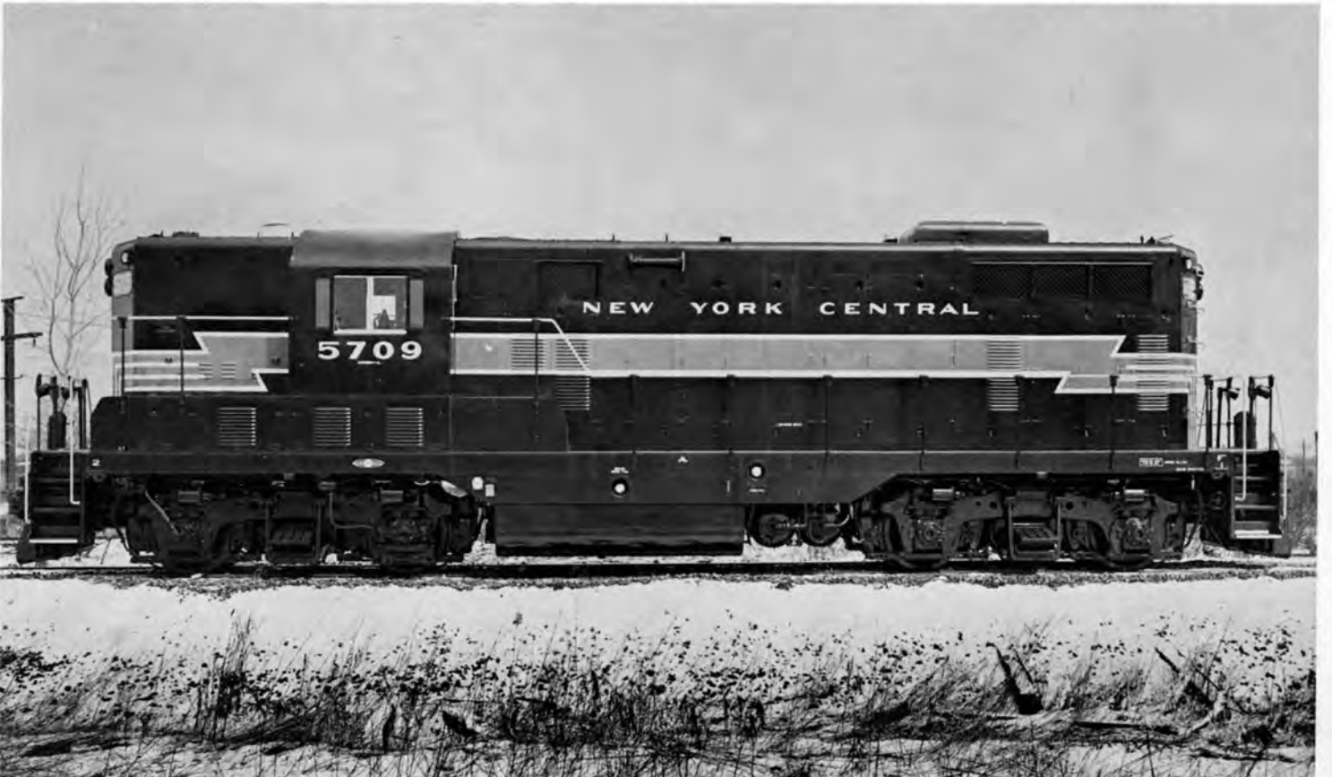
N. Y. C. No. 5709, Class DRSP-4J was a 1500hp GP-7 locomotive built by E. M. D. in March, 1952. It was reclassified to DRS-4J when its steam generator was removed prior to freight service. It was again reclassified in 1966 to ERS-15 in 1966. Note hood winterizer hatch used.
