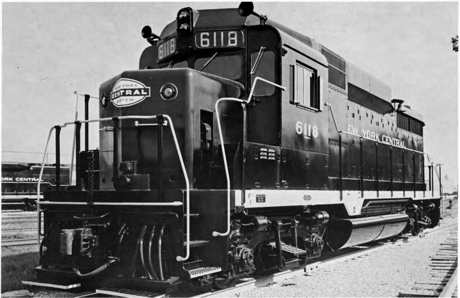
N. Y. C. No. 6118, Class DRS-13A was a 2250hp GP-30 locomotive built by E. M. D. in August, 1962. It was renumbered 2191 and reclassified EF-22 in 1966.
