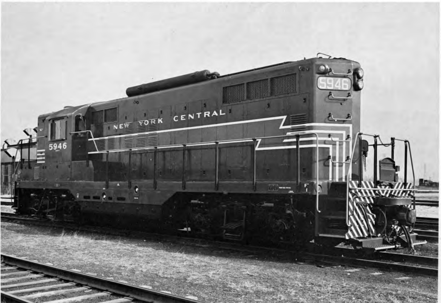
N. Y. C. No. 5946, Class DRSP-9C was a 1750hp GP-9 locomotive built by E. M. D. in December, 1955. It was reclassified DRS-9C after steam generator removal and complete rebuilding by E. M. D. following a severe wreck at Wellington, Ohio in 1960. It was again reclassified ERS-17 and renumbered 7346 in 1966.
