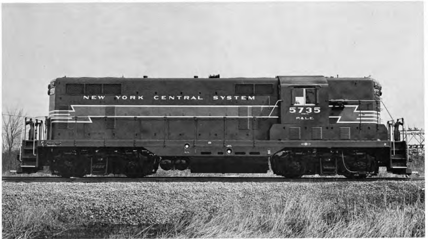
Pittsburgh & Lake Erie No. 5735, Class DRSP-4M was a 1500hp GP-7 locomotive built by E. M. D. in April, 1953. It was renumbered 5928 in June, 1966 and was reclassified ERS-15 at that time.
