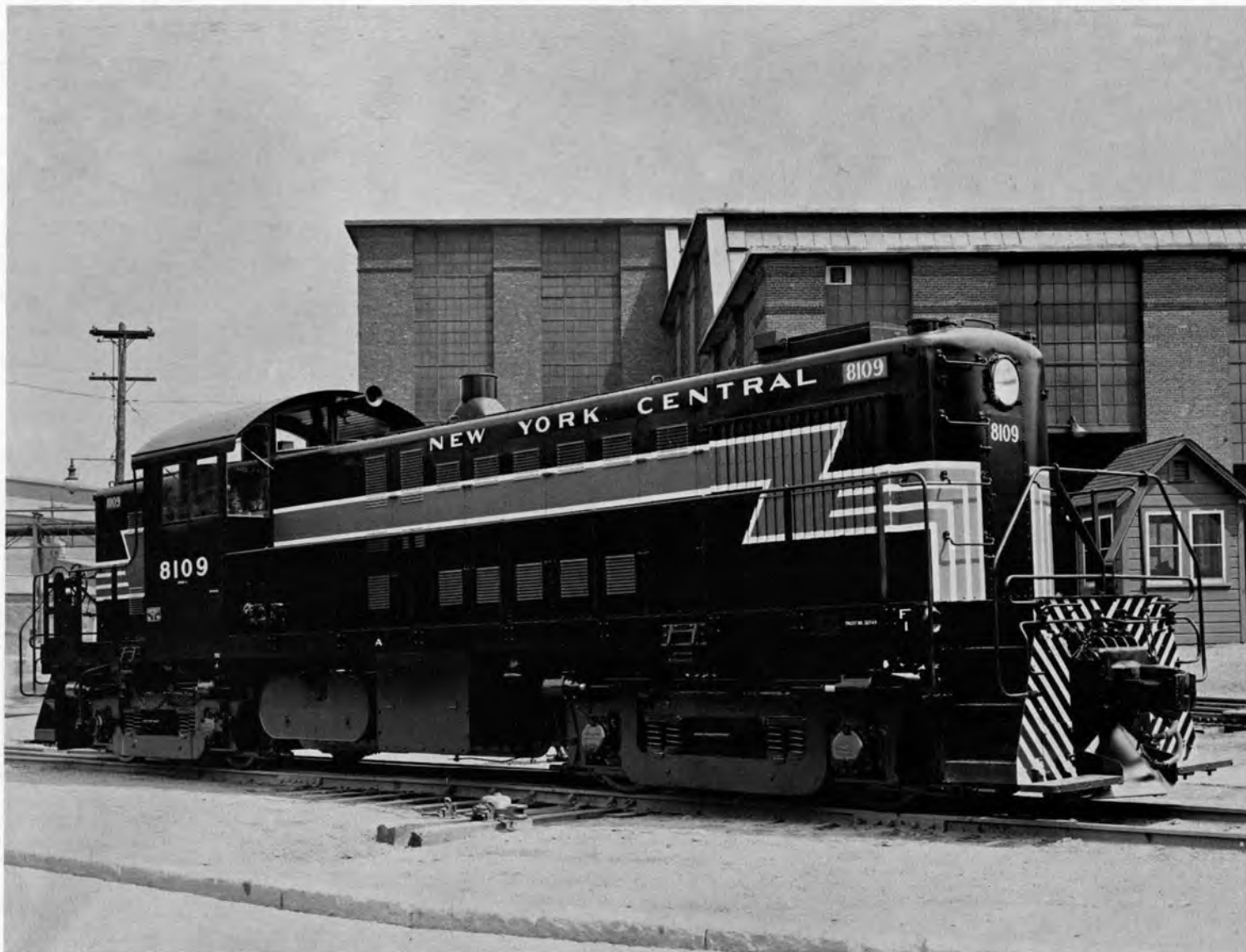
N. Y. C. No. 8109, Class DRS-1C was a 1000hp RS-1 locomotive built by Alco in April, 1950 and was renumbered to 9909 in 1966. This locomotive was equipped with M. U. controls on the #2 end only, and was used mostly in New York state.
