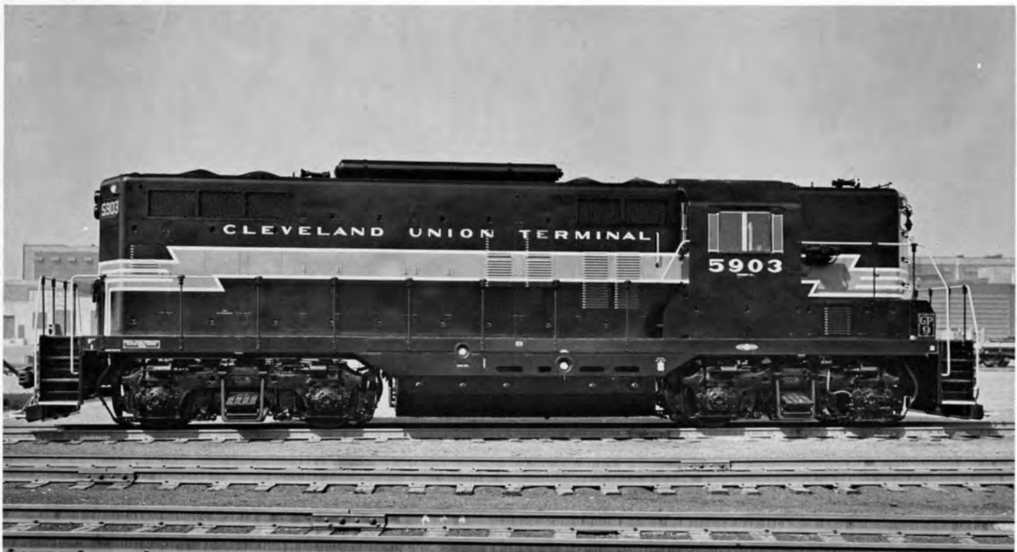
Cleveland Union Terminal No. 5903, Class DRSP-9A was a 1750hp GP-9 locomotive built by E. M. D. in April, 1954. It was renumbered to 7303 and reclassified ERS-17S in 1966 by which time it had lost the "Cleveland Union Terminal" lettering.
