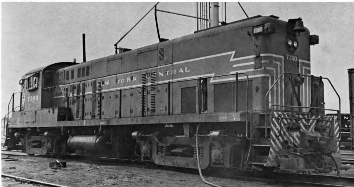
N. Y. C. No. 7300, Class DRSP-3A was a 1500hp 608SC locomotive built by Baldwin in July, 1948. It's original road number when built was 8300 which was changed to 7300 in May, 1951. It was later repowered with an EMD 567C V-16 engine in May 1956 before being retired and scrapped in February, 1966. The locomotive is shown at Collinwood, O. in August, 1959.
