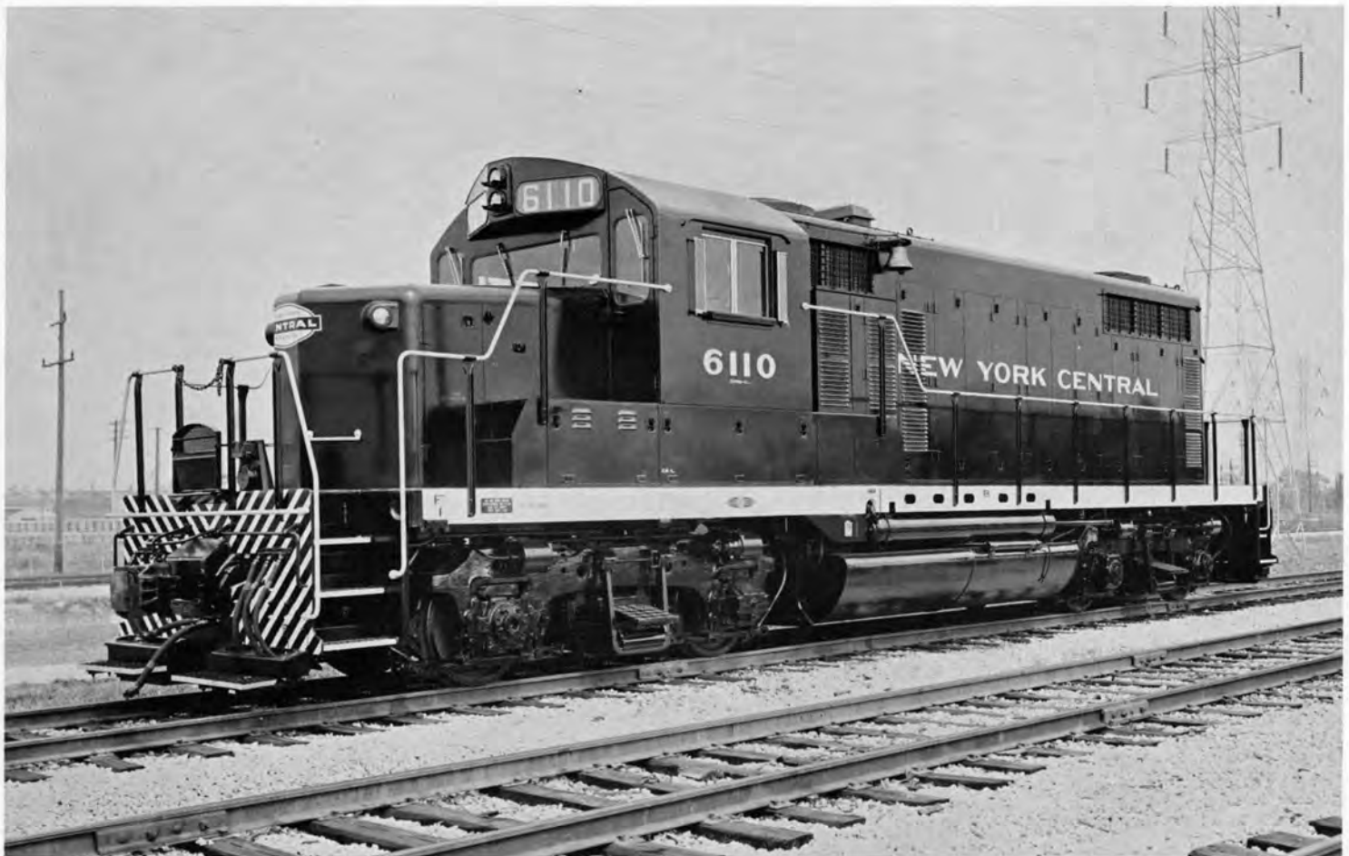
N. Y. C. No. 6110, Class DRS-11A was a 2000hp GP-20 locomotive built by E. M. D. in August, 1961. It was renumbered to 2108 and reclassified EF-20 in 1966. Hood-side mounted bell and lack of dynamic brakes are easy spotting features.
