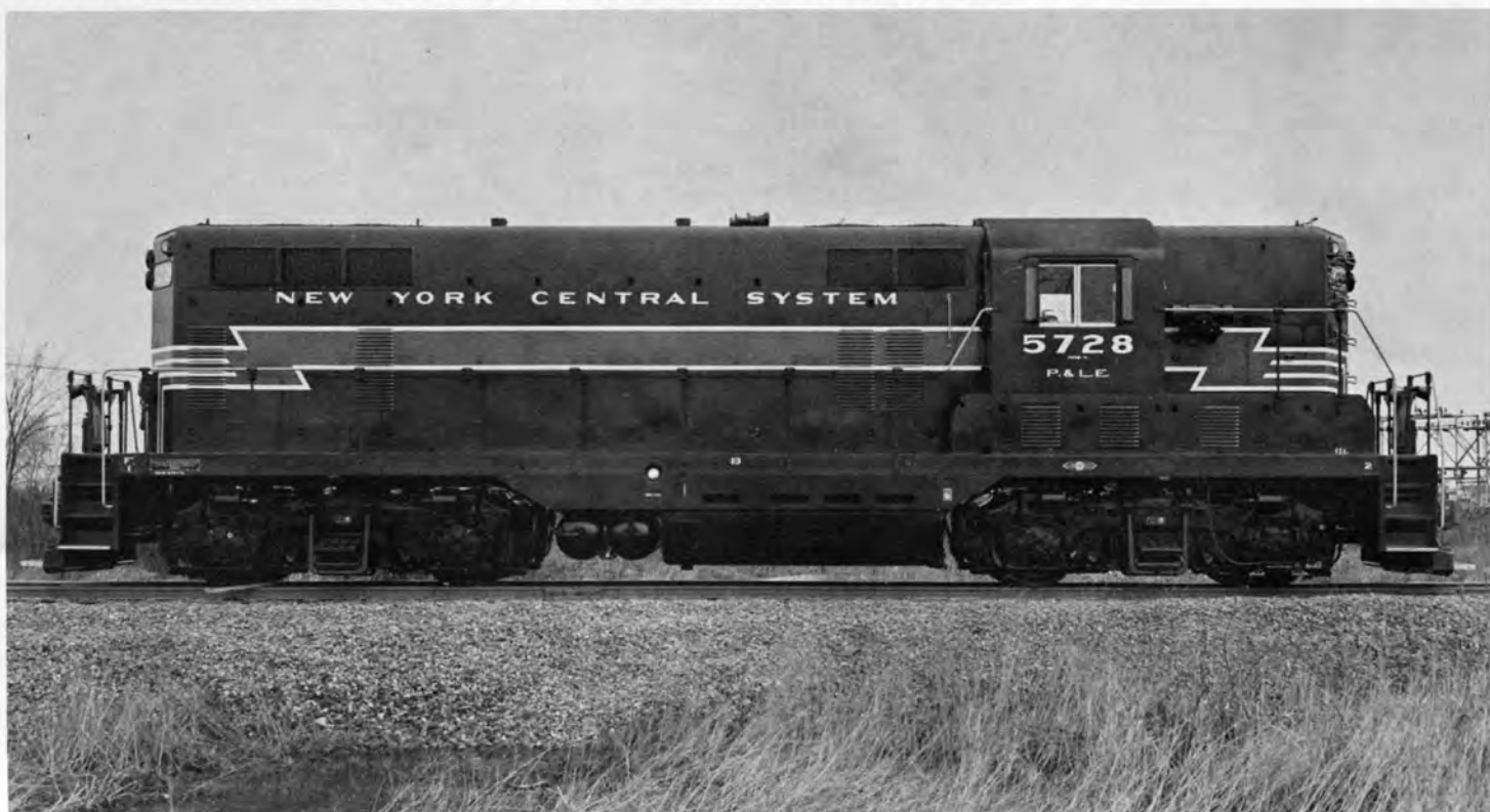
Pittsburgh & Lake Erie No. 5728, Class DRS-4L was a 1500hp GP-7 locomotive built by E. M. D. in April, 1953. Note train control motor-generator mounted near cab on the short hood.
