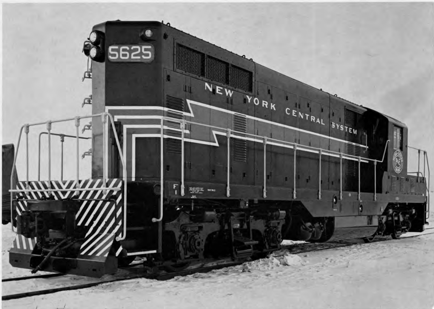
Peoria & Eastern No. 5625, Class DRSP-4D was a 1500hp GP-7 locomotive built by E. M. D. in December 1950. It was later reclassified to DRS-4D when steam generator equipment was removed. In 1966 it was again reclassified to ERS-15.
