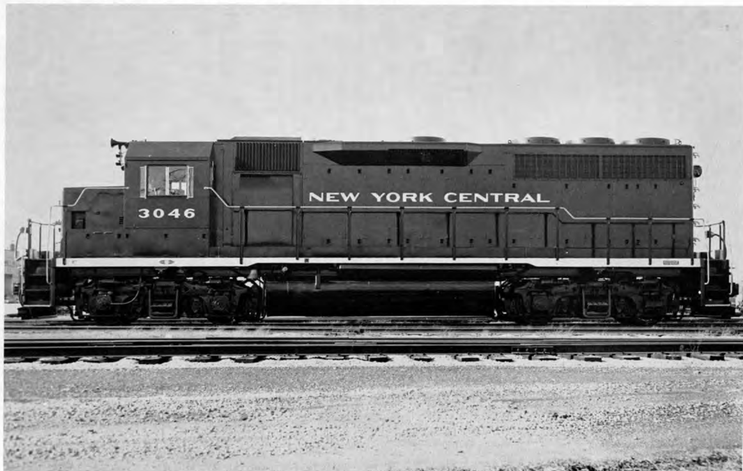
N. Y. C. No. 3046, Class DRS-16A was a 3000hp GP-40 locomotive built by E. M. D. in December, 1965. It was reclassified EF-30 in 1966, same road number. All locomotives in this class equipped with dynamic brakes.
