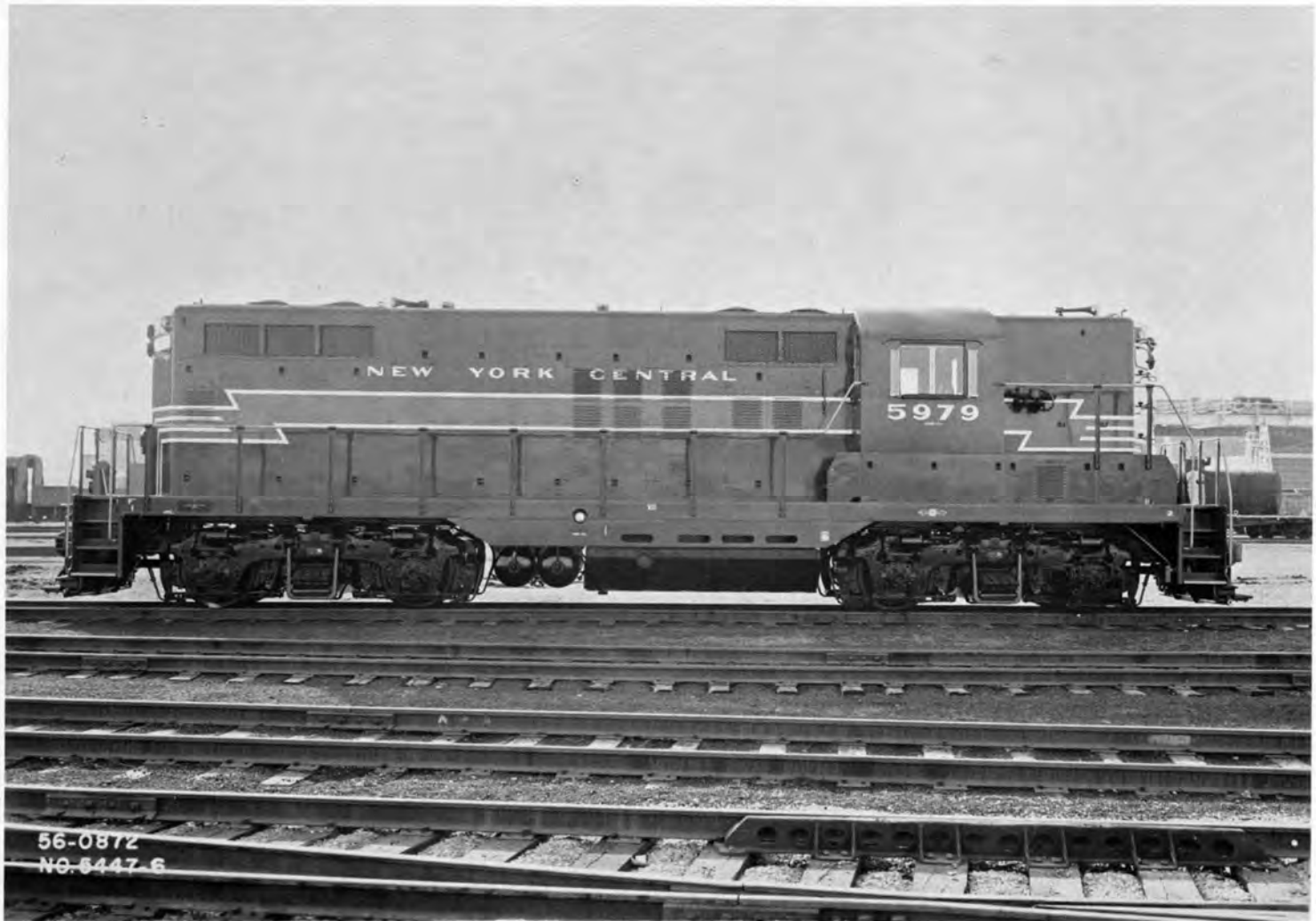
N. Y. C. No. 5979, Class DRS-9D was a 1750hp GP-9 locomotive built by E. M. D. in March, 1956. It was renumbered 7379 and was reclassified in ERS-17 in 1966. Color of carbody appears to be dark gray with black trucks and underframe.
