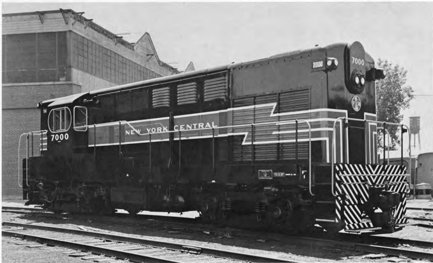
N. Y. C. No. 7000, Class DRS-7A was a 1600hp H16-44 locomotive built by Fairbanks-Morse in July, 1951. It was renumbered to 5100 and reclassified FRS-16 in 1966 before being retired and sold to General Electric in May, 1967.
