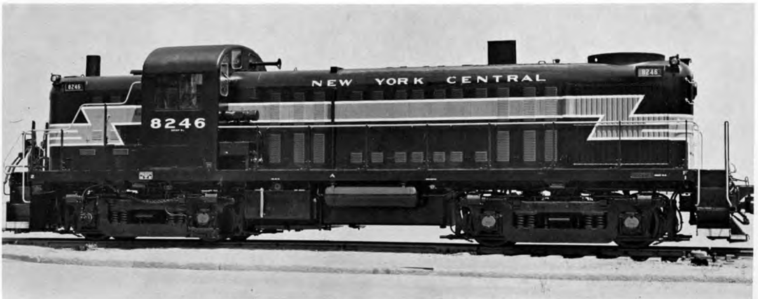
N. Y. C. No. 8246, Class DRSP-6 was a 1600hp RS-3 locomotive built by Alco in June, 1951. It also had steam generator equipment removed and was reclassified to DRS-6C. In 1966 it was renumbered 5246 and again reclassified to ARS-16.
