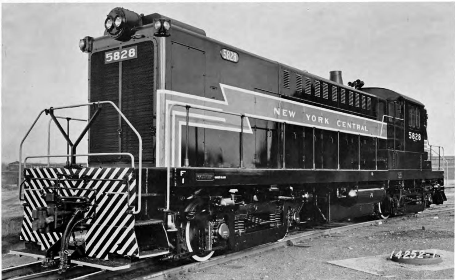
N. Y. C. No. 5828, Class DRSP-8A was a 1200hp RS-12 locomotive built by Baldwin-Lima-Hamilton in November, 1951. It was renumbered 6228 in May, 1953 and was later reclassified DRS-8A with removal of steam generator equipment. In 1966 it was again renumbered and reclassified to 8075, Class BRS-12M.
