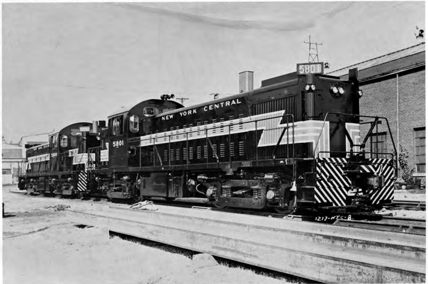
N. Y. C. No. 5801, Class DRSP-5A was a 1200hp model T-89SA locomotive built by Lima-Hamilton in September, 1950. It was renumbered 6201 in May, 1953 and was reclassified to DRS-5A in March, 1961 when steam generator equipment was removed prior to freight service. Locomotive was retired and sold for scrap in February, 1965.
