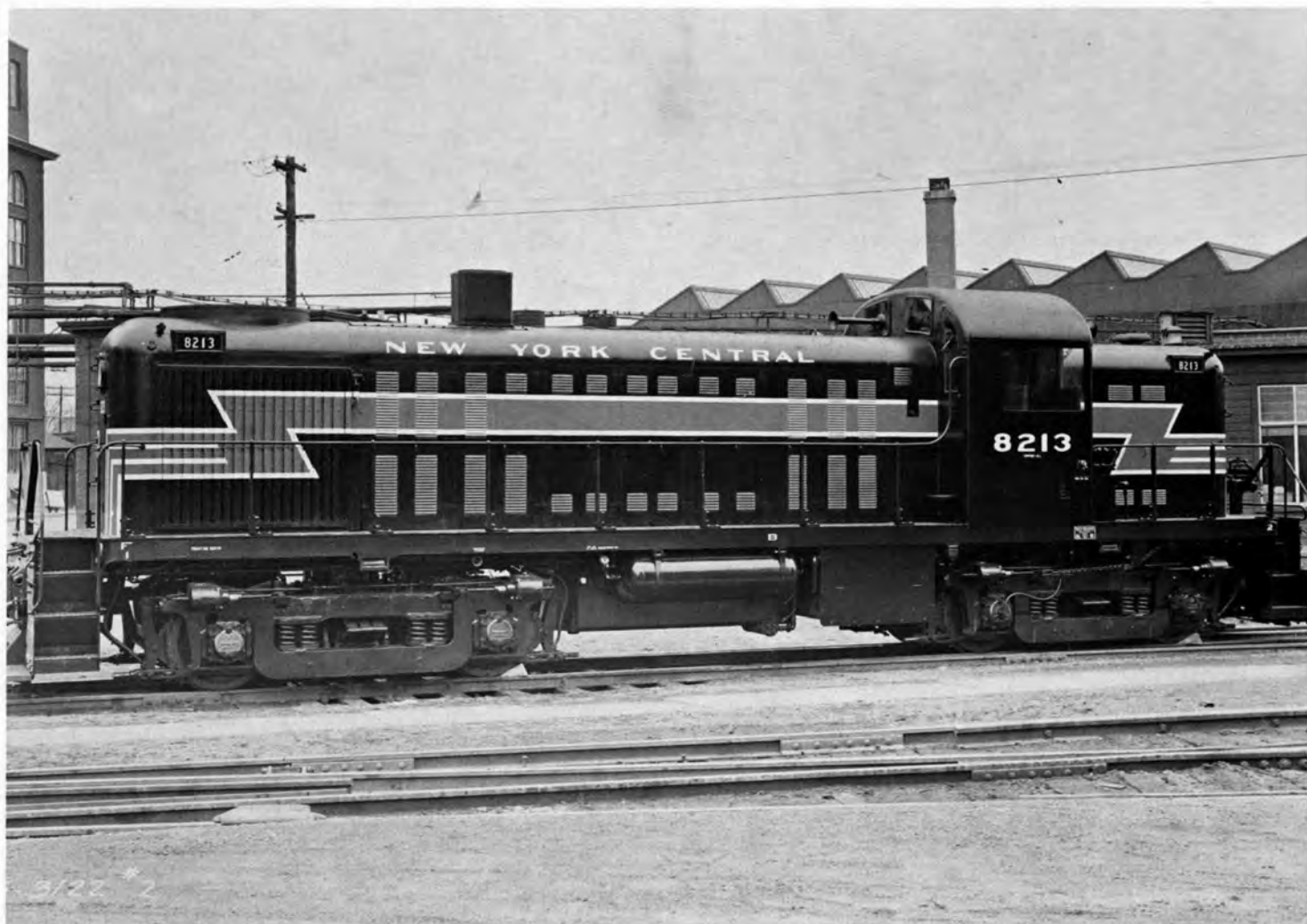
N. Y. C. No. 8213, Class DRSP-2C was a 1500hp RS-2 locomotive built by Alco in February, 1950 and was renumbered to 5213 in 1966 at which time it was also reclassified ARS-16. Steam Generator and other related equipment removed between 1958-60.
