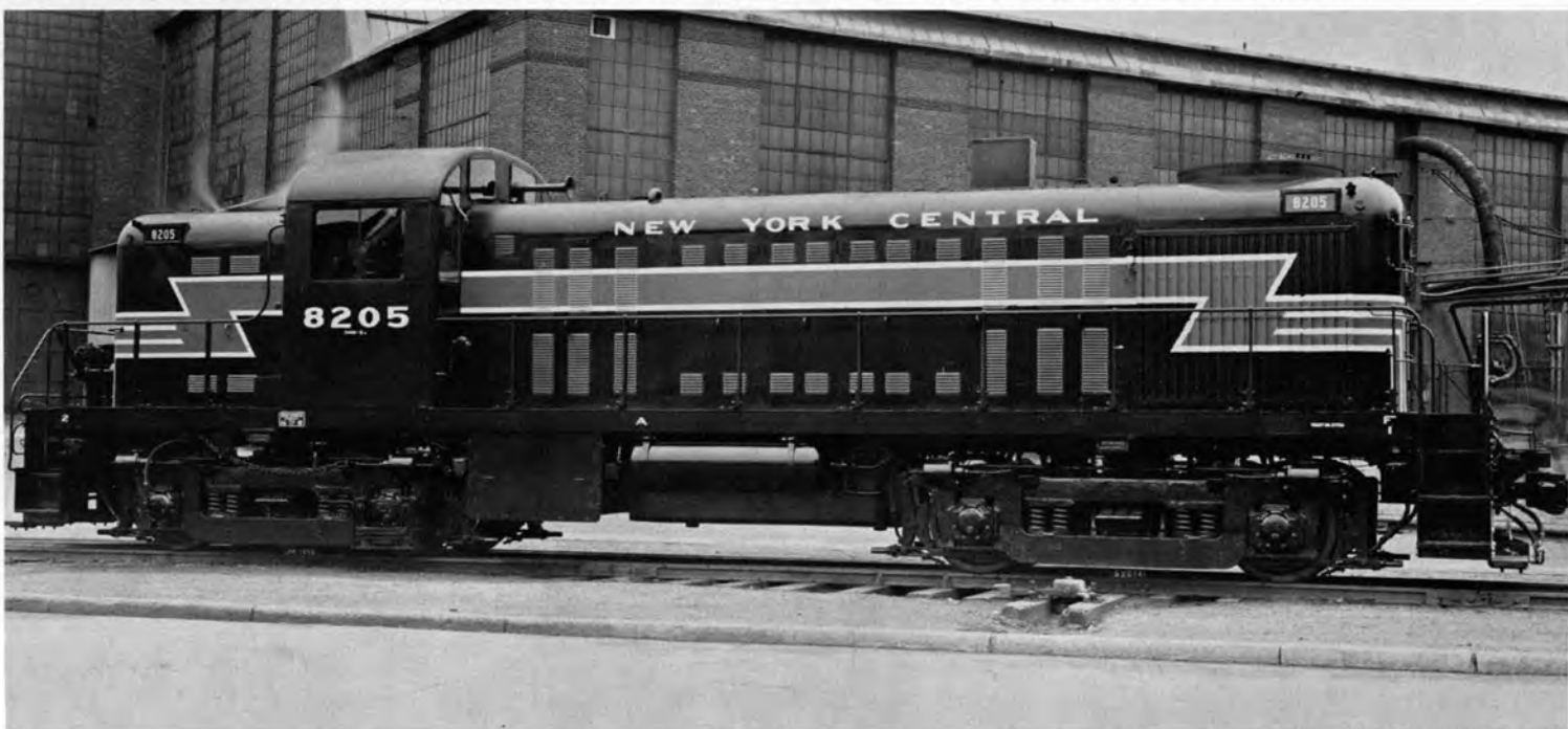
N. Y. C. No. 8205, Class DRS-2B was a 1500hp RS-2 locomotive built by Alco in January, 1949. This locomotive was equipped with M. U. controls on both ends.
