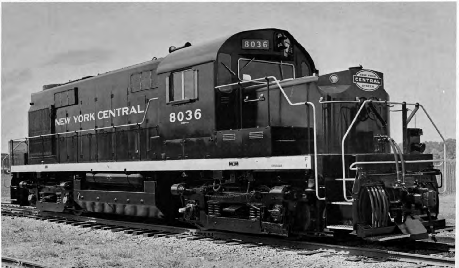
N. Y. C. No. 8036, Class DRS-12A was a 2000hp RS-32 (DL-721) locomotive built by Alco in June, 1962. It was renumbered 2036 and reclassified AF-20 in 1966. Note lack of white "safety striping" on pilot plate which soon became "standard" practice for N. Y. C. road switchers.
