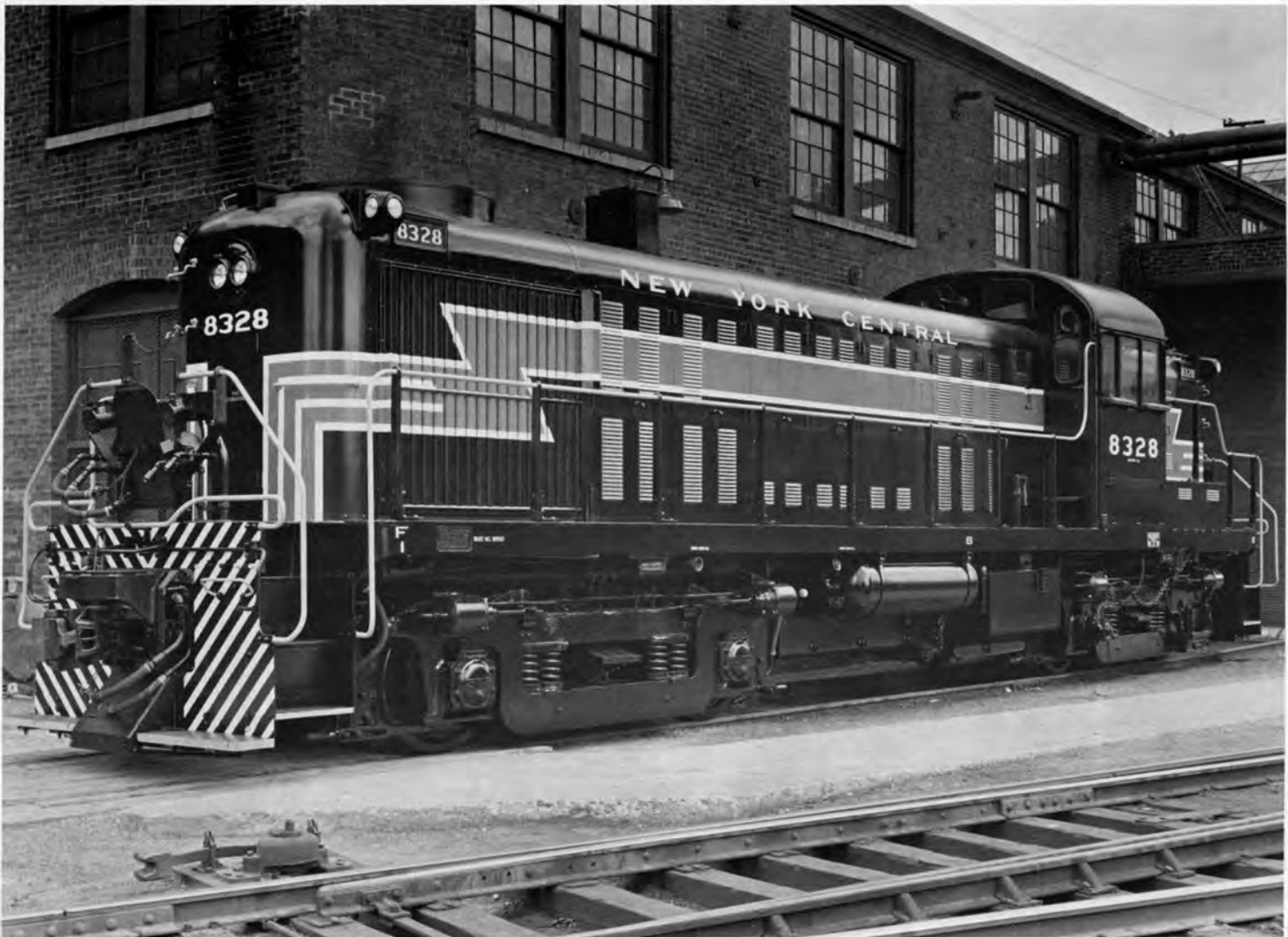
N. Y. C. No. 8328, Class DRSP-6G was a 1600hp RS-3 locomotive built by Alco in May, 1952, and was later rebuilt for freight service with steam generator removal and was reclassified DRS-6G. It was renumbered 5328 and reclassified ARS-16 in 1966.
