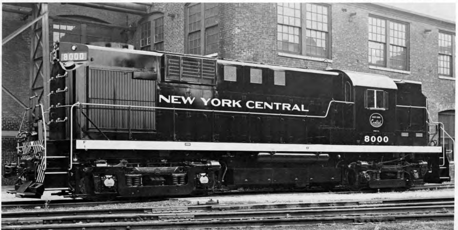
N. Y. C. No. 8000, Class DRS-10A was a 1800hp RS-11 (DL-701) locomotive built by Alco in June, 1957. It was renumbered 7600 and reclassified to ARS-18 in 1966. First N. Y. C. road switcher delivered new in the later "standard" solid black paint scheme. Notice unusual application of N. Y. C. script herald under cab window.
