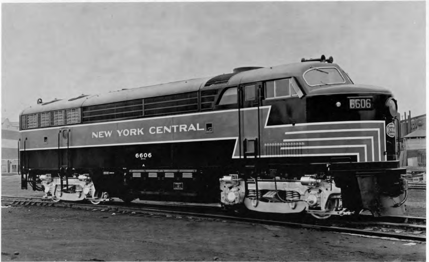
N. Y. C. No. 6606, Class DFA-9A, was a 1600hp. "C Line" locomotive built by Fairbanks-Morse in February, 1952 and was retired in September, 1966. The silver painted trucks shown in this photo were not "standard" for N. Y. C. freight power.
