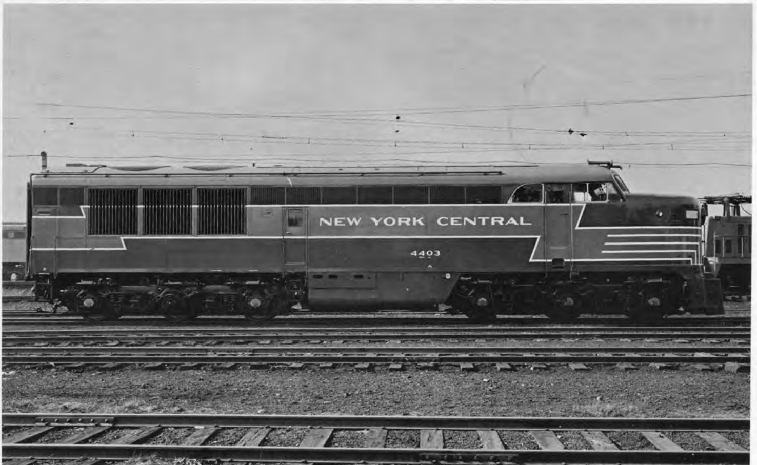
N. Y. C. No. 4403, Class DPA-3A, was a 2000hp. 10 cyl. "OP" powered locomotive built by Fairbanks-Morse at G. E.'s Erie, Pa. works in April, 1949 and was retired from service in January, 1964.
