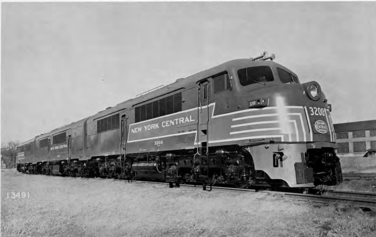
N. Y. C. No. 3200(later 3504), 3300(later 3210 then 3602) and 3201(later 3505) are shown new at Baldwin Locomotive Works in October, 1947. The enclosed drop coupler is shown in the "up" or service position. H. L. Broadbelt Collection
