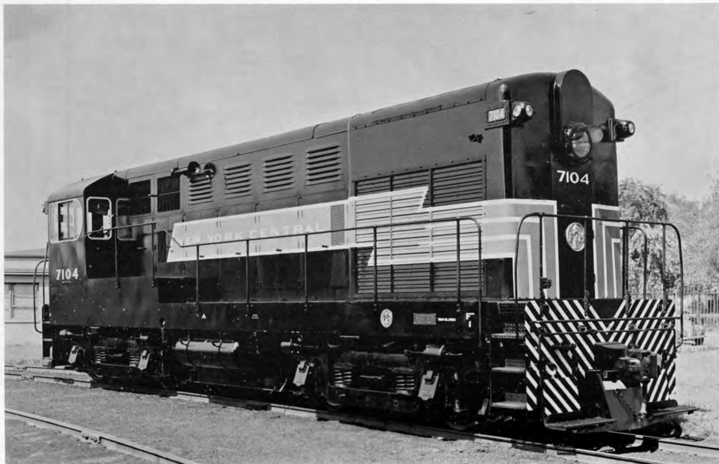
N. Y. C. No. 7104, Class DFT-1A, was a 2000hp. "Transfer Switcher" built by Fairbanks-Morse in August, 1948 and was retired from service in August, 1965.
