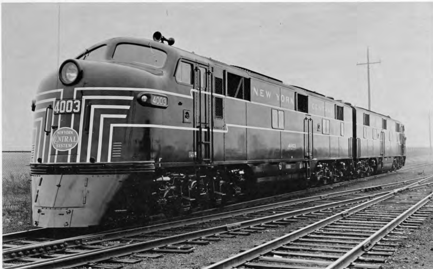
N. Y. C. No. 4003, Class DPA-1A, shown here with 4002 as built by E. M. C. in March, 1945. No. 4003 was severely wrecked near Conneaut, Ohio on March 27, 1953 and was subsequently rebuilt with an E-8 carbody (See Note;)
