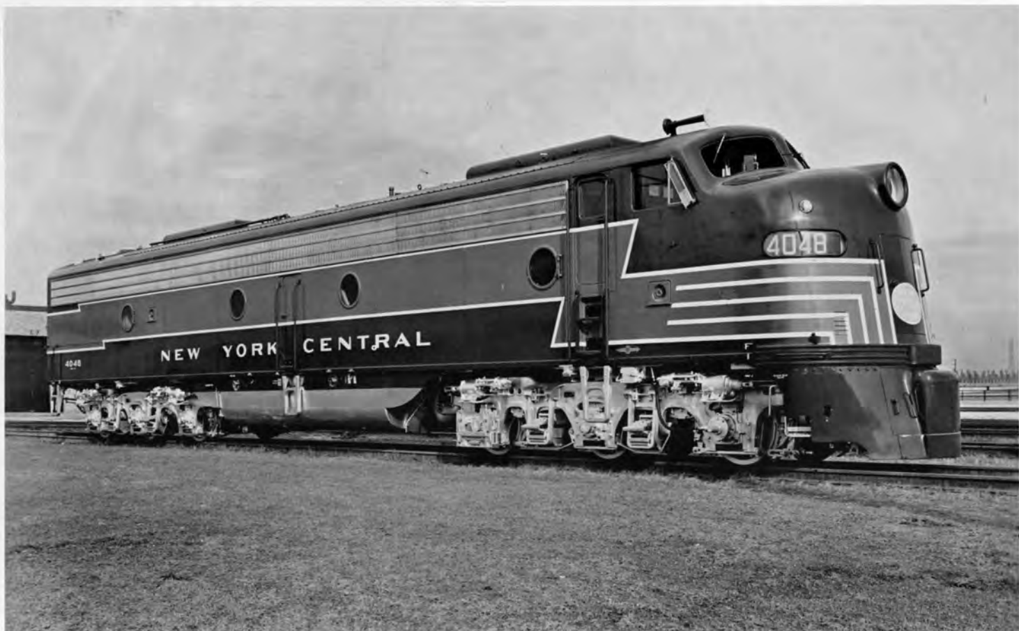
N. Y. C. No. 4048, Class DPA-5B, was a 2250hp. model E-8A locomotive which was built by E. M. D. in January, 1952
