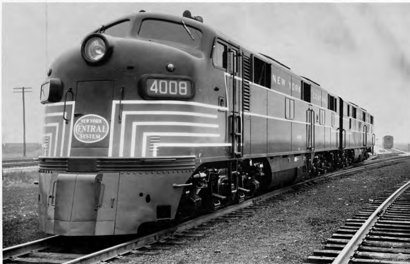
N. Y. C. No. 4008, Class DPA-1B and 4104, Class DPB-1B shown at E. M. C. in April, 1947 where these 2000hp. units were constructed. 4008 displays the newer style enclosed coupler pilot and numberboards.
