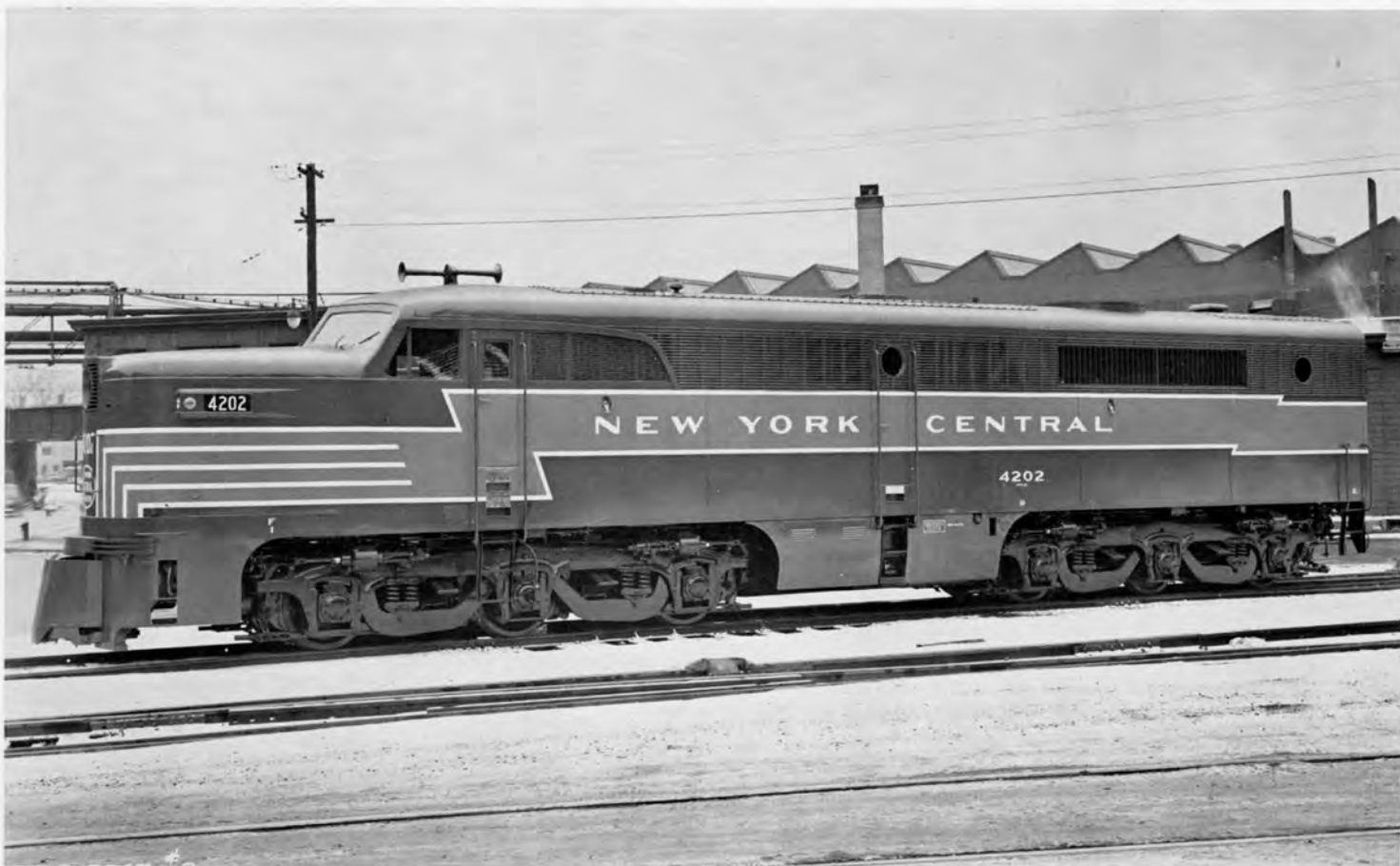
N. Y. C. No. 4202, Class DPA-2B was a 2000hp. locomotive powered by a 16 cyl. model 244 engine. This locomotive was built by Alco in December, 1948 and was retired in April, 1962.
