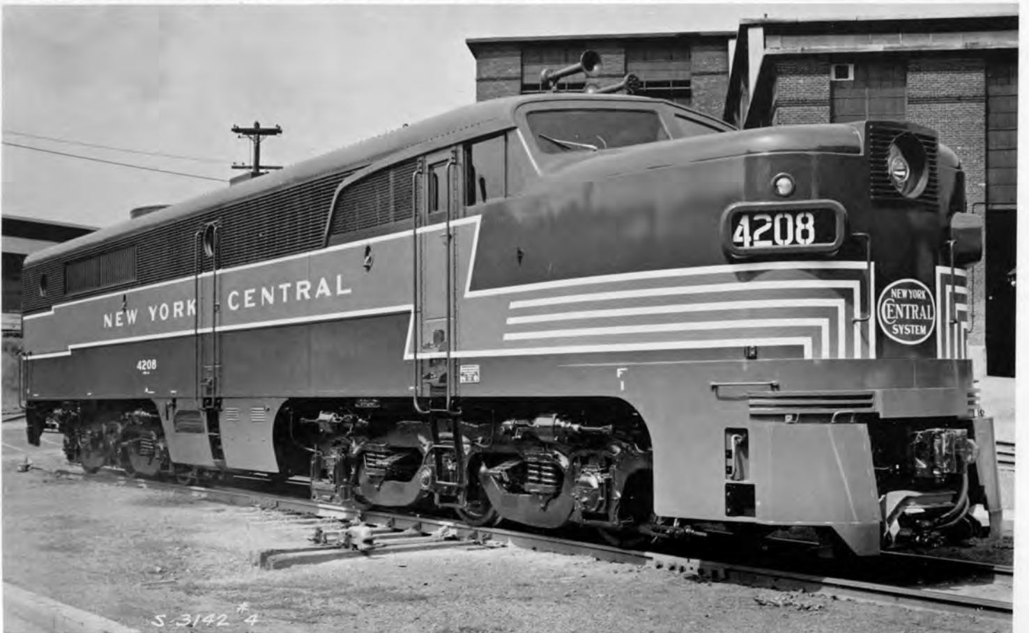
N. Y. C. No. 4208, Class DPA-4A, was a 2250hp. model PA-2 locomotive which was built by Alco in June, 1950 and was retired in April, 1965. The enclosed coupler pilot doors, which were later removed are shown here fully opened.
