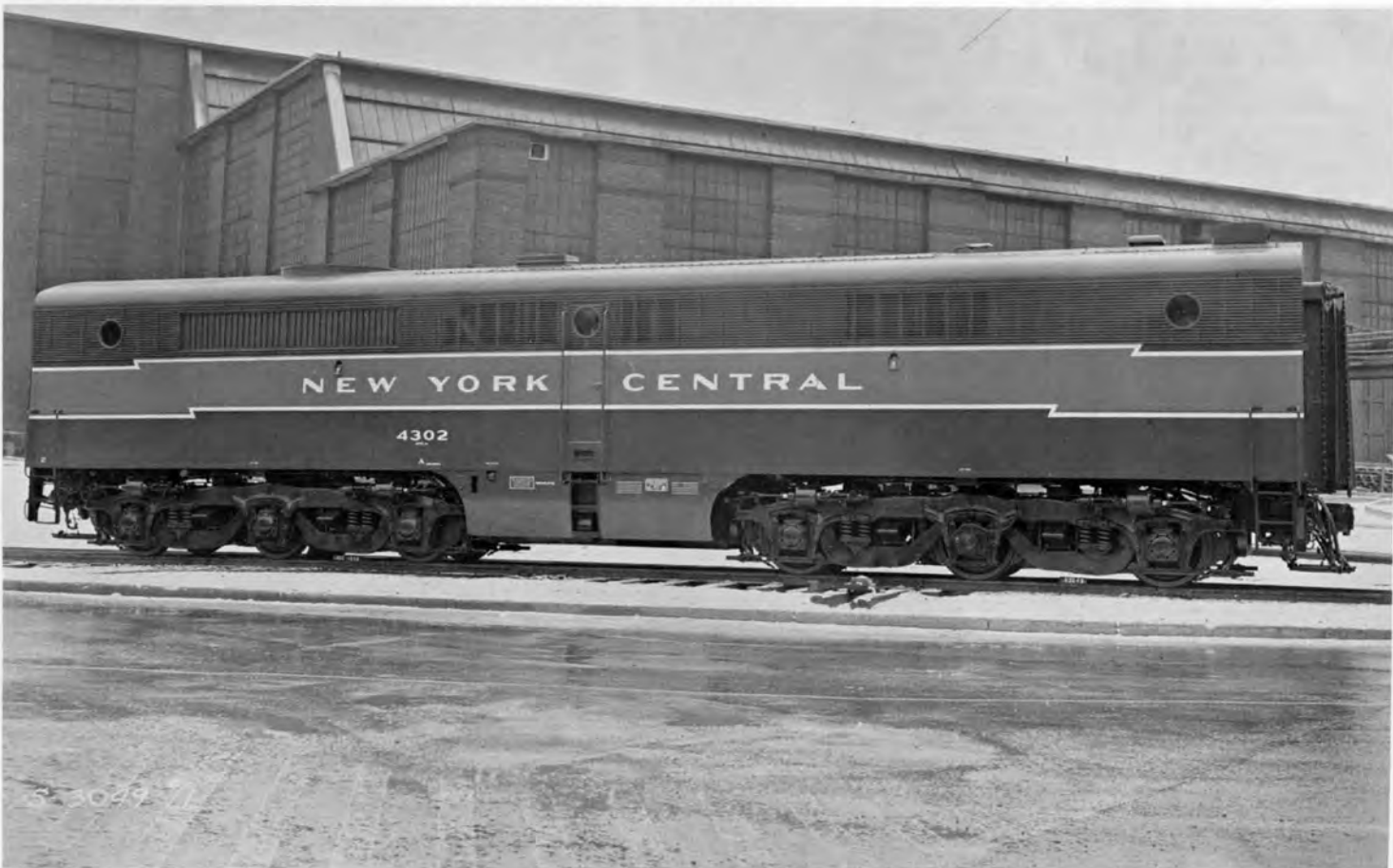
N. Y. C. No. 4302, Class DPB-2B was also built by Alco in December, 1948, but in November, 1955, the original model 244 powerplant was replaced with an E. M. D. 567C (V-16) engine rated at 1750hp. (See Note) Locomotive was retired in April, 1962.
