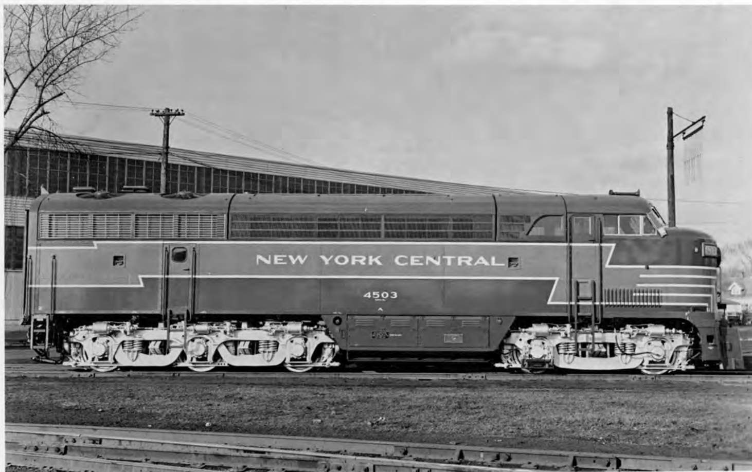
N. Y. C. No. 4503, Class DPA-6A, was a 2400hp. "C Line" locomotive built by Fairbanks-Morse in April, 1956 and was retired in October, 1966. As with 4048 pictured above, silver painted trucks were standard for N. Y. C. passenger power during most of the 1950's.
