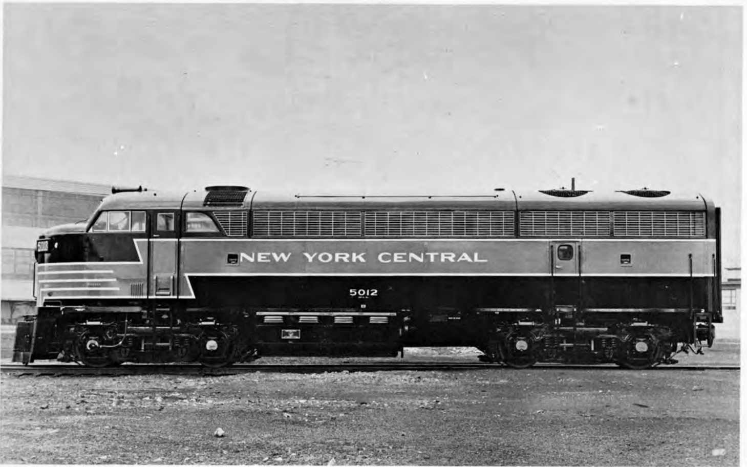
N. Y. C. No. 5012, Class DFA-6A, was a 2000 hp Fairbanks-Morse "C" line locomotive. It was built in April 1950 and re-engined in June 1956 with a 1750 hp EMD 567C engine before being retired in February 1965.
