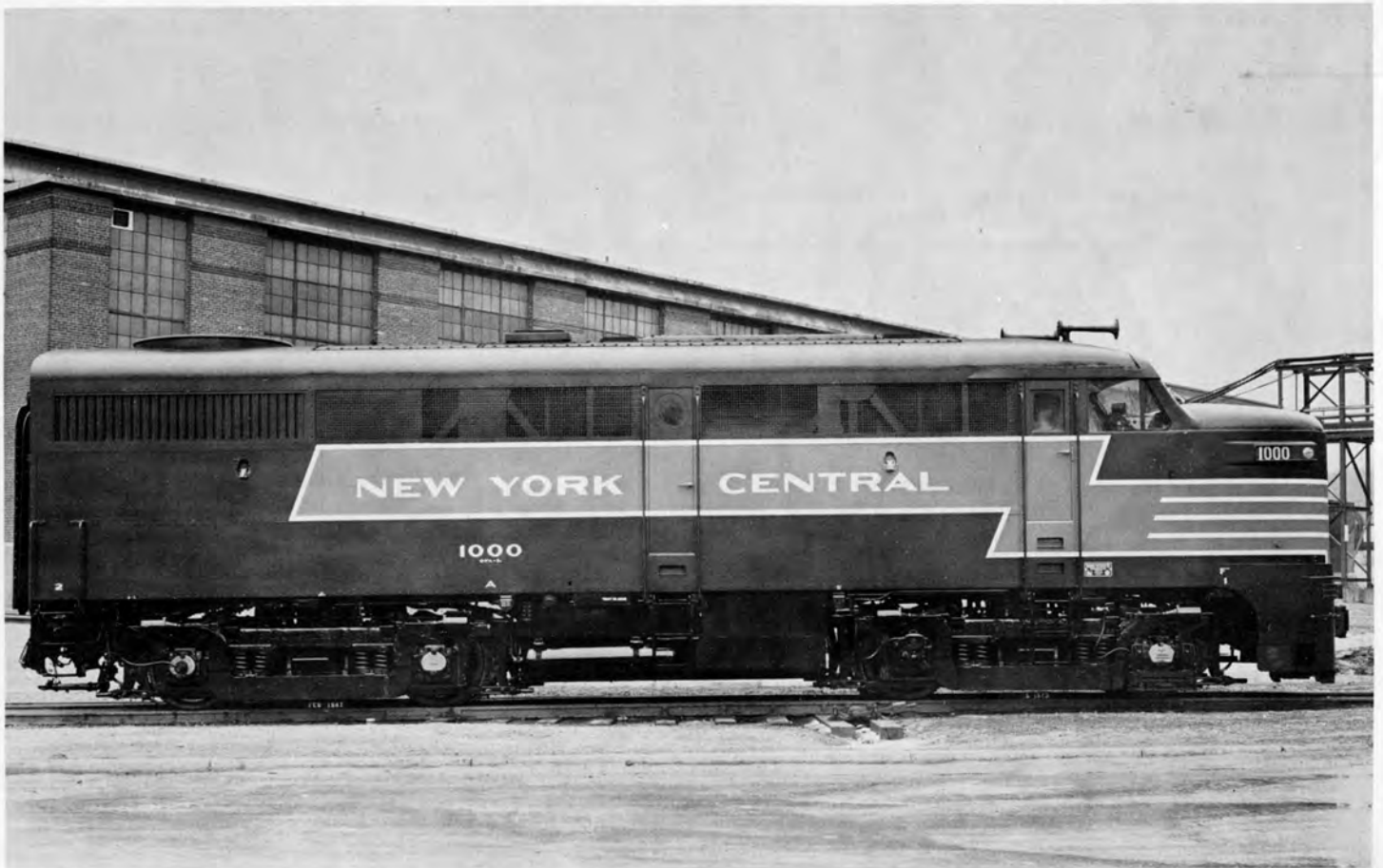
N. Y. C. 's first Alco FA-1 unit was No. 1000, Class DFA-3A, this 1500 hp unit was built in February 1947.
