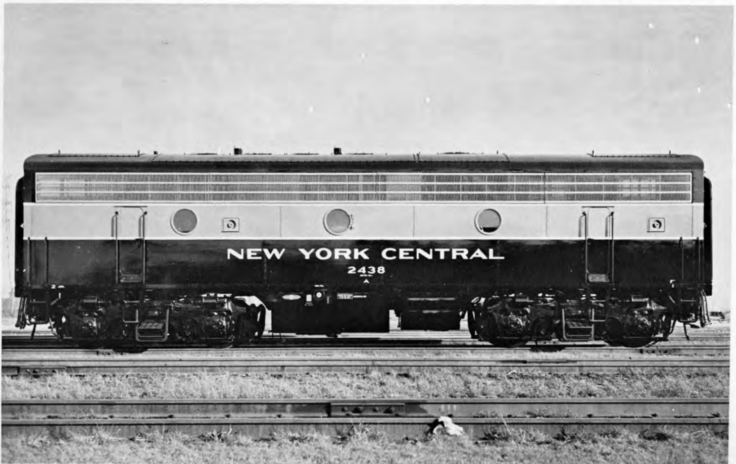
N. Y. C. No. 2438, Class DFB-2F was built by E. M. D. in November 1951. Note late style stainless steel radiator grills.
