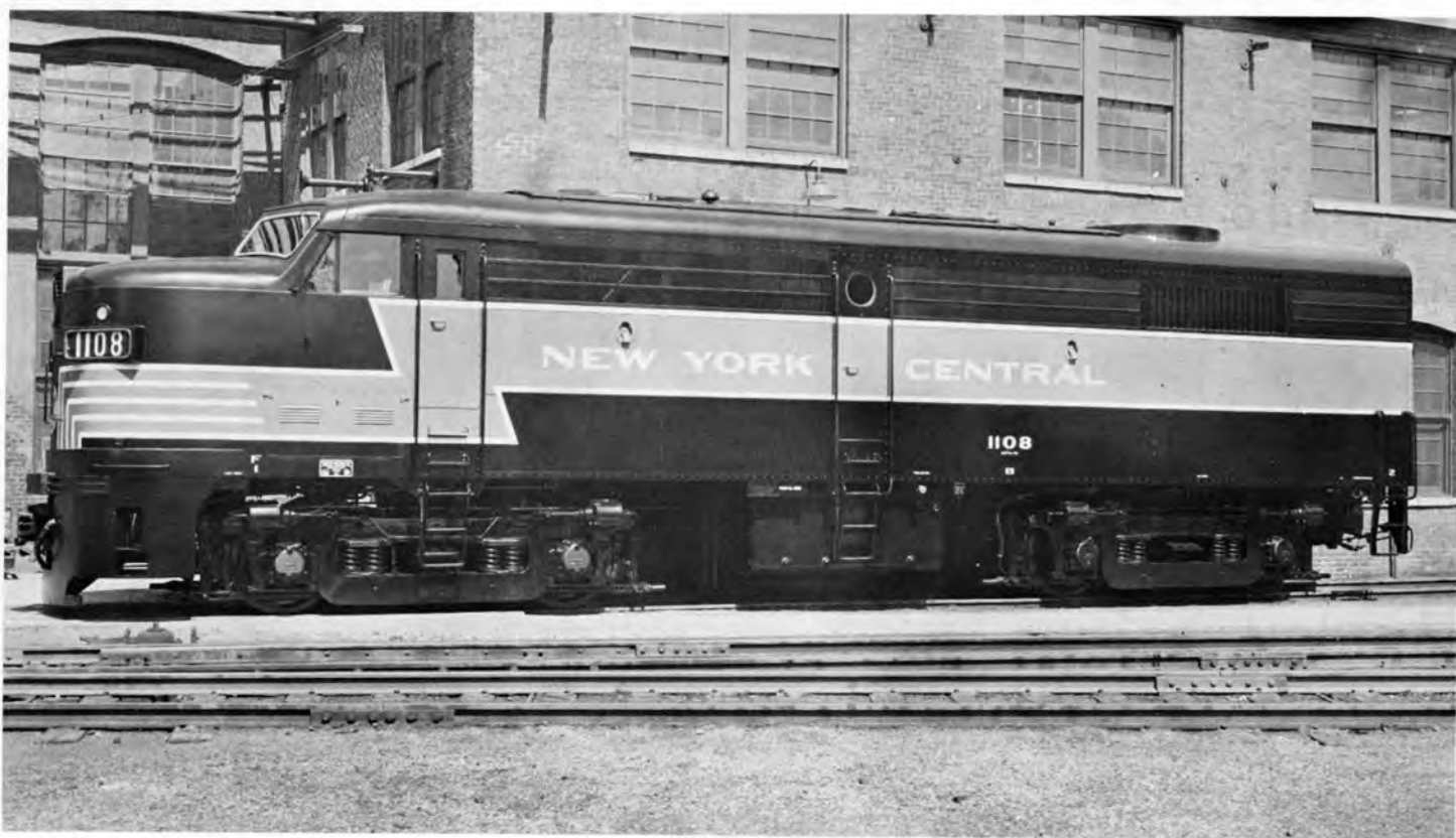
N. Y. C. No. 1108, Class DFA-7D was built by Alco in May 1952. This 1600 hp FA-2 model features a "full length lightning stripe"
