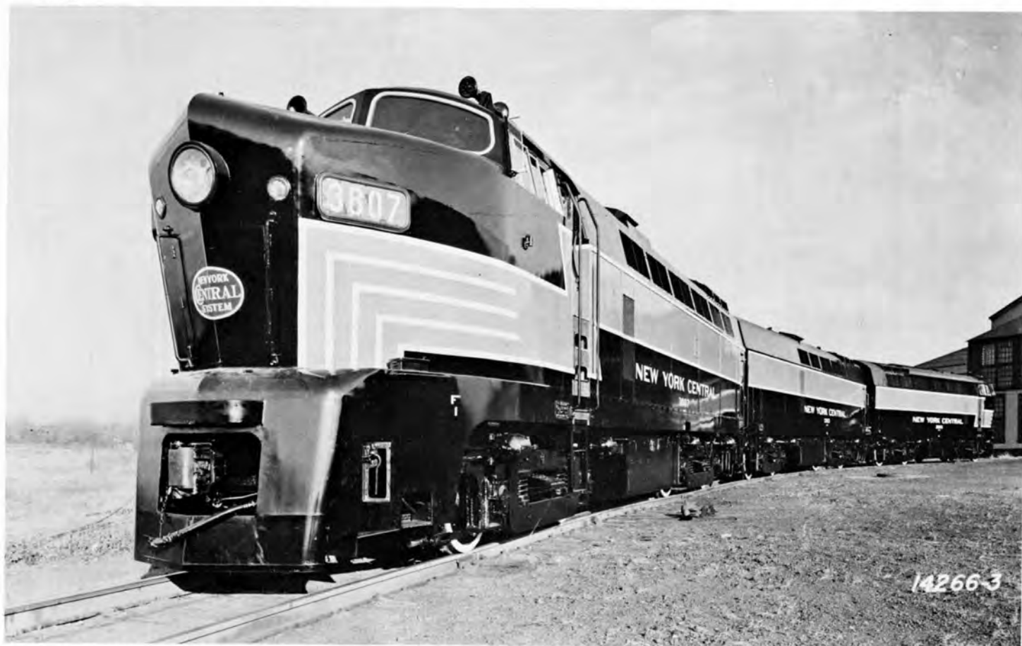
N. Y. C. No. 3807, Class DFA-8A, was a 1600 hp RF-16 "Sharknose" built by Baldwin Locomotive Works in December 1951. It was renumbered 1207 in 1966 before being sold to GE in May 1967. These locomotives spent most of their service life on the "Big Four"
