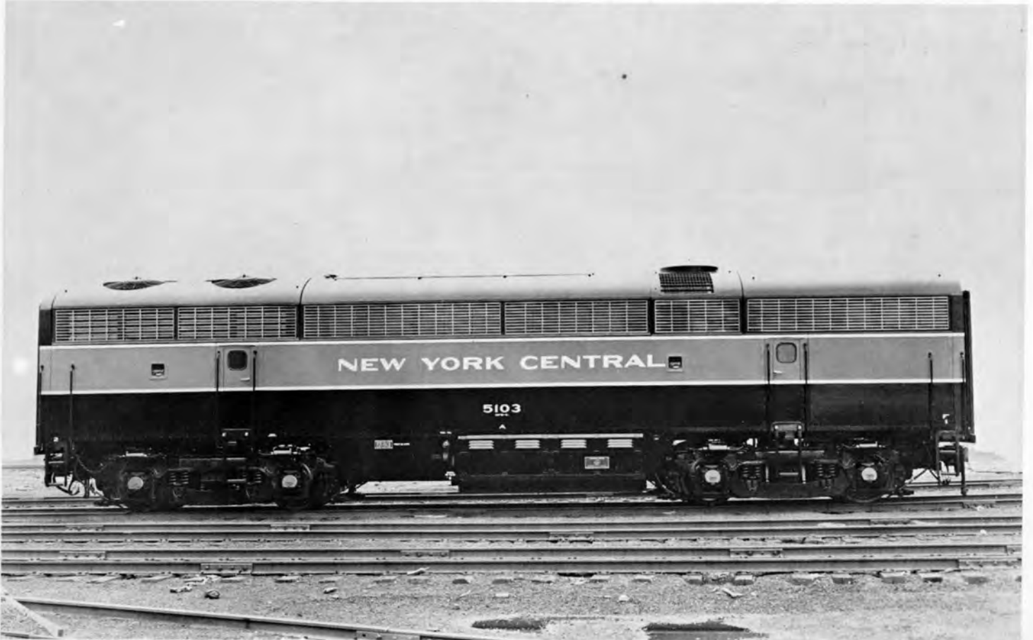
N. Y. C. No. 5103, Class DFB-6A was built by Fairbanks-Morse in June 1950 and was re-engined in December 1956 with a 1750 hp EMD 567C engine. It was finally sold for scrap in March 1966.
