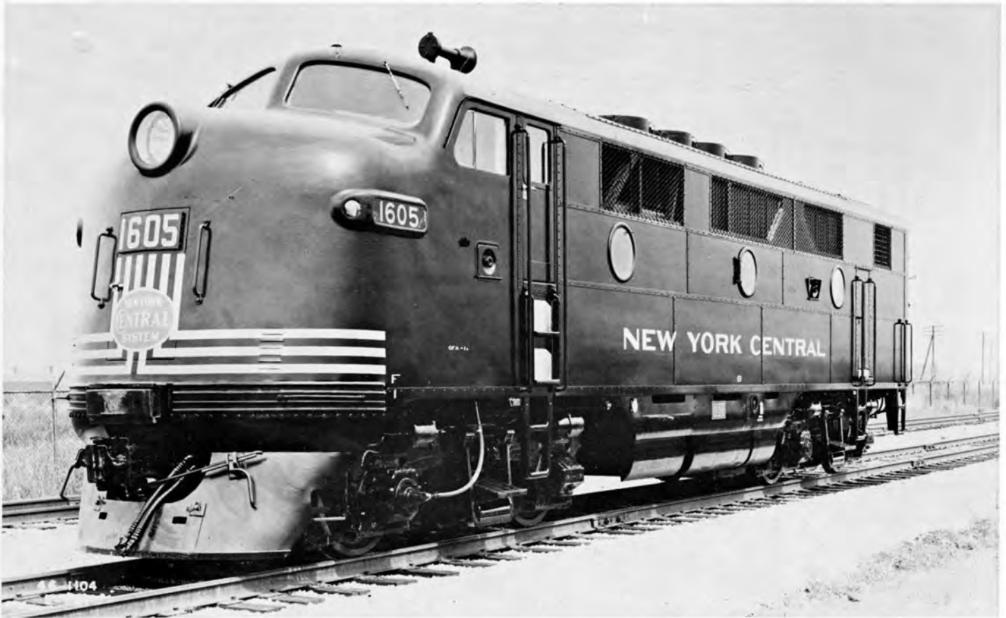
N. Y. C. No. 1605, Class DFA-1B as delivered by E. M. D. in July 1946. Note small number boards and three carbody portholes.
