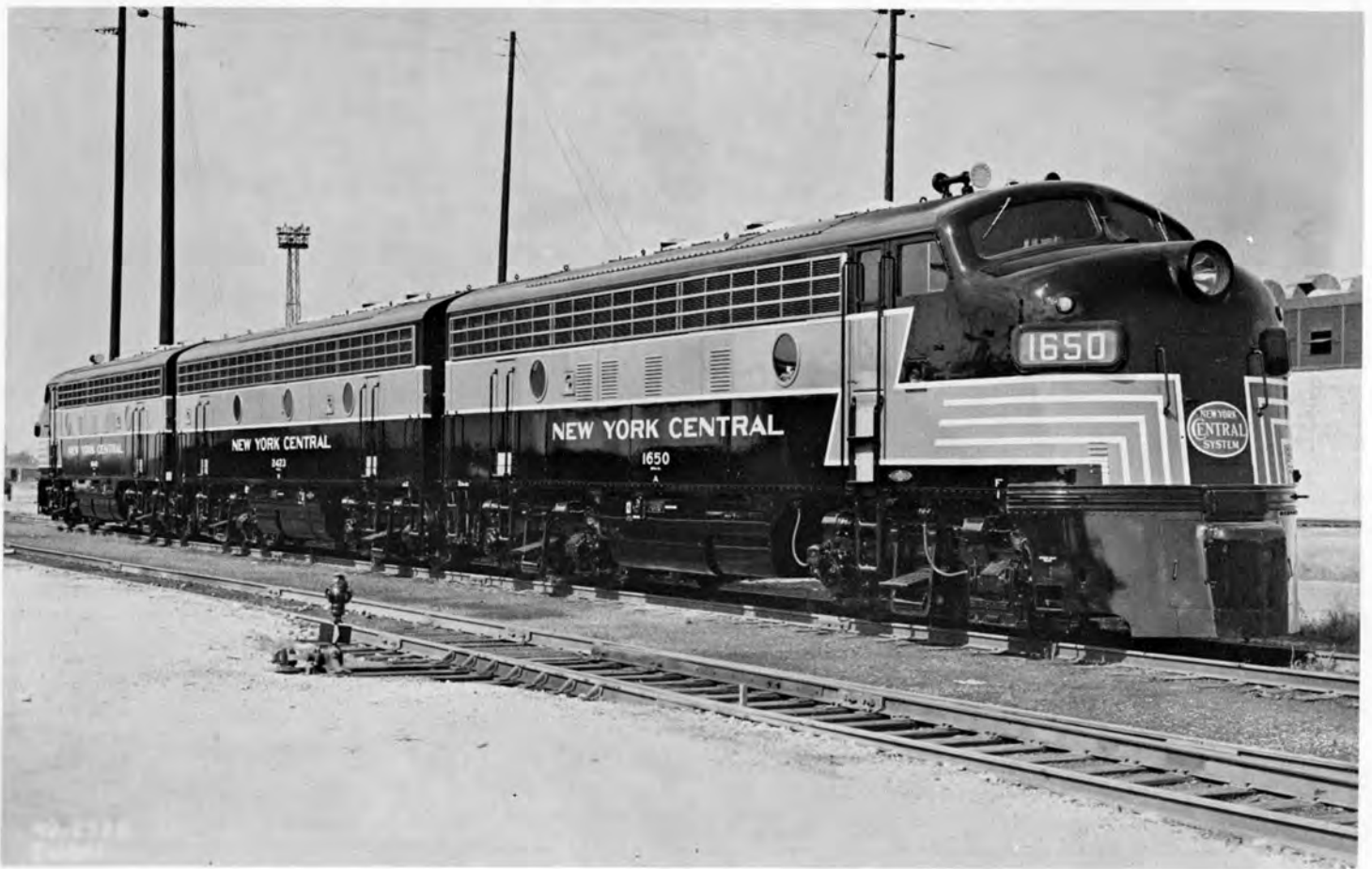
N. Y. C. F-7 model diesels No. 's 1650, 2423, 1649. These 1500 hp locomotives were built by E. M. D. in July 1949.
