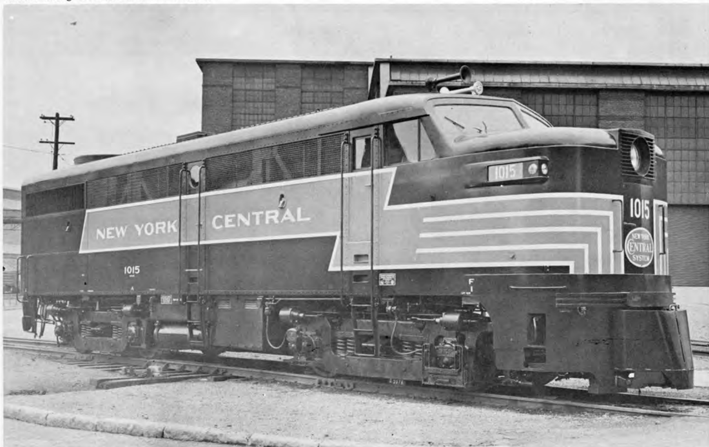
N. Y. C. No. 1015, Class DFA-3C was a 1500 hp unit constructed by Alco-GE in November 1948. Note the rather ungainly enclosed coupler doors on the pilot.
