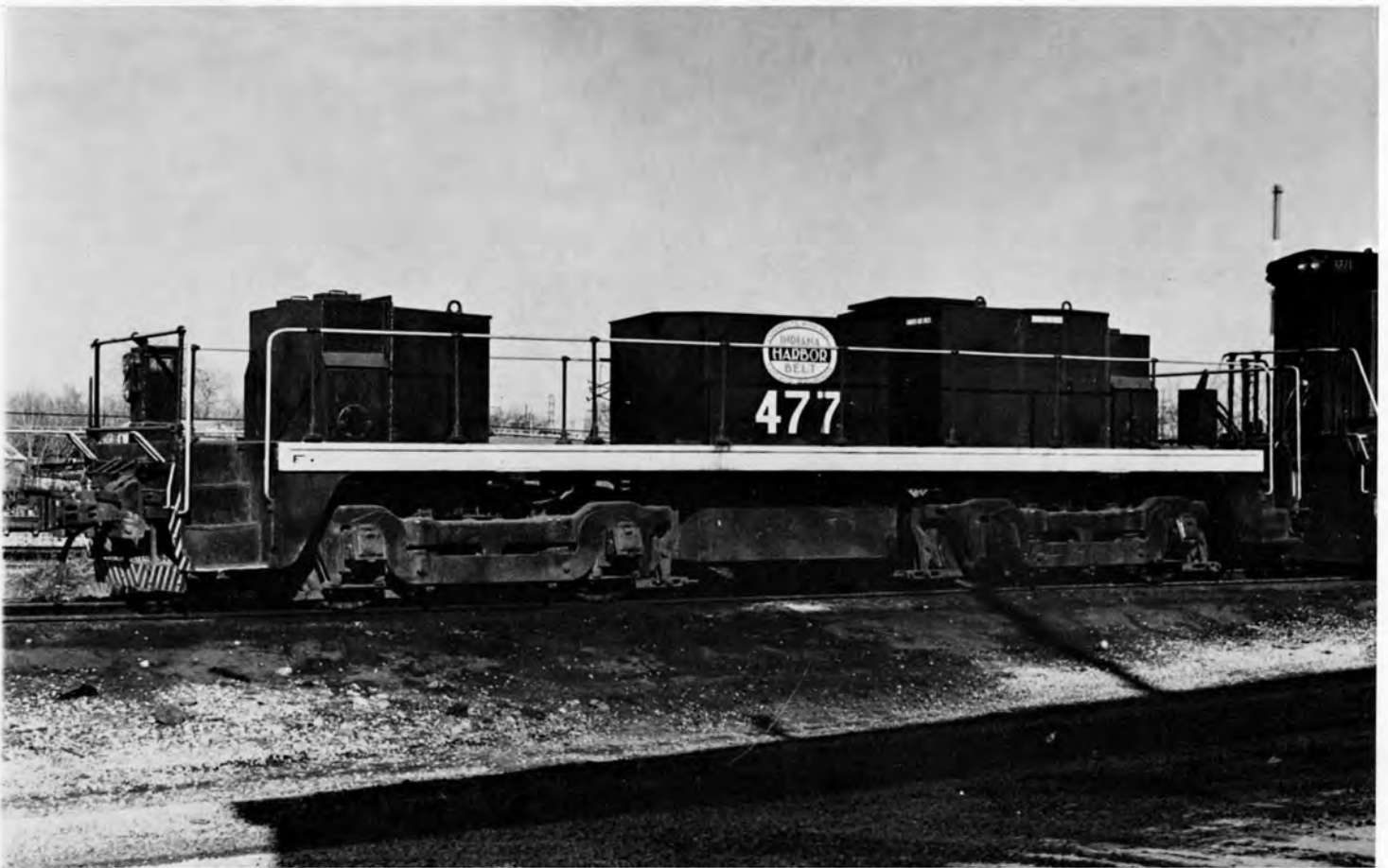
I. H. B. No. 477, Class DHT-2F after rebuilding from wrecked EMD NW-2 No. 8777 (DES-13G) is shown here coupled to a EMD SW-1500 switcher.
