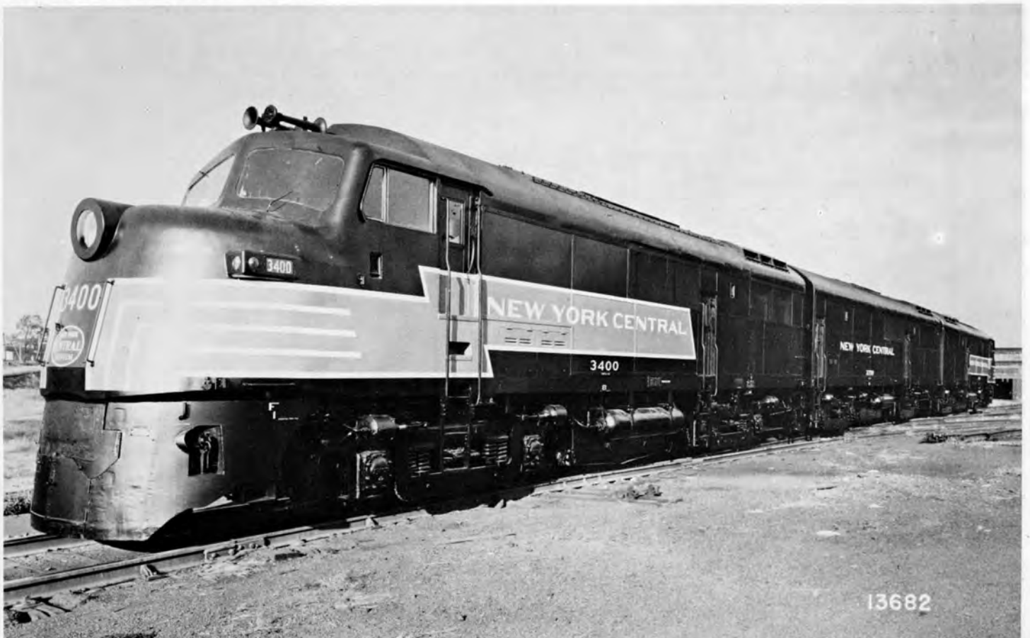
N. Y. C. No. 3400, Class DFA-4A was built by Baldwin Locomotive Works in October 1948 and was renumbered 3800 in June 1951. This DR-4-4-15 unit was finally cut up for scrap in July 1962. H. L. Broadbelt Collection
