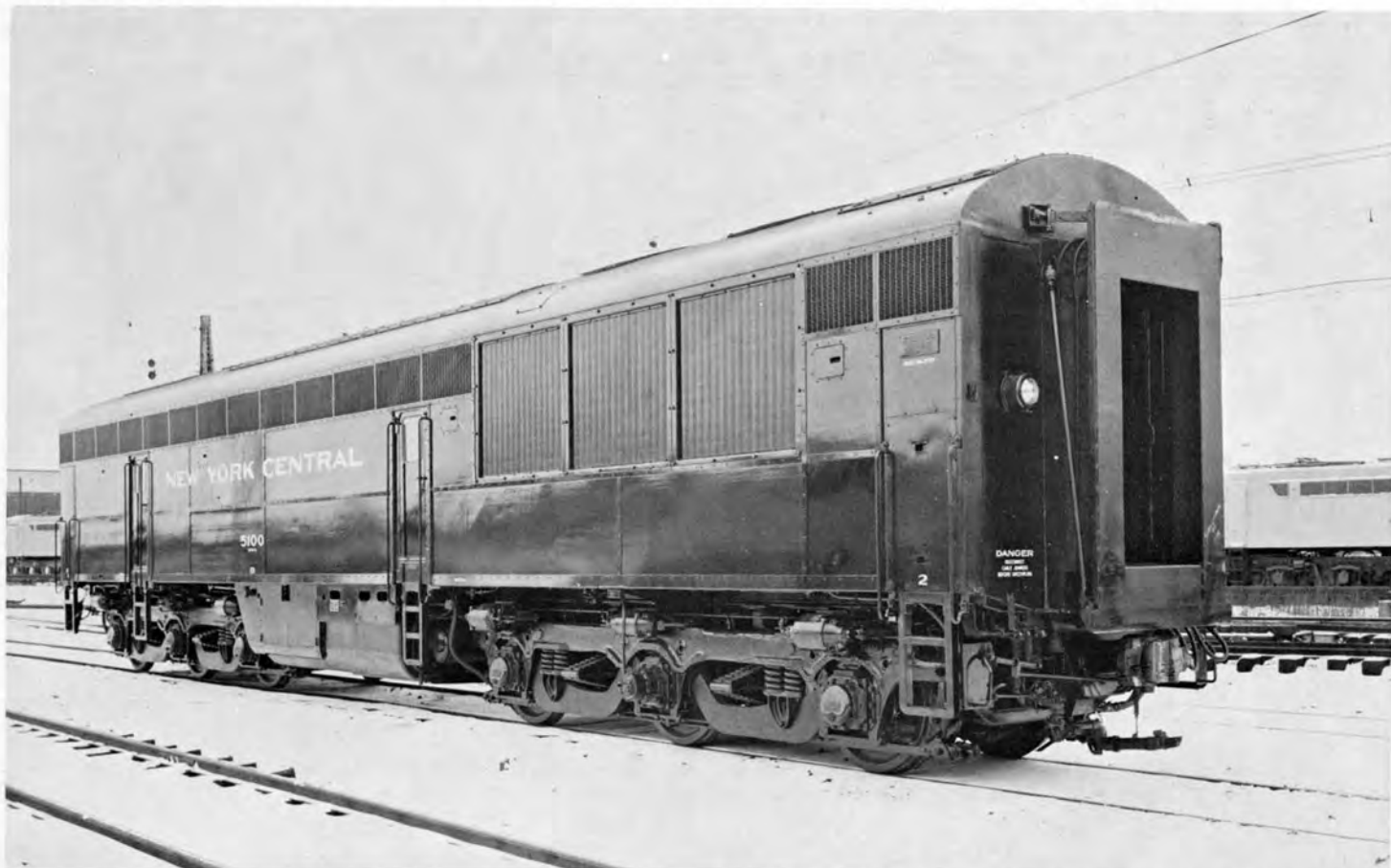
N. Y. C. No. 5100, Class DFB-5A was also an "Erie Built" locomotive rated at 2000 hp. It kept it's original F. M. OP power until it's retirement in December 1960.
