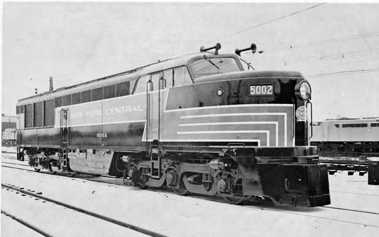
F. M. "Erie Built" No. 5002, Class DFA-5B was built for the N. Y. C. in December 1948, it was repowered with a E. M. D. 567C V-16 engine rated at 1750 hp in November 1957 at Collinwood. It was dropped from the roster in April 1963.
