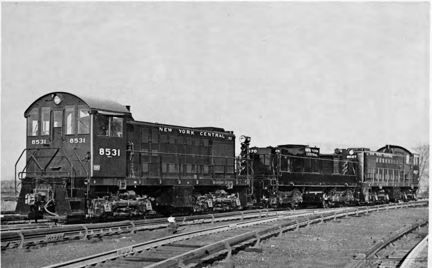
N. Y. C. No. 470, Class DHT-2B shortly after rebuilding from DEs-2 No. 525 is shown here connected to Alco S-2's 8531 & 8527
