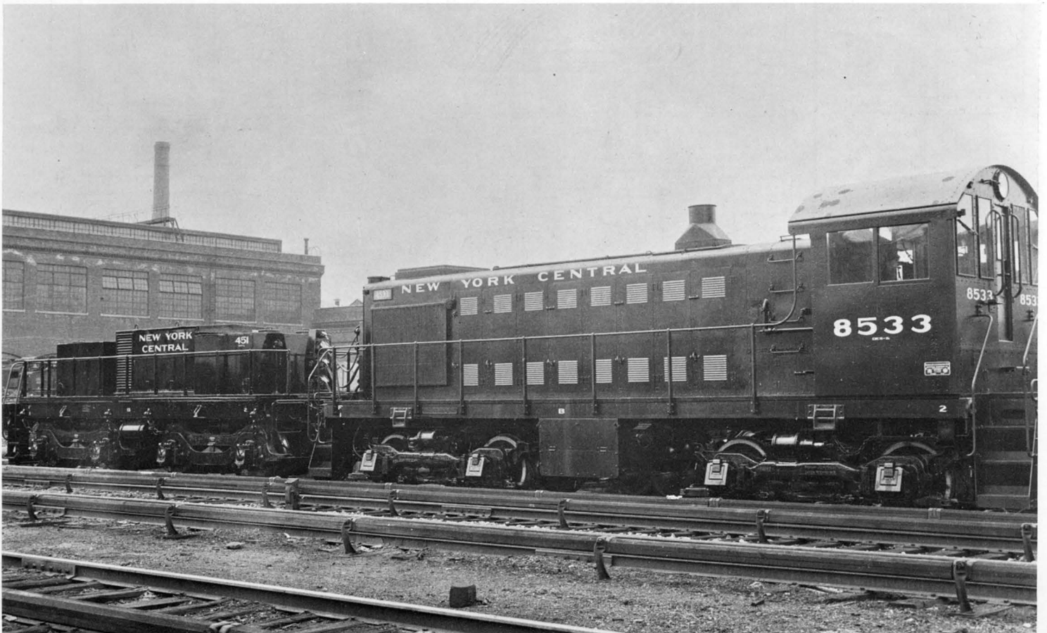
Hump Trailer No. 451, Class DHT-1a, Rebuilt February, 1945, shown here MUed to Alco S-2 8533, Class DES-11c.
