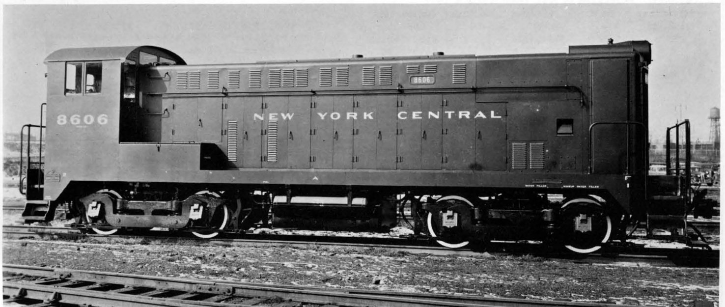
No. 8606, Class DES-12b was a model DS-4-4-10 (VO-1000) switcher built by Baldwin in February 1945 then renumbered 9306 in February 1952 and sold for scrap in February 1964. H. L. Broadbelt Collection.
