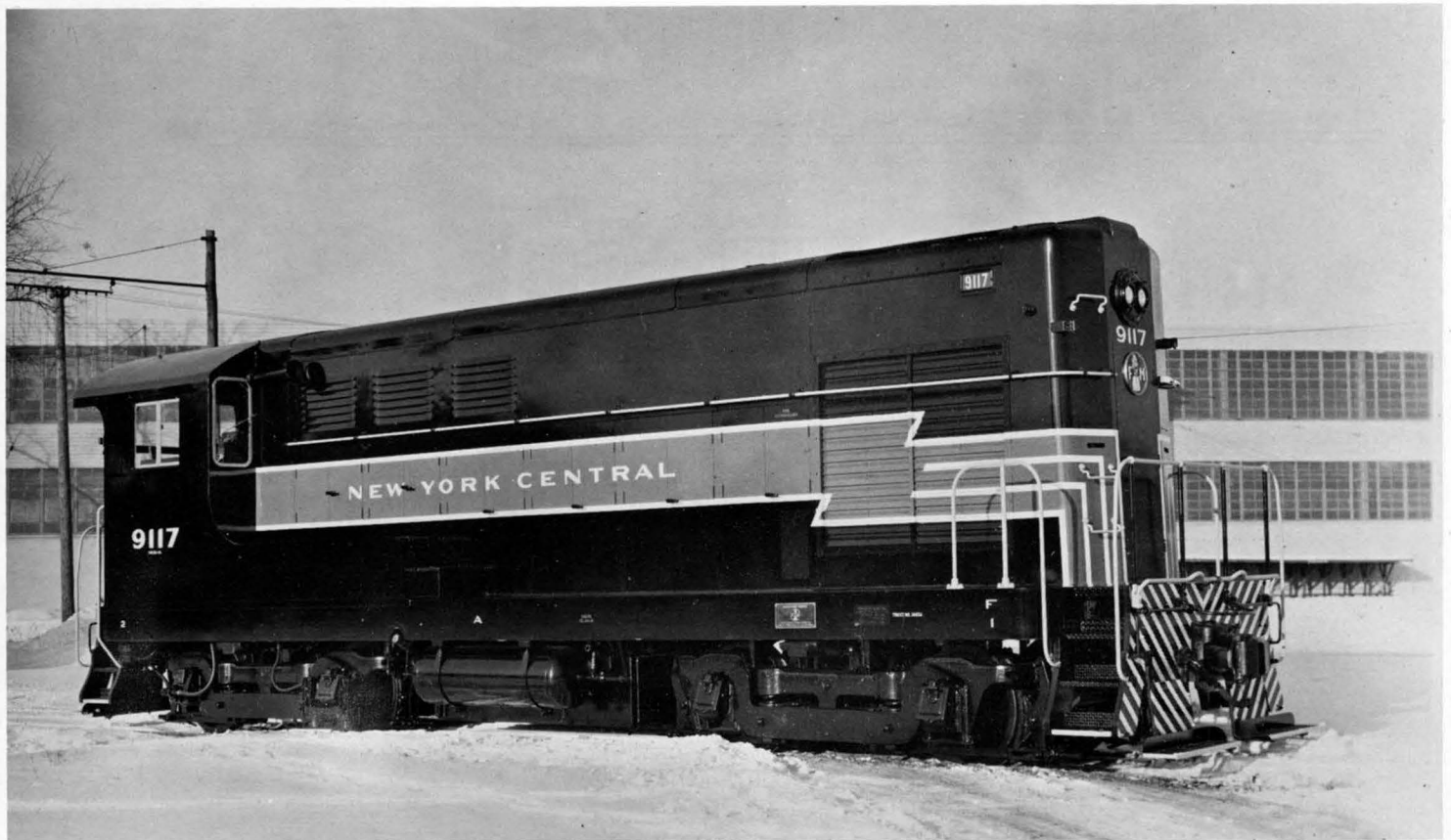
No. 9117, Class DES-17a was a model H12-44 switcher rated at 1200 hp. and built by Fairbanks-Morse in January 1951, and was renumbered 8306 in June 1966 before being retired in August 1967. The "lightning stripe" paint design was unusual for N. Y. C. yard switchers
