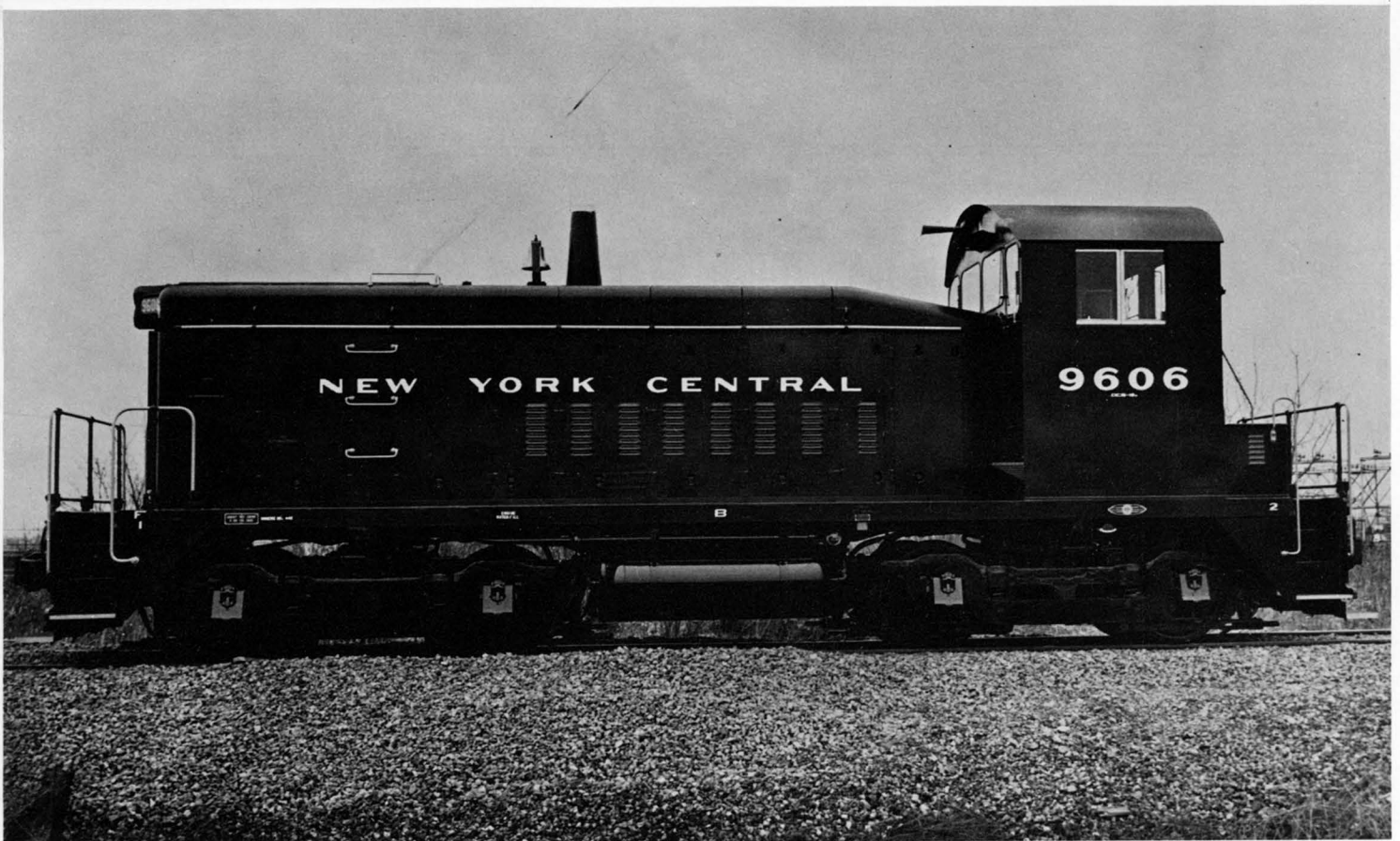
No. 9606, DES-18b was a model SW-8 switcher rated at 800 hp. and built by E. M. D. in February 1952. It was renumbered 8606 in March 1966.
