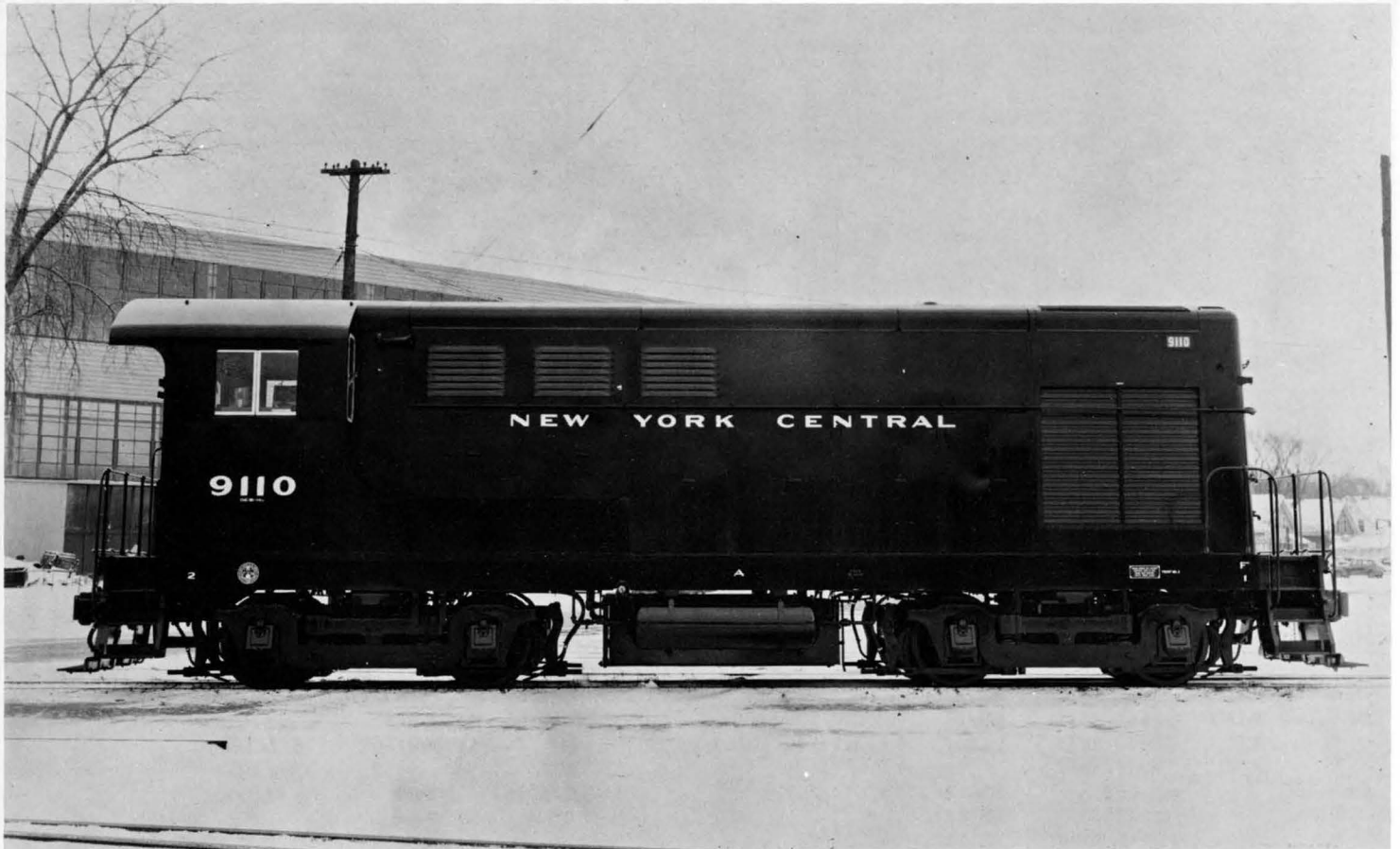
No. 9110, Class DES-14e was a H10-44 model switcher rated at 1000 hp. and built by Fairbanks-Morse in February 1950. This opposed piston powered locomotive was renumbered 8210 in May 1966 and was retired from service in 1967.
