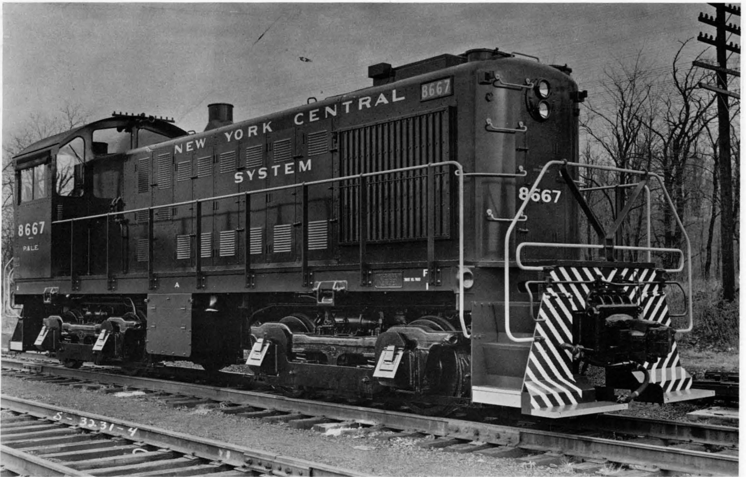
No. 8667, Class DES-11 L Built by Alco-GE for the P&LE in November 1953. This 1000HP S-2 was painted "Pacemaker" green with black trucks. Note that the older type headlight is replaced with a Pyle-National twin sealed beam unit.
