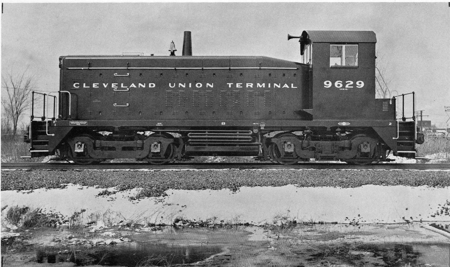
No. 9629, Class DES-21a was a model SW-9 switcher rated at 900 hp. and built for Cleveland Union Terminal in March 1954 by E. M. D. This locomotive was relettered for the N. Y. C. and renumbered 8629 in May 1966.
