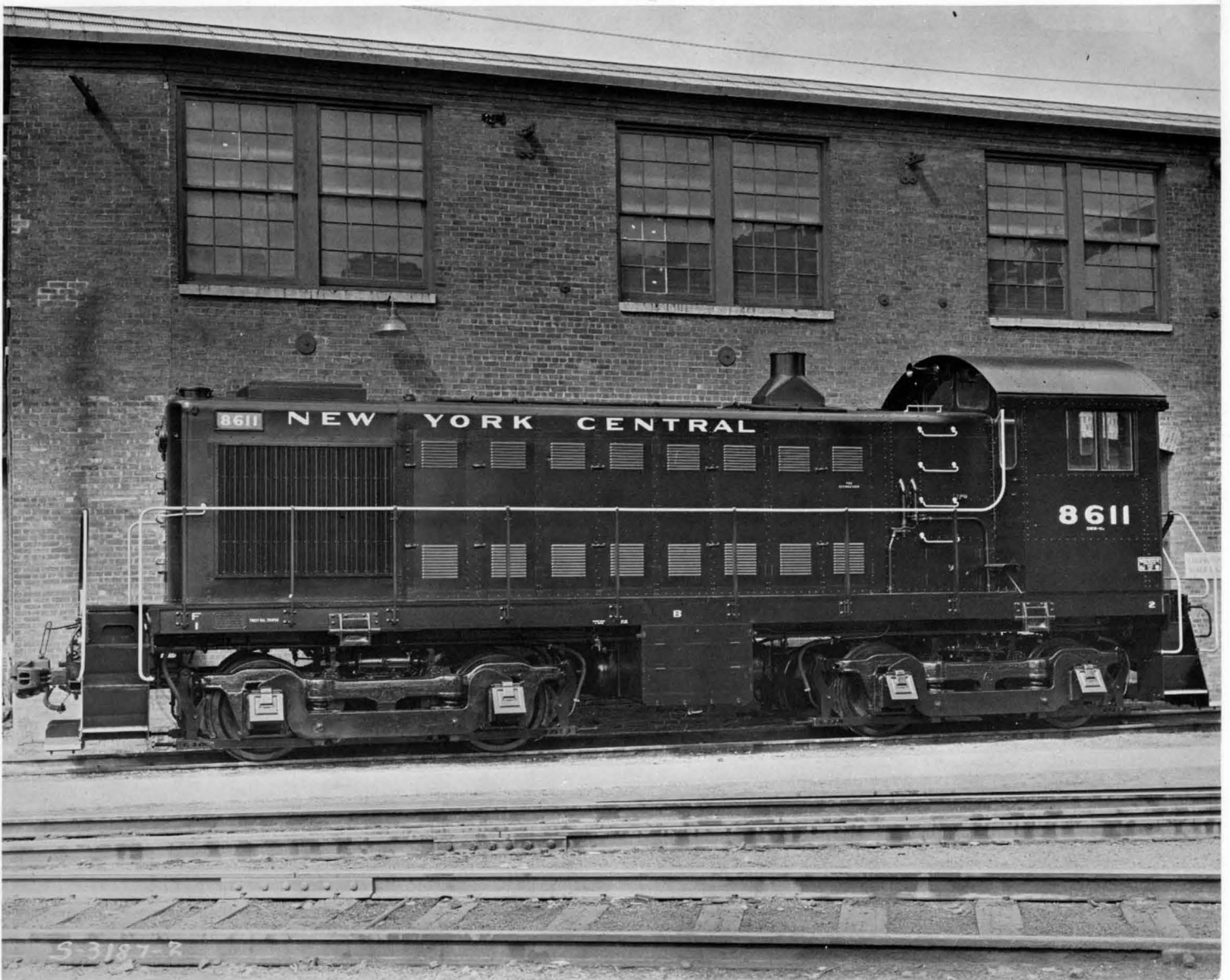
No. 8611, Class DES-11k was a model S-4 switcher built by Alco in March 1952. This 1000 hp. locomotive was renumbered 9683 in May 1966 and was retired in 1967.
