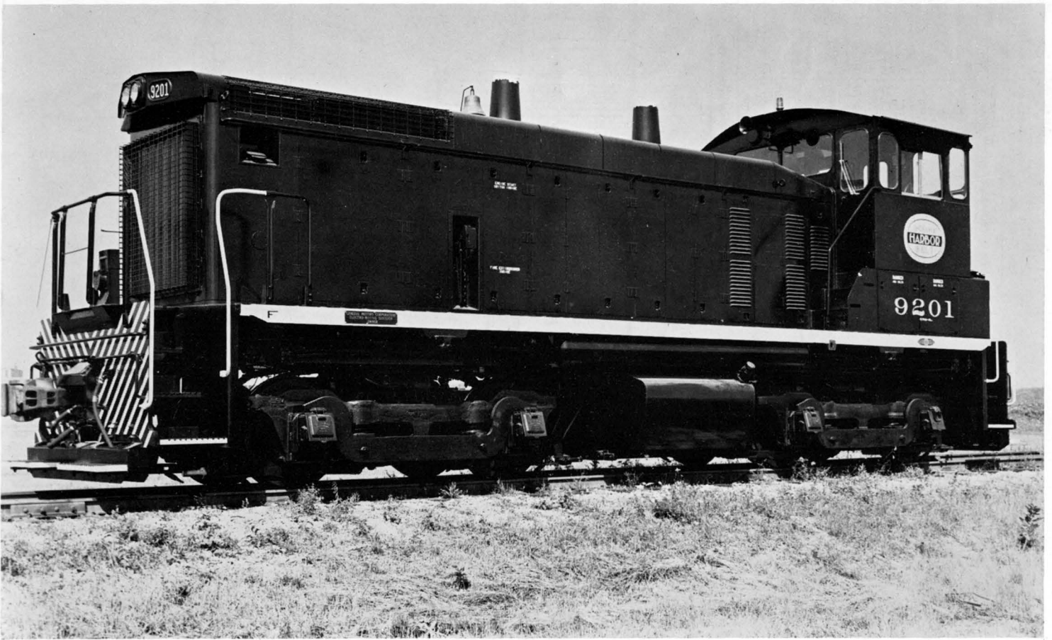
Indiana Harbor Belt No. 9201, Class ES-15m. SW-1500 was built by E. M. D. in July, 1966. N. Y. C. S. classification DES-22 was assigned, but not lettered on locomotive or officially used due to the pending P. C. merger.
