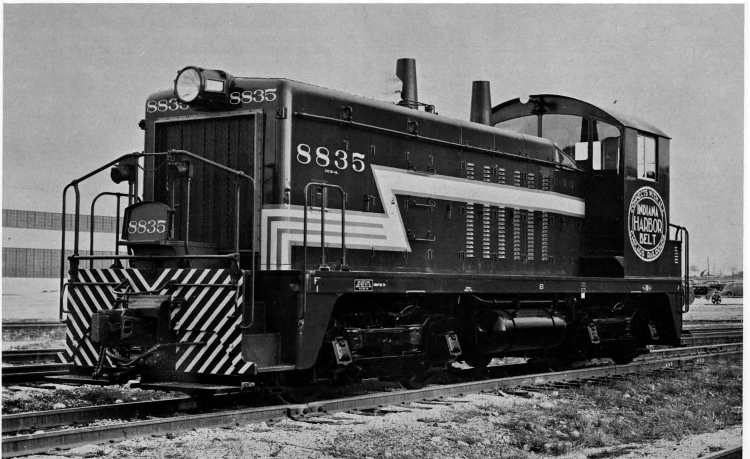
I. H. B. No. 8835, Class DES-16a, model SW-7 switcher was built by E. M. D. in Oct. 1949. Bell has been wrapped up.
