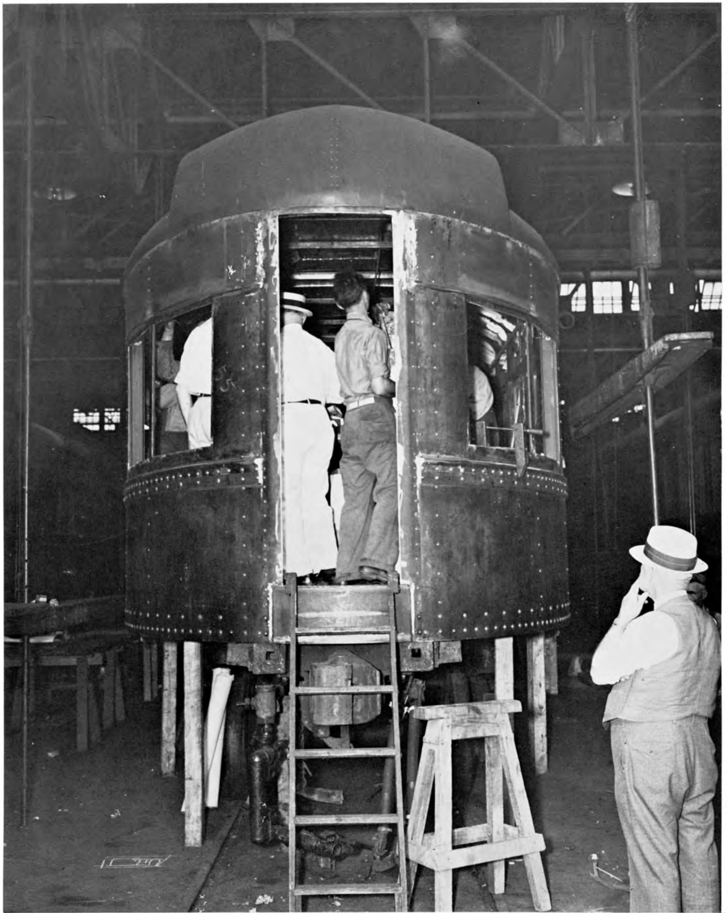
Unusual observation end view of either lounge observation No. 53 or No. 56 as it appeared at the Beech Grove shops in 1940, undergoing its second rebuilding for use on the "Pacemaker."
