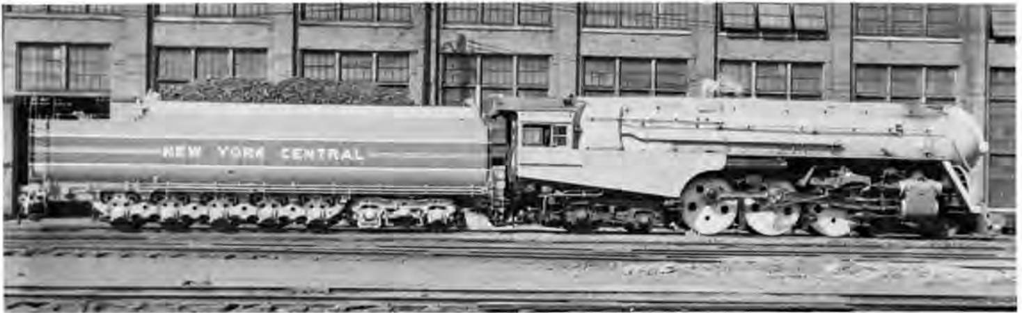
On PT tenders a condensed arrangement of 1941 Empire State Express tender lettering was used, with the 1939 striping, as shown here on a PT-1 tender, as new, at Beech Grove Shop in May 1943. NYC RR photo, collection of Al Stauffer.
