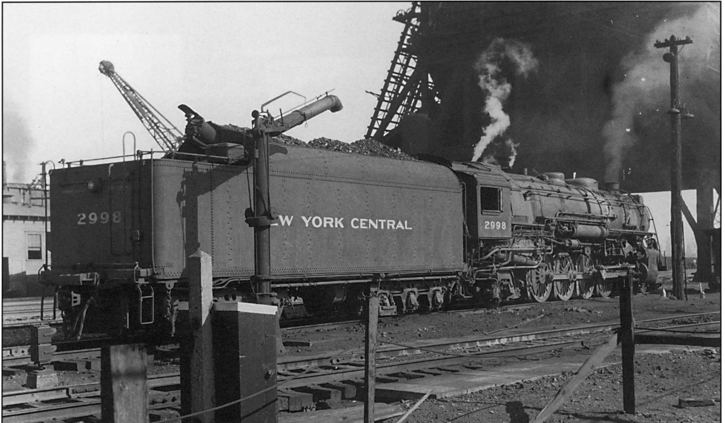
Class L2d (converted) 2998 at Wesleyville, Pa. main line coal dock, October 1948. Engine faces east. Tenders on the 2995 and 2998 were unique, passenger style collars, no overflow control. Note Union Steel Casting Co. Web Spoke driving wheel centers. Photo by H. L. Vail, Jr.
