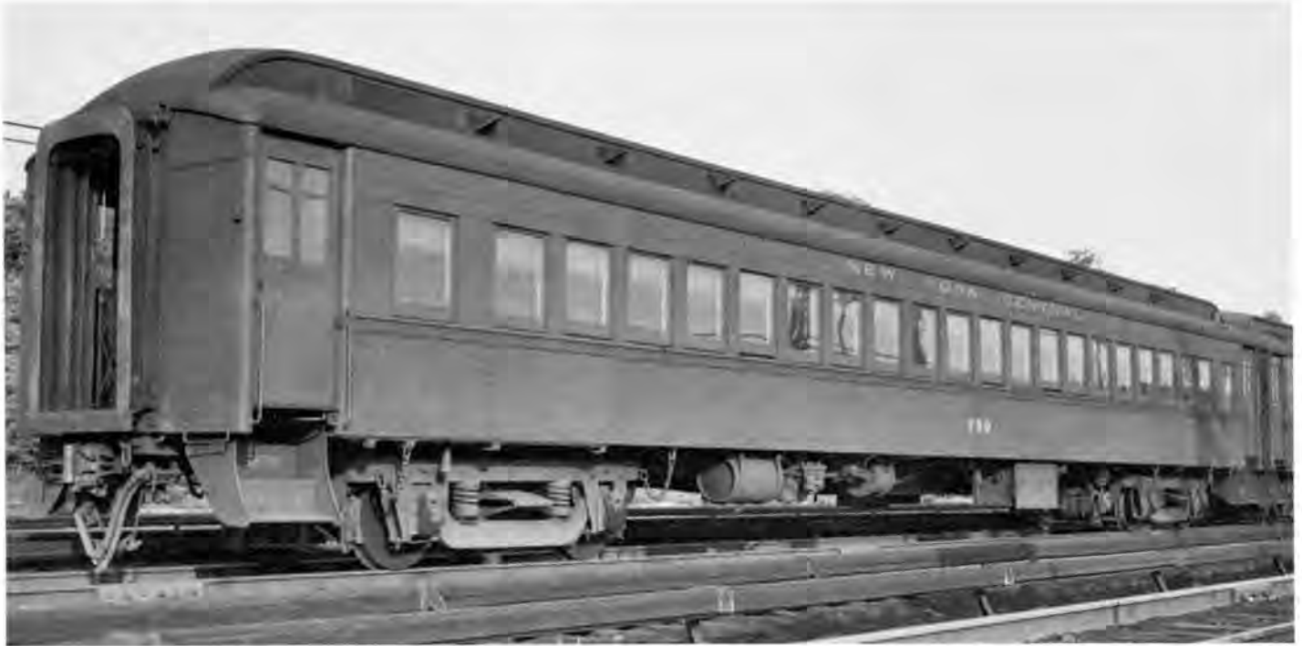
This photo is of unusual interest for two reasons. First, it illustrates the split-plate letterboard which was an as-built detail on a number of 70-foot steel coaches and which required a slightly higher-than-usual placement of the lettering. Most cars had the one-piece letterboard plate illustrated in the other photos. Second, this car was built by Standard Steel Car Company in 1918 as NYC 1152 and had been renumbered to NYC 1783 in 1937. But as part of a limited renumbering program, which covered some of the oldest non-ACed 70-foot steel coaches used in commuter service, this car was renumbered again in the 1940's to 789.
