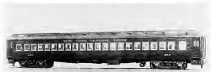
This builder's photograph illustrates as-built lettering for a subsidiary road, in this case the P&LE, and the rare use of brass window sashes instead of the normal wooden sashes. NYCSHS Collection
