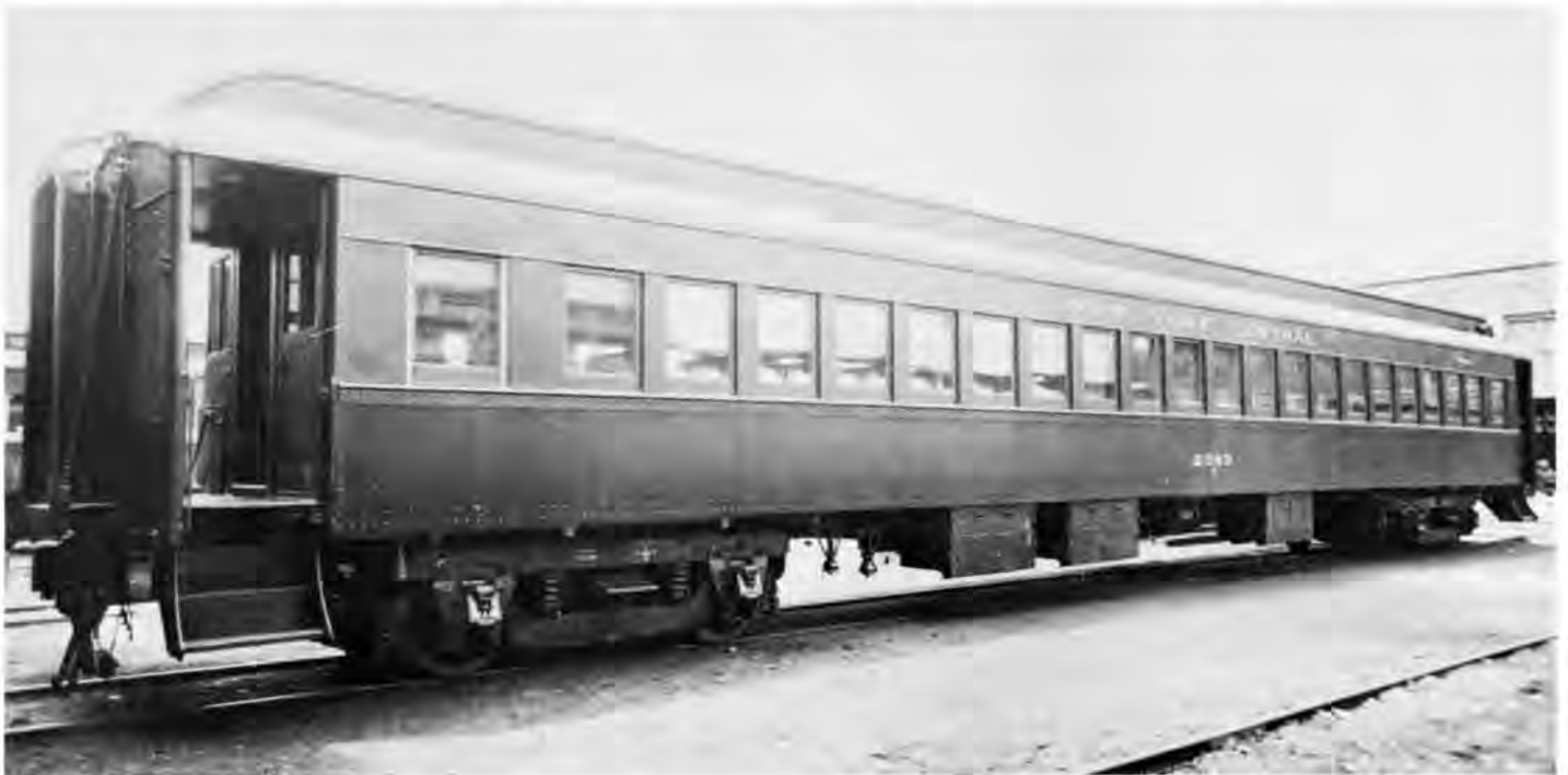
This photo shows one of the earliest cars to be air conditioned as it appeared in 1939. Note that the car is still in pre-1939 serif-style lettering, with a "C" under the road number to indicate air conditioning. The use of one road number per side, as shown here, first appeared in 1934. Note also how the Ward ventilator openings along the side of the clerestory have been sealed over. Cars air conditioned after 1941 looked similar, but had a Garland ventilator installed over the lounges, whereas 2383 and other pre-1941 air conditioned cars retained the original Globe ventilators there. This car was built by Pullman in 1926 as MC 394. NYCSHS Collection
