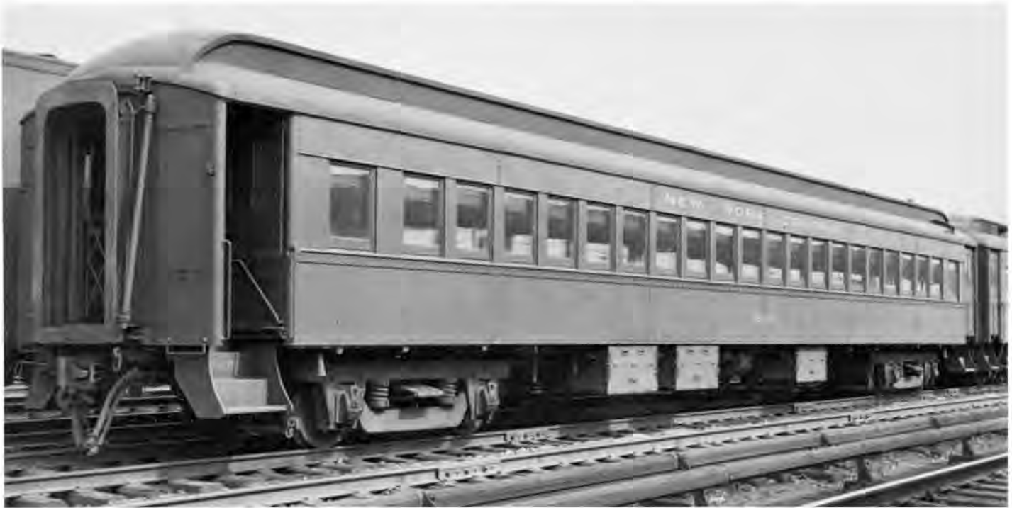
A typical air-conditioned coach with the sans-serif style of lettering which first appeared in 1939. This car was built by Standard Steel Car Company in 1924 as NYC 1049. W. M. Curtis, Edward L. May Collection
