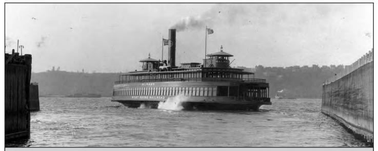
The Albany was the last ferry built for the West Shore Railroad, replacing the sole remaining sidewheel ferry, the *Buffalo*, in 1925. She was different in appearance from the West Shore's other ferries then in service, with pilot houses above the top deck and a different seating arrangement on the lower deck. Here she is at an early date in her career, leaving 42nd Street. NYC Neg. 9161, NYCSHS Collection.
