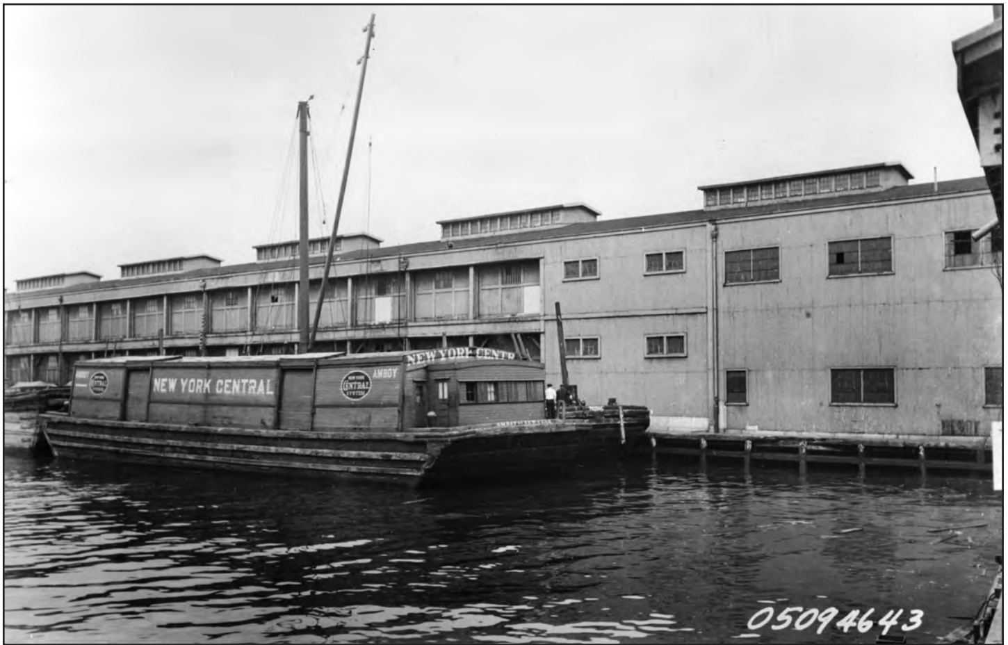
The wooden barge Amboy is tied up at a Manhattan pier, with two crewmen on it looking at the neighboring stick lighter, whose derrick sticks up behind the Amboy . There are some variations in these barges; here the captain's cabin sticks out at the end in a somewhat unusual way. But the size and capacity of the Amboy were very standard: 100' x 30', 250 tons. This image was made for the New York City Department of Docks. "System" in the oval dates the photo later than 1935. T. Flagg Collection.
