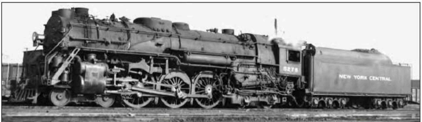
When No. 8 arrived at Syracuse with DPA-2B (Alco PA-1) 4202 "dead on arrival," J-1d 5276 was coupled on ahead. With Jim at the throttle and engineer J. Noe on "the engine next to the train," the doubleheader left Syracuse 30 minutes late and arrived at Albany 20 minutes late. Here's the Elesco coll-type feedwater heater-equipped 5276 in East Buffalo a year later on October 28, 1952. Photo by William Curtis, May Memorial Collection.
