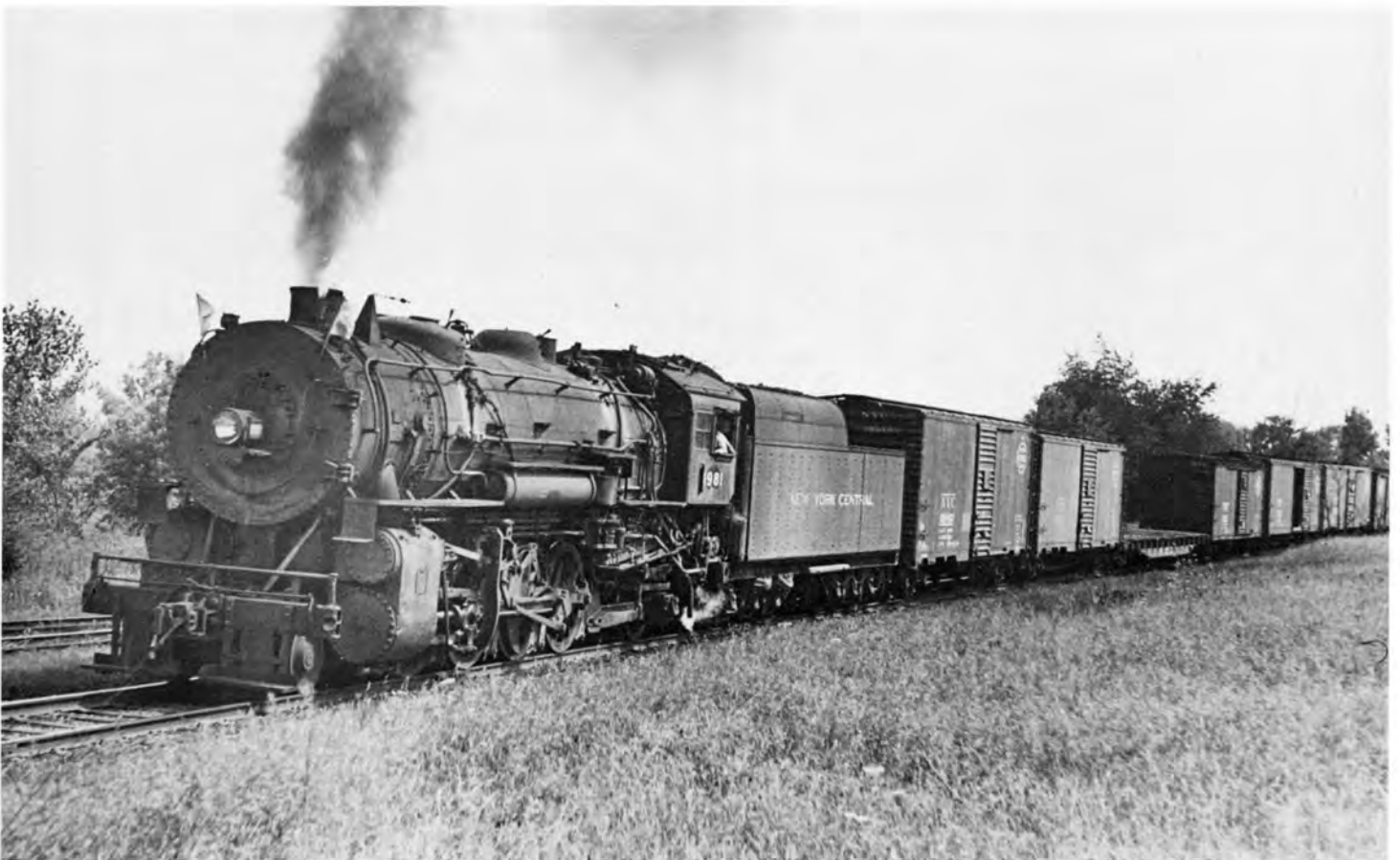
H7e 1981 on southbound freight at Washington, Indiana, 1952. Note pyramid support for radio antenna to rear of stack. Ray Tobey
