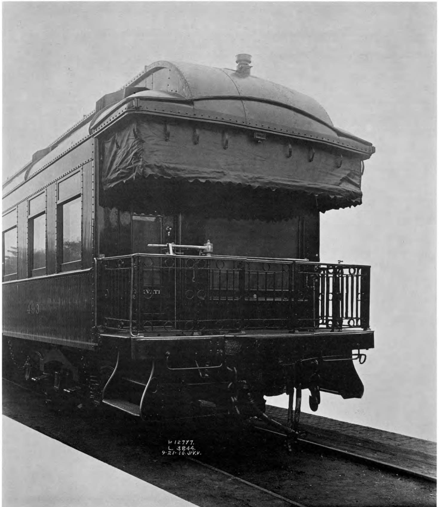
Here is the "business end" of car No. 493, named "Herkimer". This N. Y. C. & H. R. car was originally assigned to President W. C. Brown. For further details see pages 20 and 21. Note offset end door and wide "picture window."
