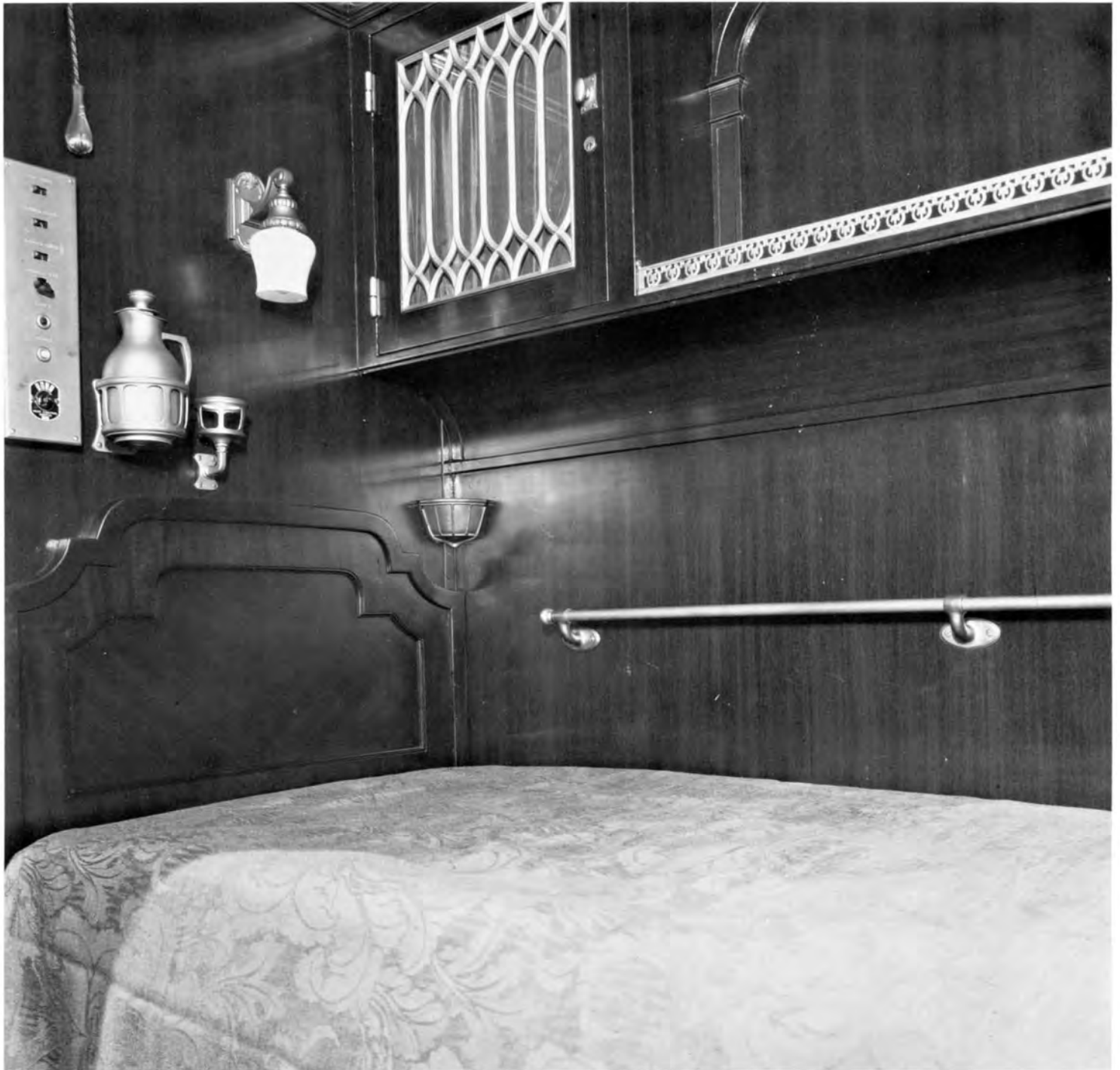
View of main stateroom located next to dining room of business car No. 2. Above the end of the bed are mounted; reading lamp, water pitcher with bracket and drinking glass holder. Control panel at left operated heating controls, ventilation fans and a push button to summon the porter. Heaven help the engineer if the ride was rough enough to require the use of the handrail mounted on the wall.
