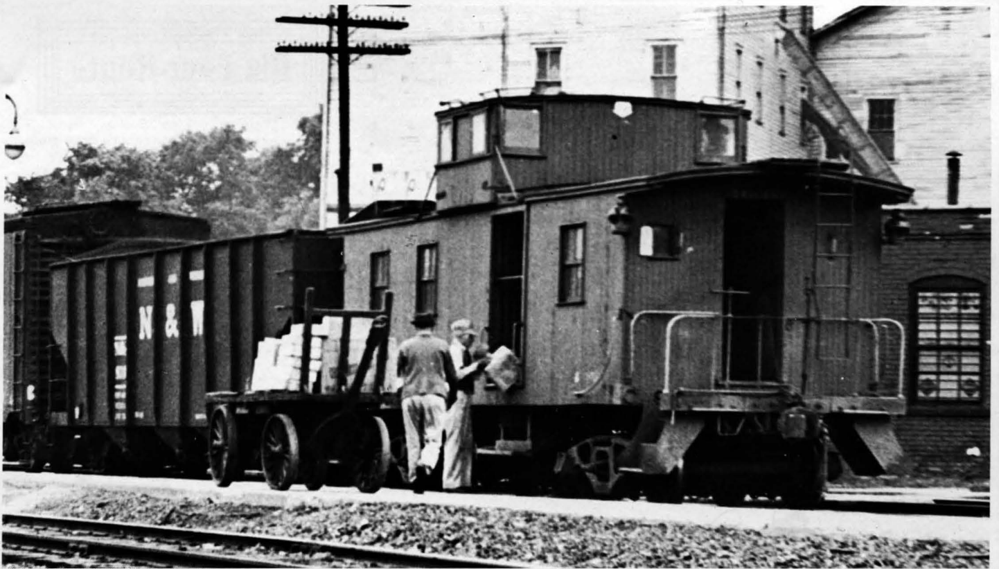
A rare Big Four caboose rebuilding featured a side door, shown here being loaded with l. c. l. freight at Bellefontaine, Ohio in 1948. Train was the T. & O. C. St. Marys Local 554. Si Herring Photo
