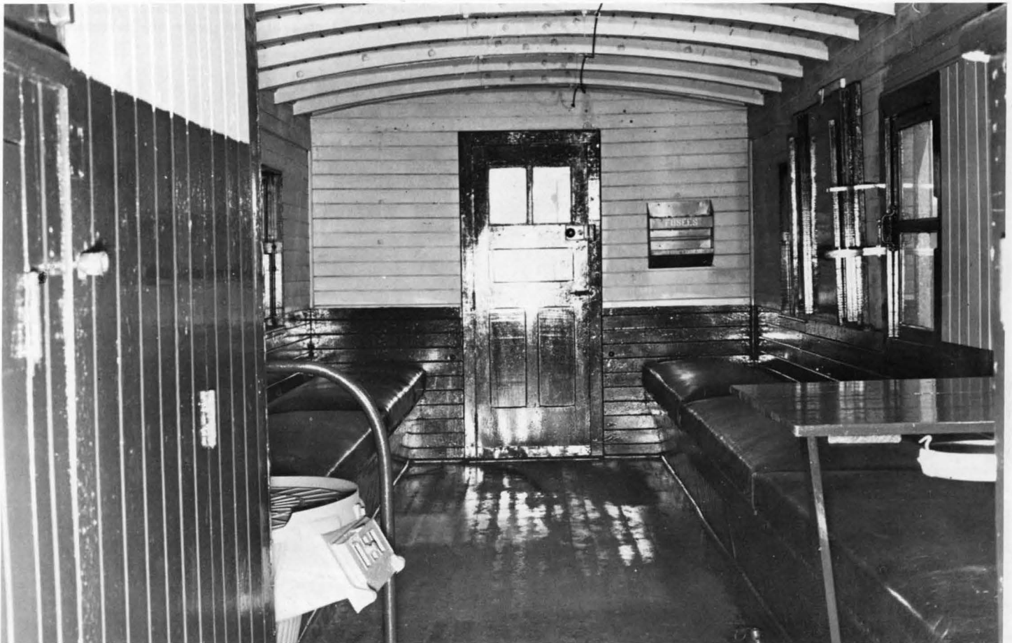
Interior of P. & L. E. Caboose #211. View shows "long end" of caboose from underneath cupola. All N. Y. C. S. "Standard" caboose interiors were similar. Note folding table at right with coal stove and safety guard rail showing at left.
