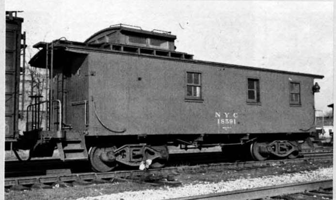
Caboose #18591 at Conneaut, Ohio on November 21, 1946. No N. Y. C. herald appears above the "roman" style lettering but handrails have been painted yellow.
