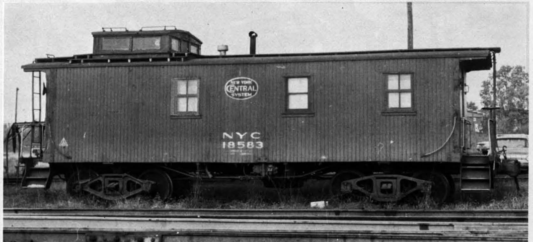
Caboose #18583 shows location of stove smokepipe and vent for the "dry hopper" toilet, whose use could hardly be considered "featherbedding." The truck at the left, under the cupola end of the caboose was the older style "T" section swing motion truck used on N. Y. C. cabooses for many years. The other truck side frame is more modern, having a "U" section casting. Built at Collinwood, Ohio in 1910. Harold K. Vollrath Collection via Carl Prisco
