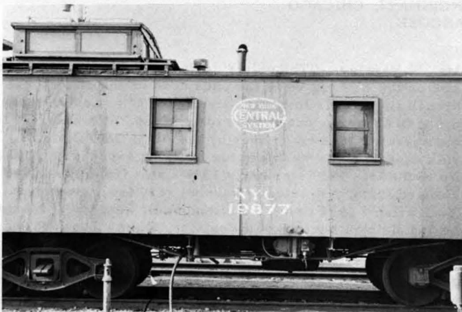
In later years of wood caboose operation, when the tongue and groove siding rotted out, it was covered with plywood sheeting as shown here on #19877 at Niagara Falls, N. Y. at the late date of May 1973. Peter C. Zayau Collection
