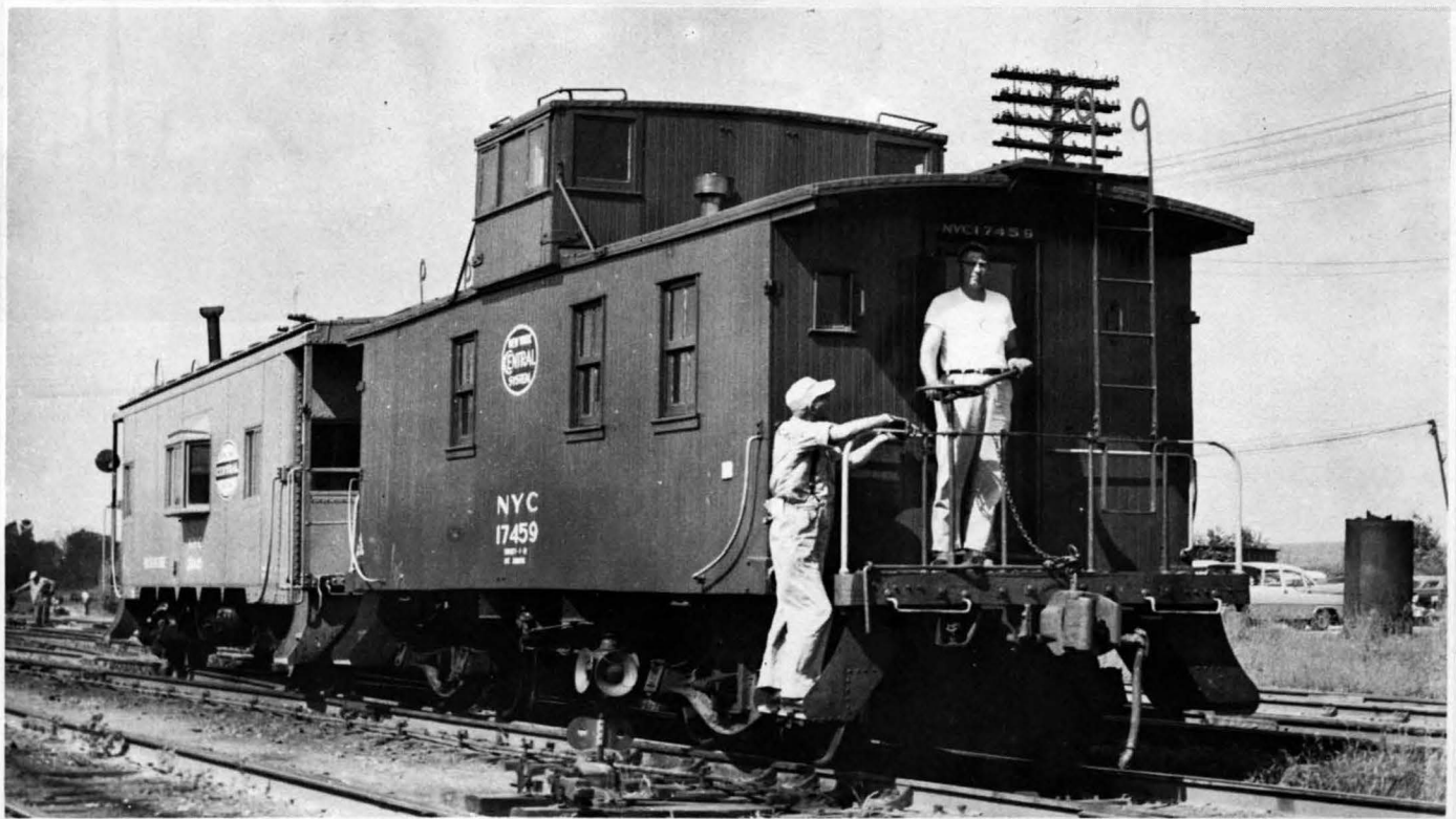
The old and the new. Caboose #17459, freshly painted box car red, has one of its side windows boarded over. Note small window appearing on the left side of the caboose end. No. 17459 has been kicked by a yard engine and is rolling towards the caboose track along with a jade green bay window caboose. Yard conductor J.D. Marker prepares to set the brakes on a warm March day in 1962 at Bellefontaine, Ohio.
