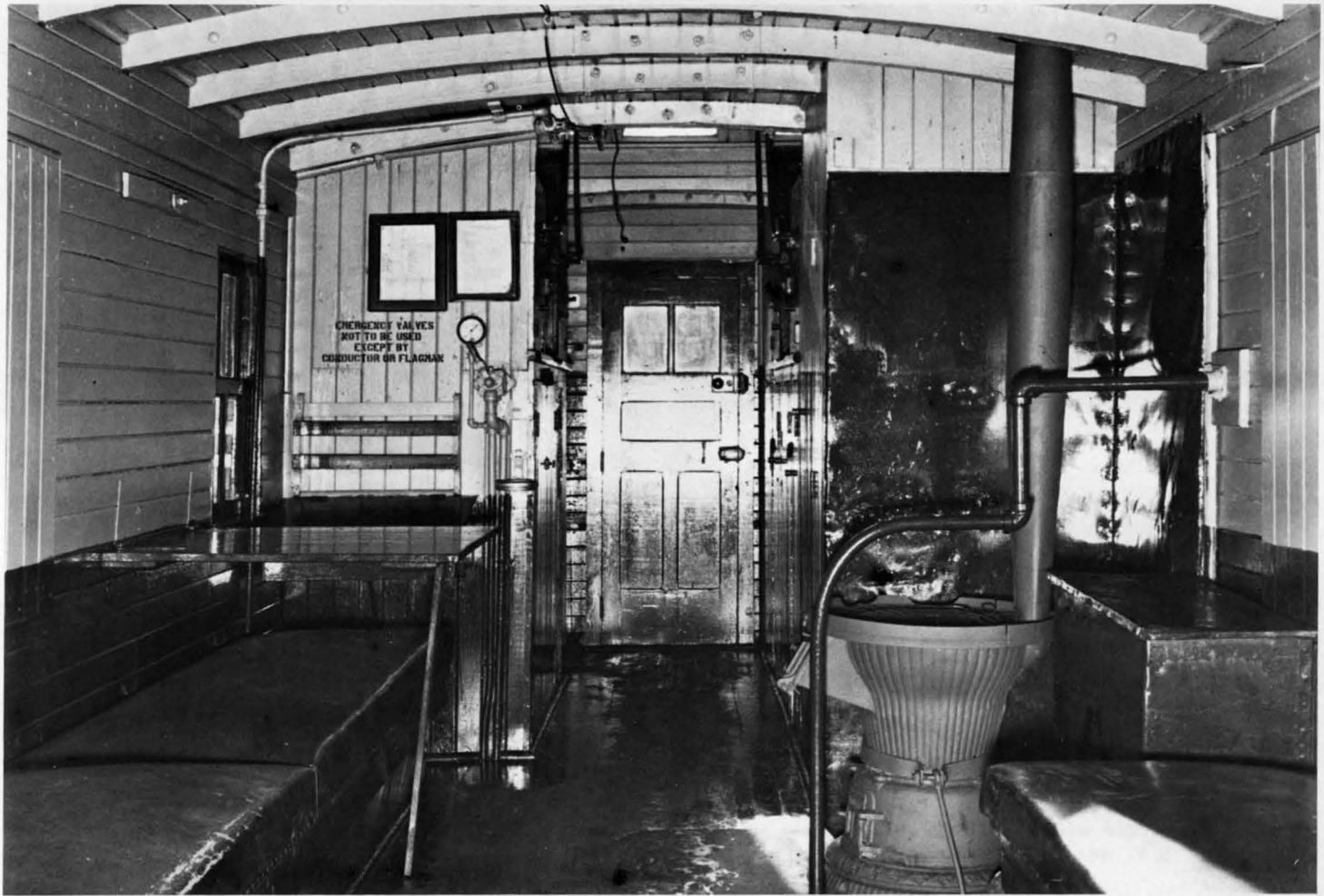
Interior view of P. & L. E. caboose #211 taken from long end of car. Note coal box and metal heat shield behind stove area. Fire was an ever present danger in wood cars with coal stoves. Air brake controls and gauge are mounted on bulkhead of storage locker and cupola seats.
